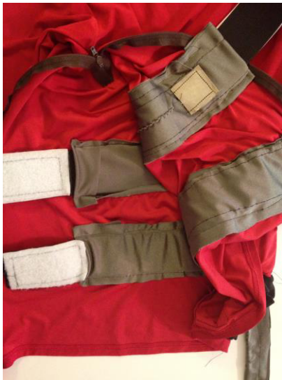
Figure 1: Electrode Integration into Shirt (inside)
