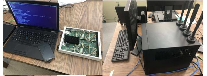
Fig. 4. Experimental Setup: Our testbed consists of Amarisoft Cell and a high performance PC connected to USRPX310.
