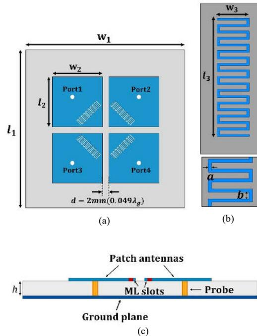
Fig. 4. The configuration of a proposed 2 x 2 slotted antenna array with integrated ML slots: (a) top view, (b) magnified ML slot on patch antenna, and (c) cross-section view. The dimensions of the proposed antenna are:  $w_1 = 40$  mm,  $l_1 = 40$  mm,  $w_2 = 14.75$  mm,  $l_2 = 14.75$  mm,  $w_3 = 2.05$  mm,  $l_3 = 8.25$  mm,  $a = 0.15$  mm, and  $b = 0.3$  mm.
