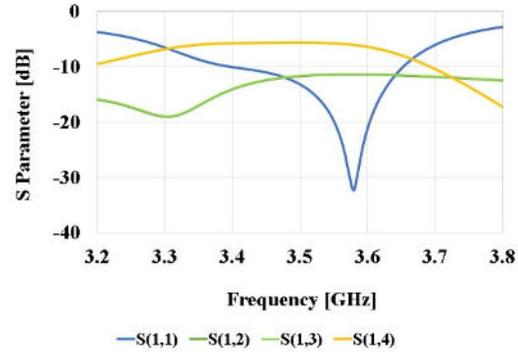
Fig. 3. Simulated return loss (S11) and mutual coupling factors (S12, S13, S14) of the 2 x 2 array antenna with a distance of 2 mm between patches.
