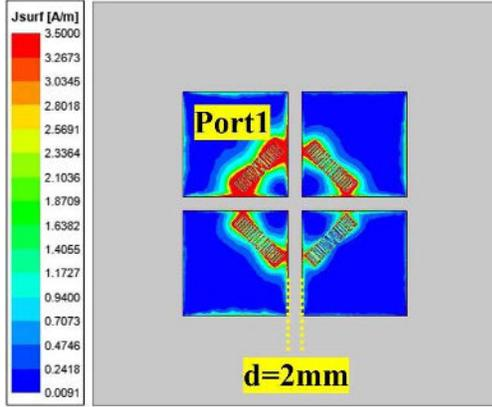
Fig. 5. Simulated current distribution of the proposed 2 x 2 patch arrays ML loading and pitch is 2 mm at 3.5 GHz.
