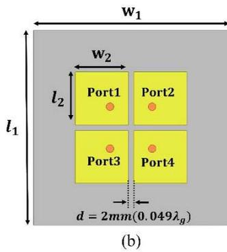
Fig. 1. Configuration of a 2 x 2 patch array antenna: (a) 3-D view. (b) Top view. The geometrical parameters are:  $w_1 = 60$  mm,  $l_1 = 60$  mm,  $w_2 = 19.4$  mm,  $l_2 = 19.4$  mm, and  $d = 2$  mm.
