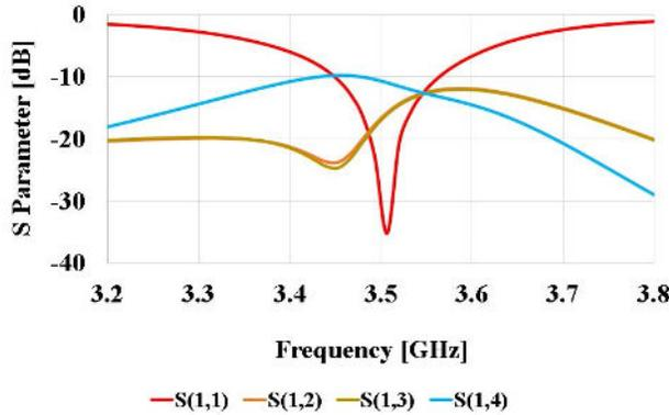
Fig. 6. Simulated return loss and insertion loss of the proposed 2 x 2 patch arrays ML loading and pitch is 2 mm at 3.5 GHz.
