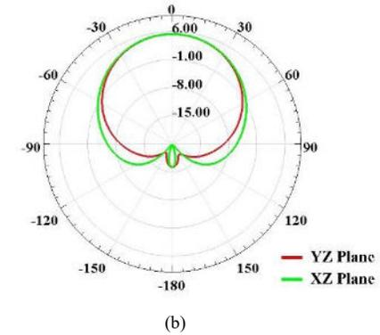
Fig. 7. Simulated radiation pattern of the proposed 2 x 2 patch array antenna. (a) Without ML slots (b) With ML slots
