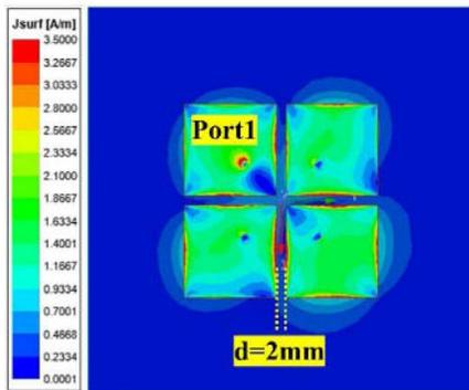
Fig. 2. Current distribution of the 2 x 2 array antenna with a distance of 2 mm.
