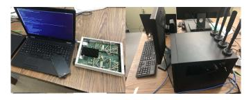
Fig. 4. Experimental Setup: Our testbed consists of Amarisoft Cell and a high performance PC connected to USRPX310.
