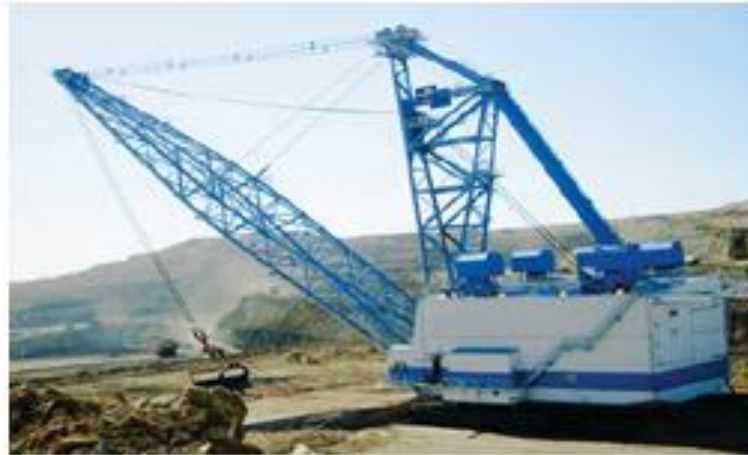
Figure 5-1. 24MW AC-drive dragline in an open-pit mine, 89.
