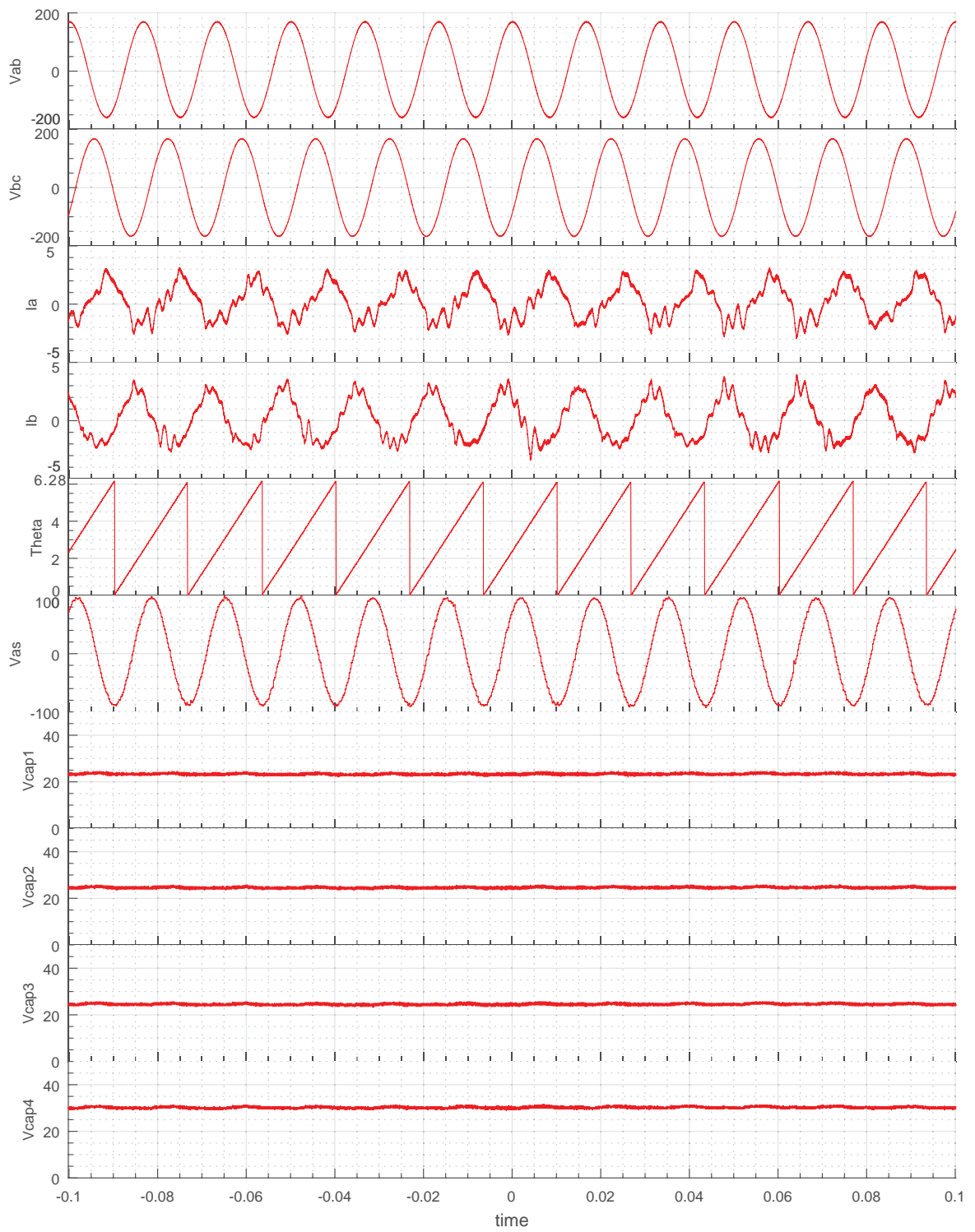
Figure 6.52: CHB in Normal Operation (PLL Output is Shown)
