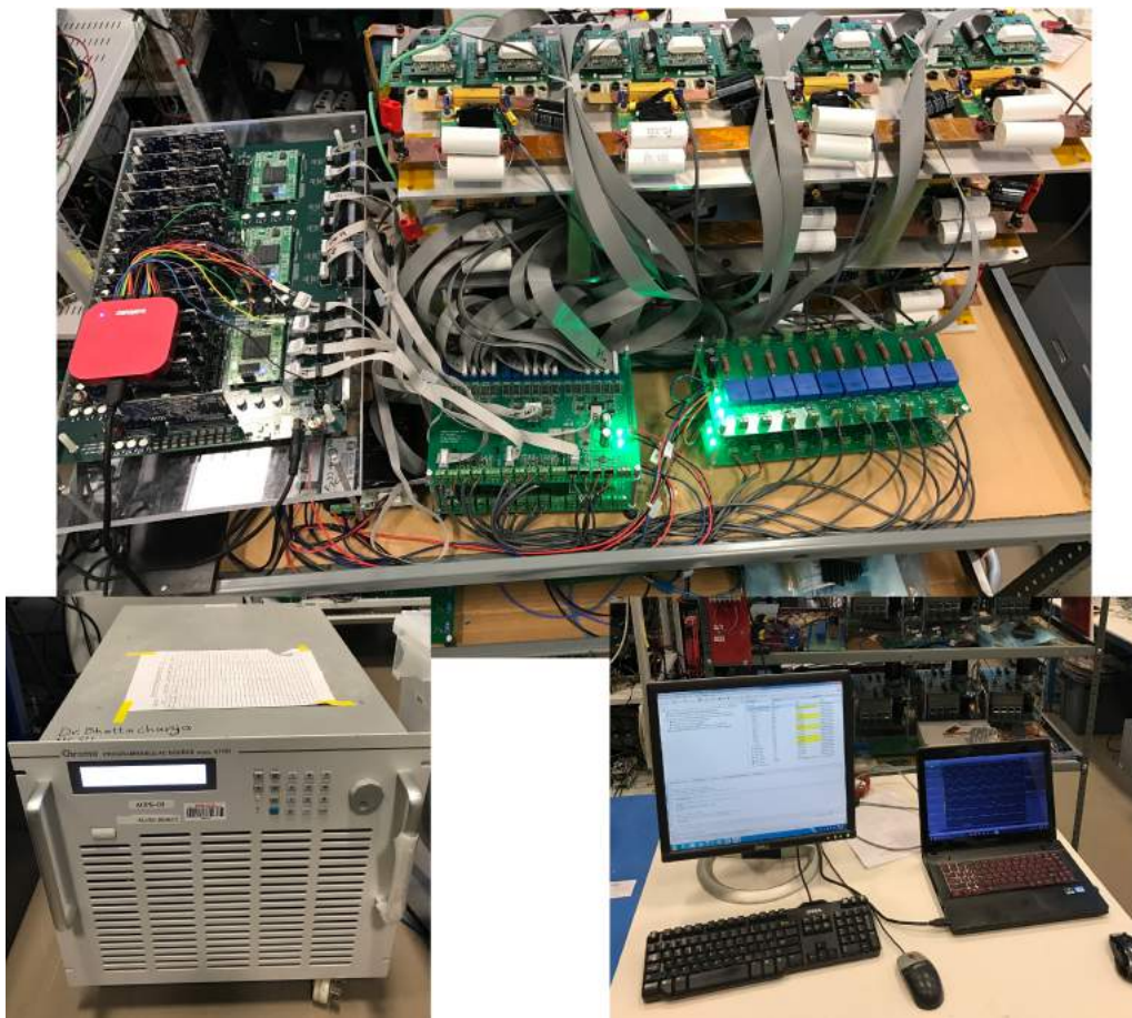
Figure 6.46: Experimental Setup of Cascaded H-bridge Converter (CHB) in Connection with Fault-tolerant Controller
