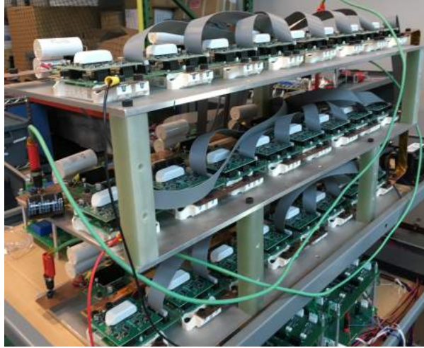
Figure 6.47: Side View of Cascaded H-bridge Converter (CHB)
