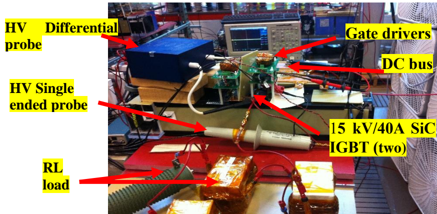
Fig. 5-15: The experimental circuit DC-AC half bridge ZVS converter
