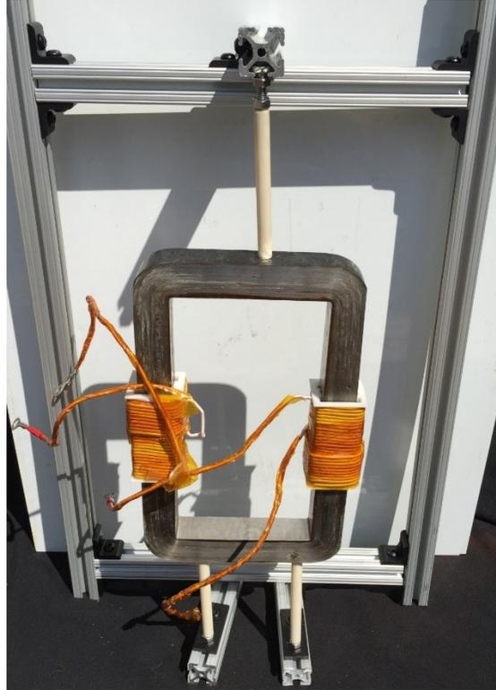
*Figure 3.27: High Temperature Core Harness Prototype.*
