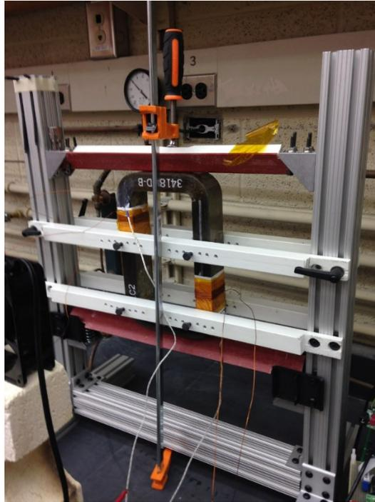
*Figure 3.18: Magnetic Core Testbed Harness.*
