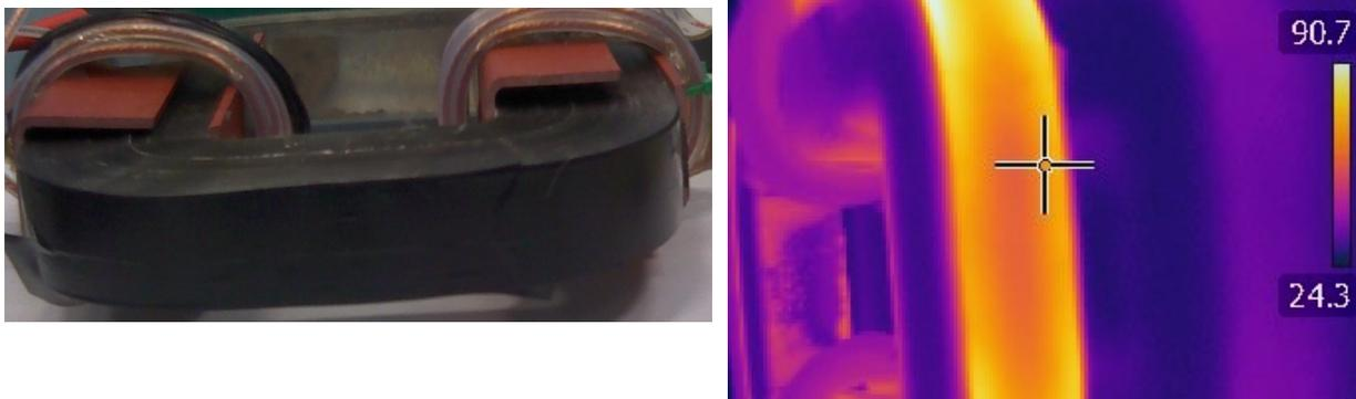
*Figure 4.32: 10 kW DAB Transformer Case Study, Unshielded Top View. Photograph (Left) and Leakage Test Thermal Profile (Right).*
