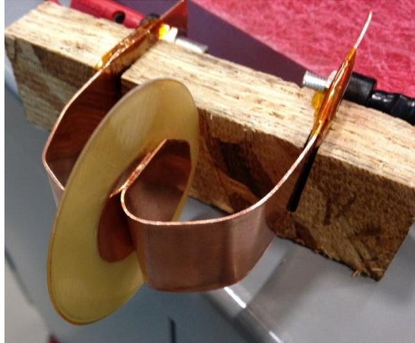
Figure 3.47: *Prototype Dielectric Testing Harness.*
