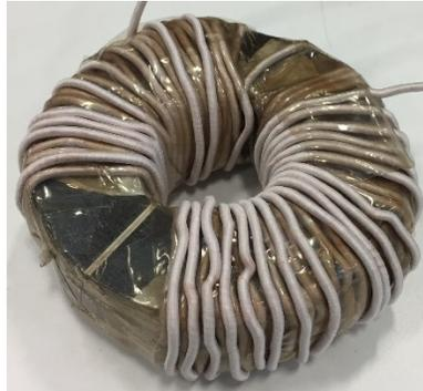
Figure 6.57: Auxiliary Inductor for 10 kW Concentric Transformer.
