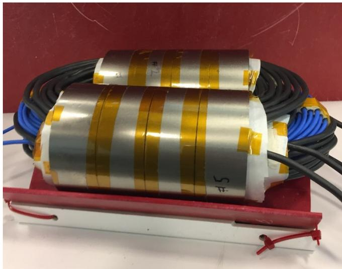
Figure 6.65: Prototype 10 kW Three Port Triaxial Transformer.
