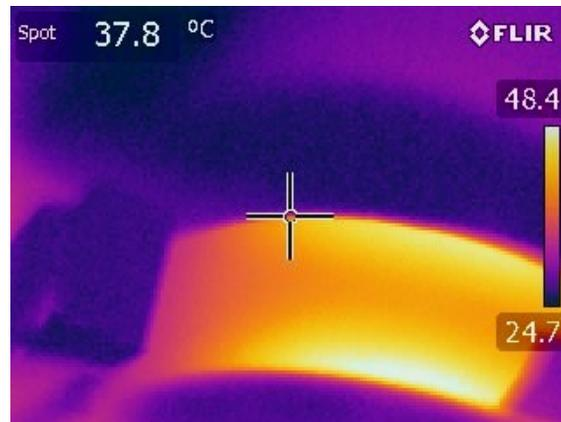
*Figure 4.36: Bar Shield Leakage Top View Thermal Profile.
