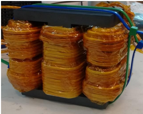
Figure 8.14. Three Port High Frequency Transformer.
