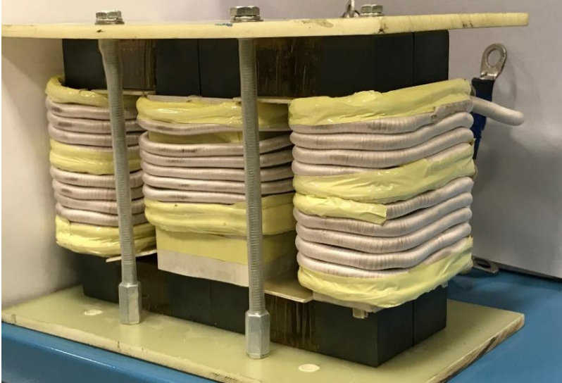
Figure 6.22. 50kW Ferrite Core Transformer Prototype.
