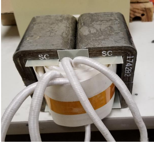
Figure 7.12. Three Port Transformer in Open Frame.
