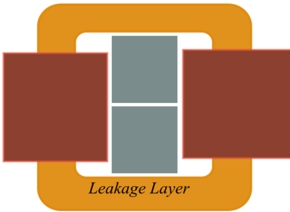
Figure 7.33. Leakage Inside Window.
