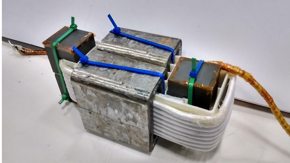
Figure 7.61. Laboratory Prototype of Integrated Transformer Type 2.
