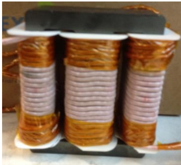
Figure 3.15. Designed Transformer Prototype.
