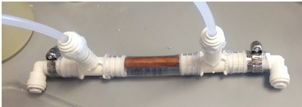
Figure 5-4 Heat rejection section
