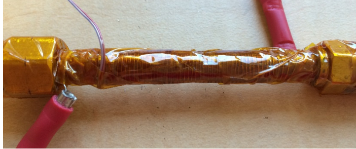
Figure 5-3 Heat source section
