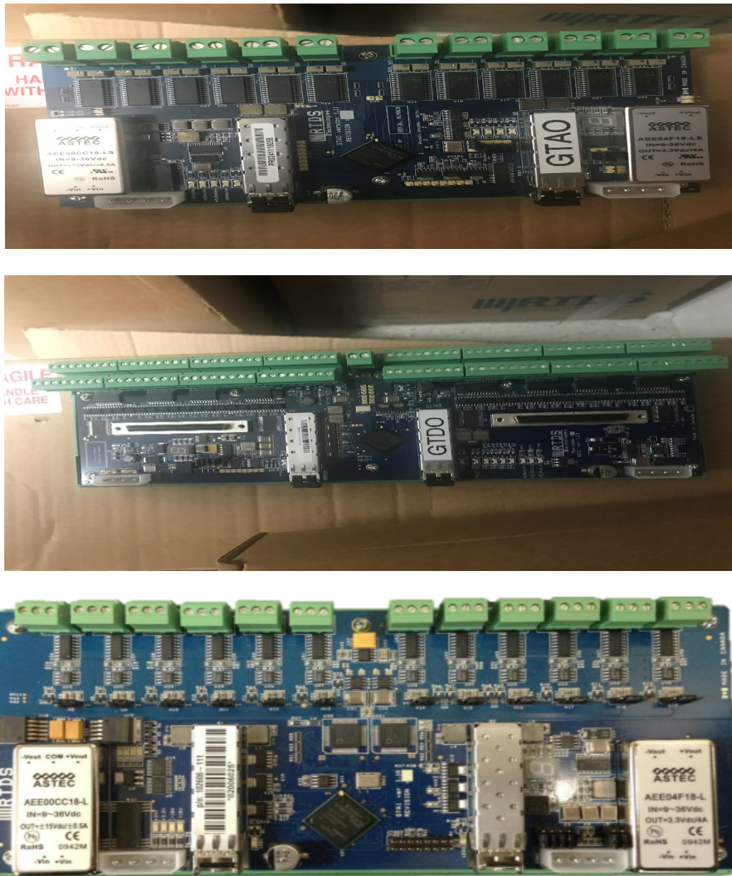
Figure 6-4: GTA0, GTDO and GTAI Cards
