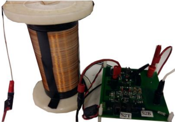
Figure 6.12 Double pulse test setup for the dynamic characterization.
