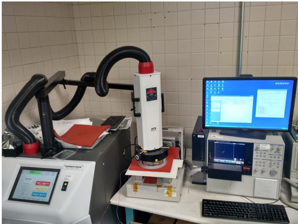
Figure 2.2: Static Characterization Setup with Thermostream
