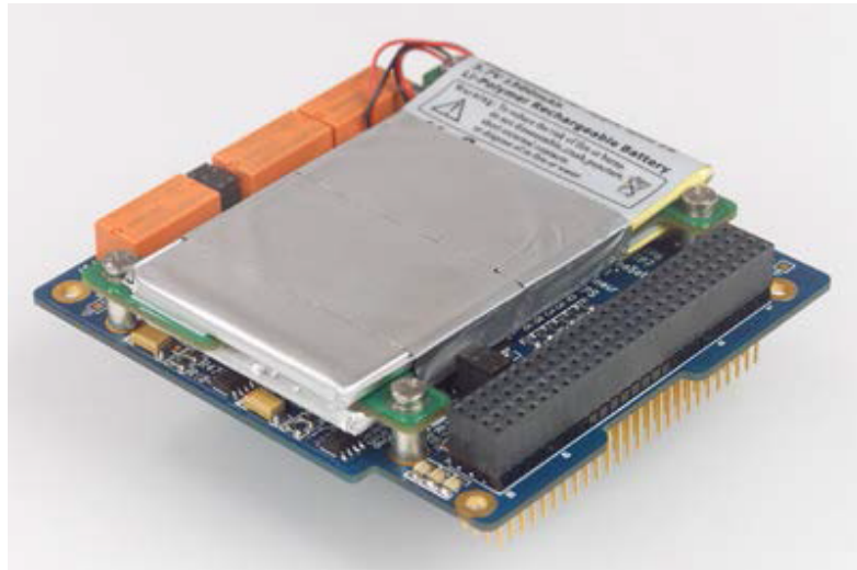
Figure 3.2: CUBESAT KIT EPS
