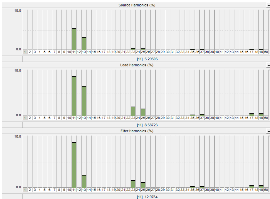
Figure 3.22: Harmonic magnitude plot of the currents in Figure 3.21
