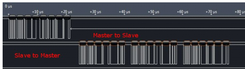
Figure 4.10: CSMA Data Transfer from Slave Controllers to Master Controller
