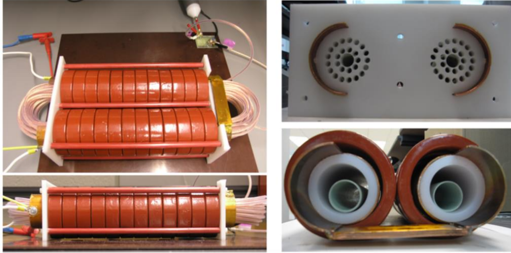
Figure 3.6: Prototype of MV-MF coaxial winding transformer
