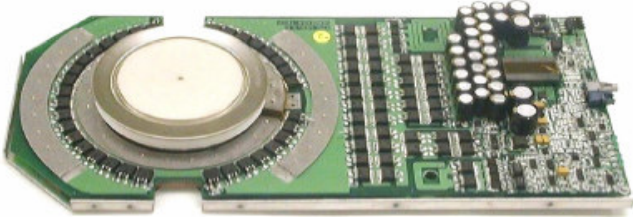
Figure 1-4. The 4.5kV 4.0kA Generation III ETO
