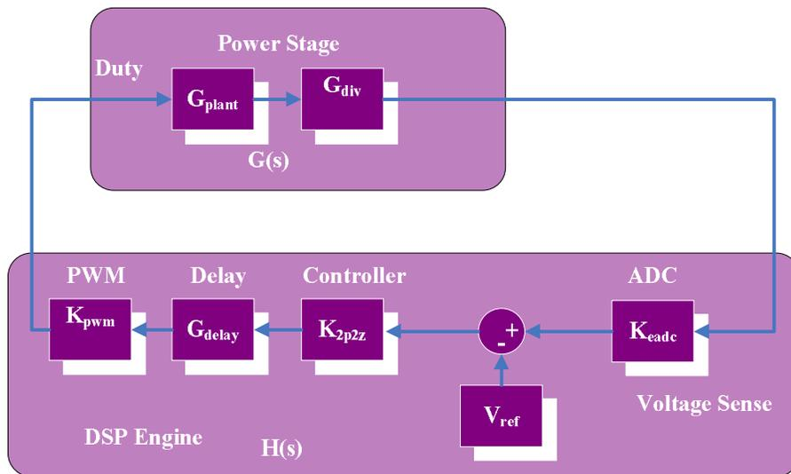
**Figure 52 Digital Closed Loop control elements**
