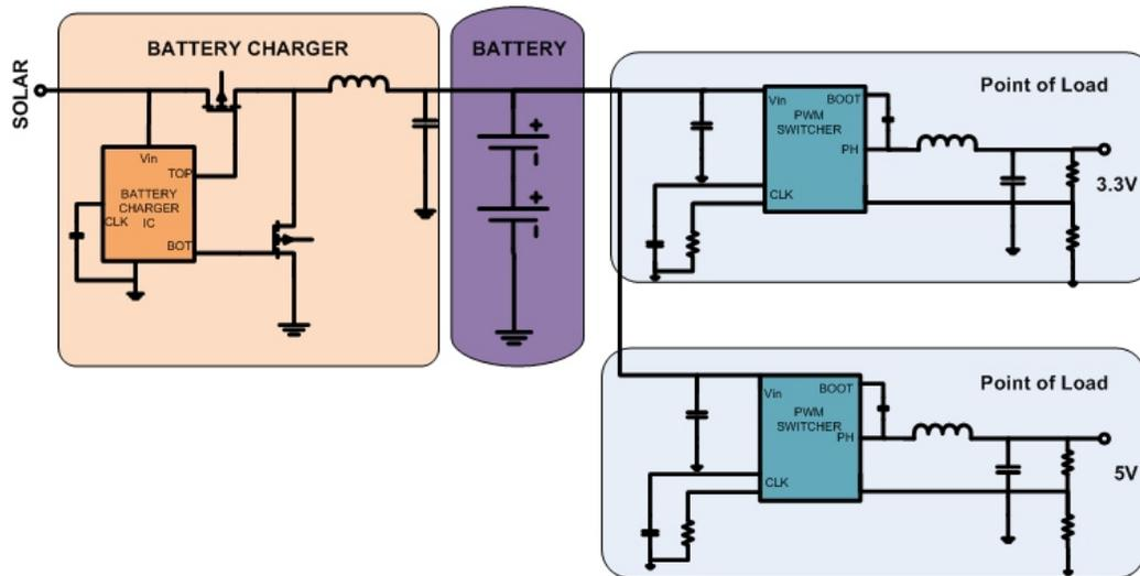
Figure 4 EPS Module for cubesat, block diagram.
