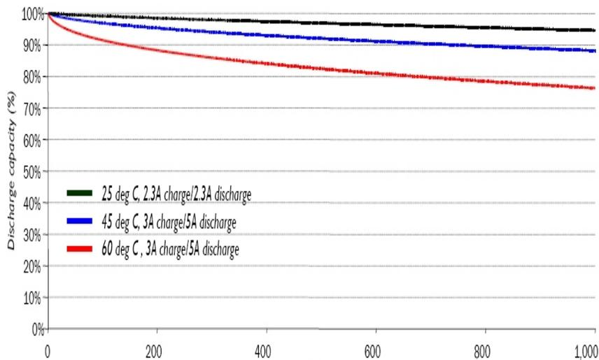
**Figure 34 Cycle Life performance, 100% DOD, various temperatures**
