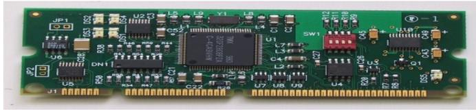
**Figure 50 Central controller control card used for the FBCM and FDPOL**
