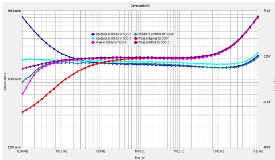
**Figure 42 Galvanostatic EIS measurement Bode plot for Li-ion battery for**
