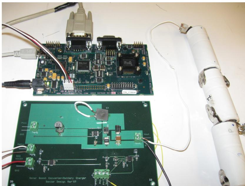
Figure 64 Non-Synchronous Boost Based Battery Charger
