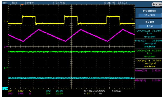
Figure 68 Voltage Mode Boost Converter  $V_{in}=14V$   $V_{out}=28V$   $I_{out}=2A$
