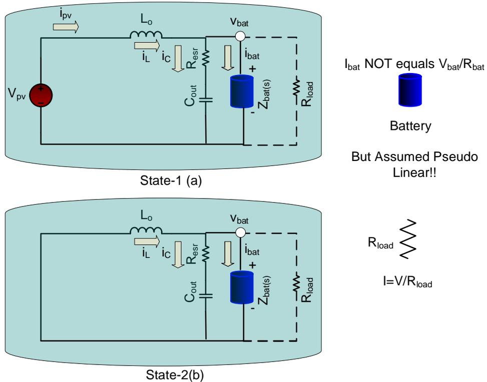
**Figure 15 Linear equivalent circuit for each state of the converter in CCM**
