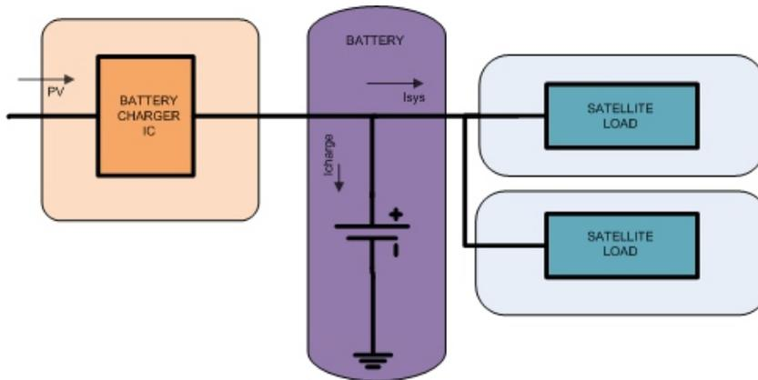
**Figure 5 Direct Connection Topology**
