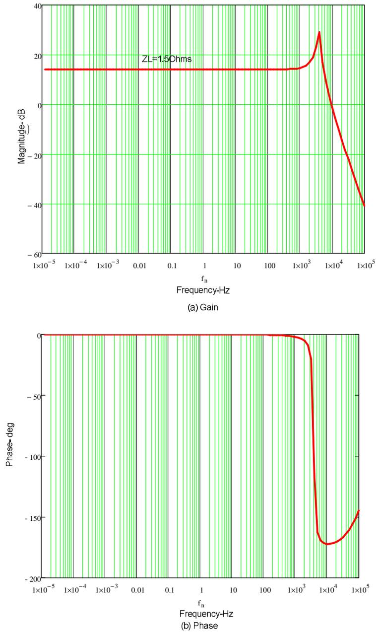
Figure 18 Control-to-Output Voltage Transfer Function (a) Gain and (b) phase plots
