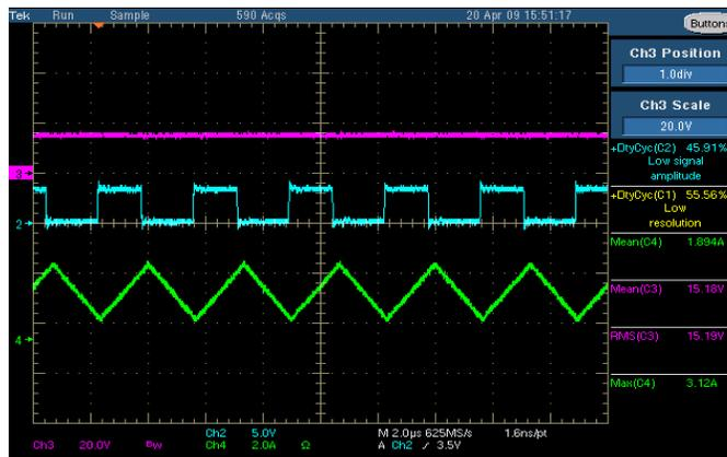
Figure 70 MPPT/Current Mode Boost Converter  $V_{pv}=16V$ ,  $I_{pv}=1.8A$
