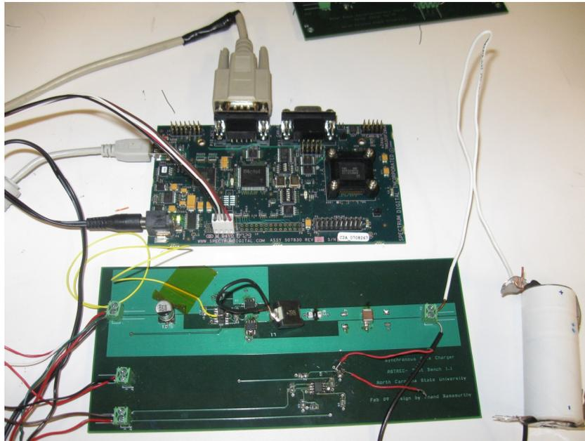
Figure 63 Synchronous Buck Based Battery Charger
