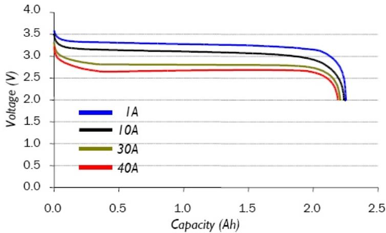
**Figure 32 Discharge Characteristics of ANR26650 Li-ion battery from A123**
