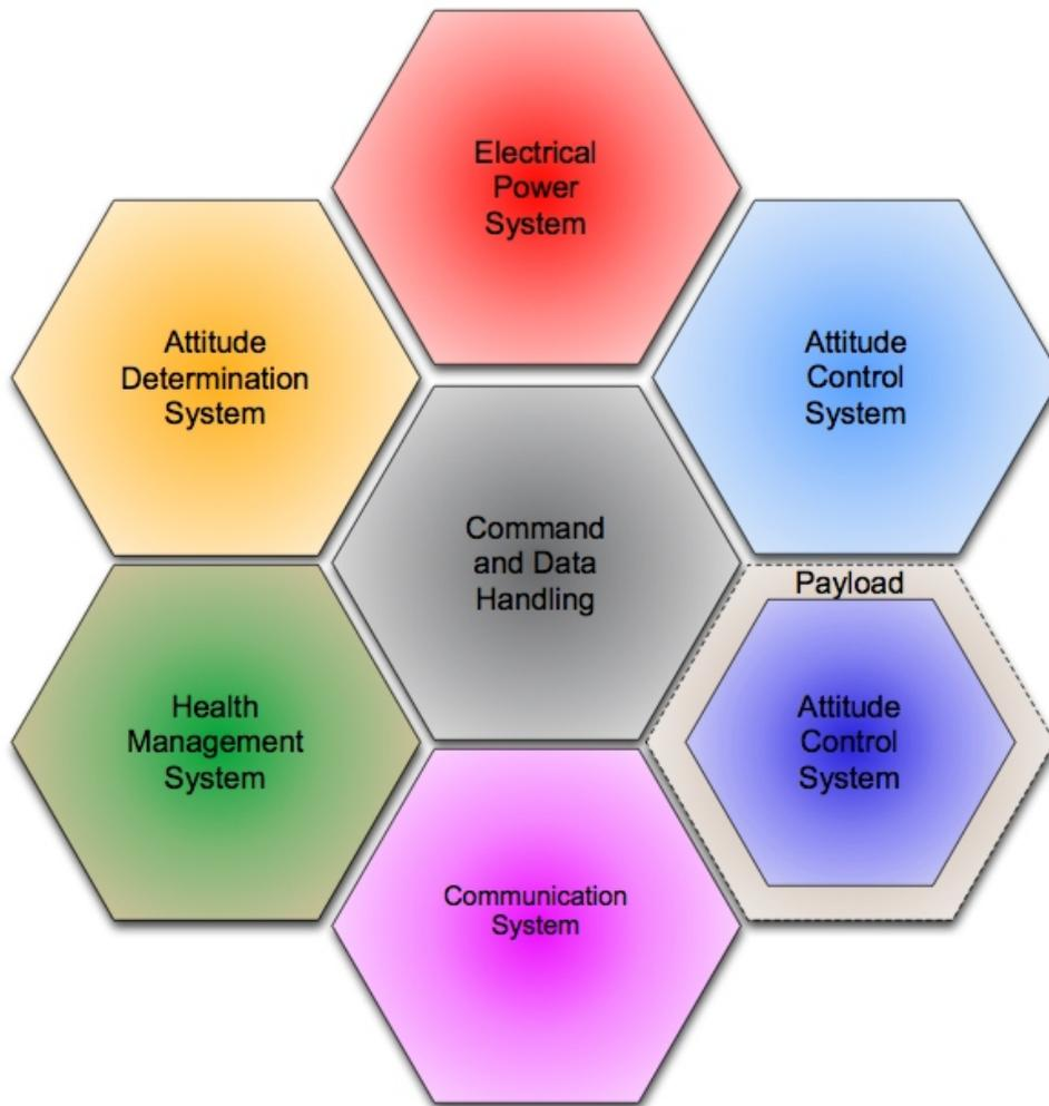
**Figure 1 Small Satellite Subsystems**
