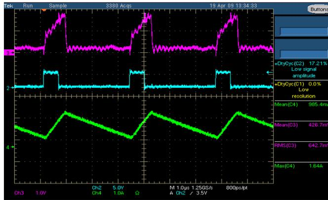
Figure 69 Current Mode Boost Converter  $I_{out}=2A$
