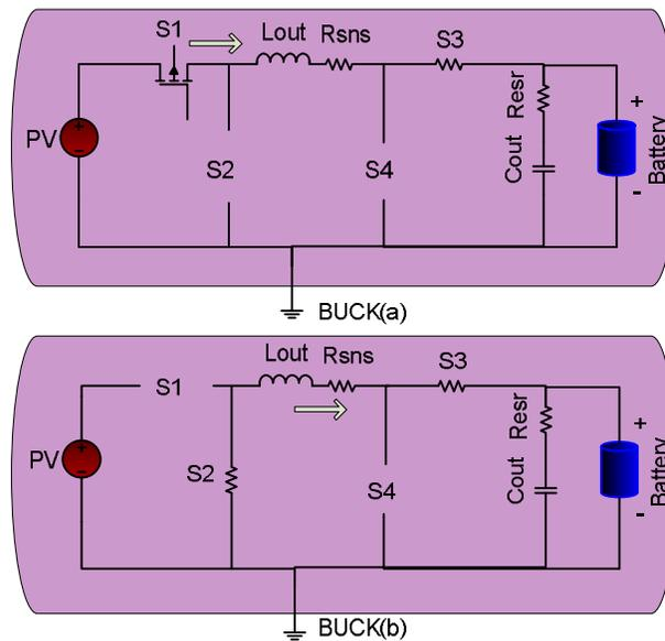
Figure 12 Buck Inductor charge and (b) Inductor discharge
