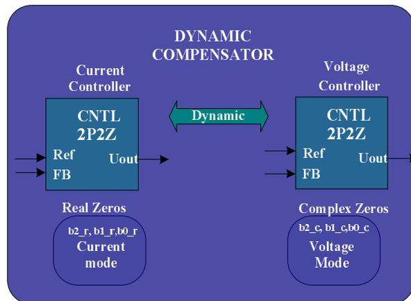
Figure 55 Dynamic compensator model for battery charging algorithm.
