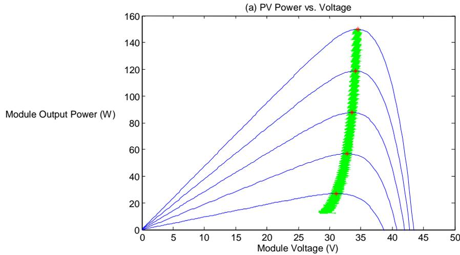
Figure 44 Maximum Power Point Tracking with variable irradiance level
