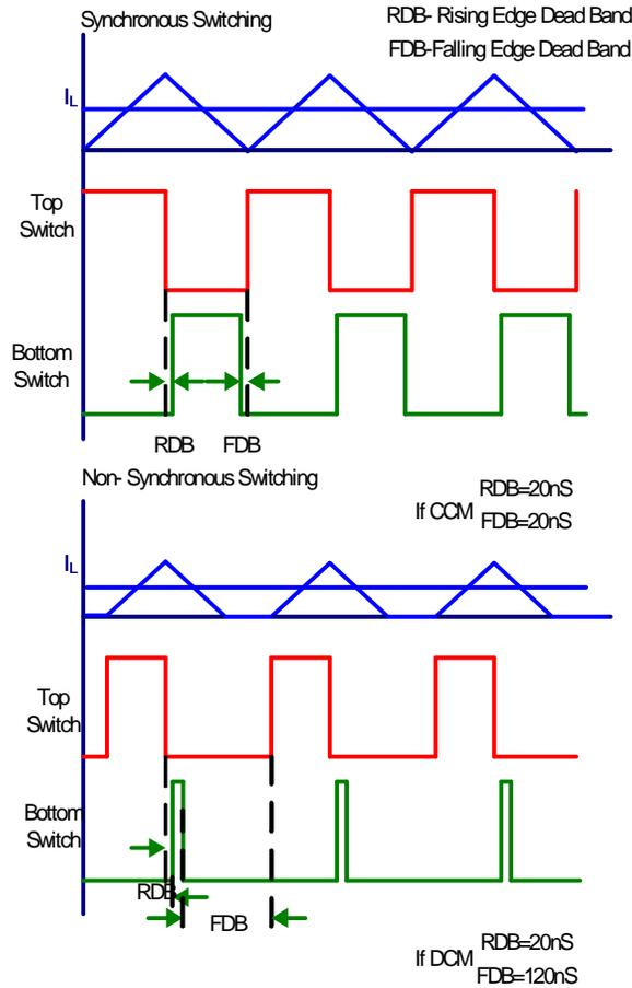
**Figure 58 Synchronous Switching and Non-Synchronous switching**
