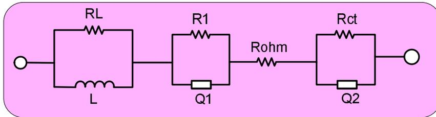
Figure 41 the equivalent circuit model used for NLLS fitting curve
