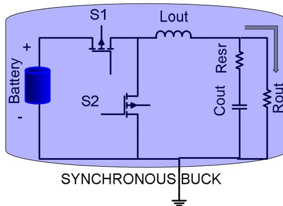
Figure 14 Synchronous buck stage used for FDPOL modules
