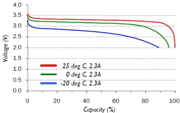
**Figure 33 Low temperature discharge performance**
