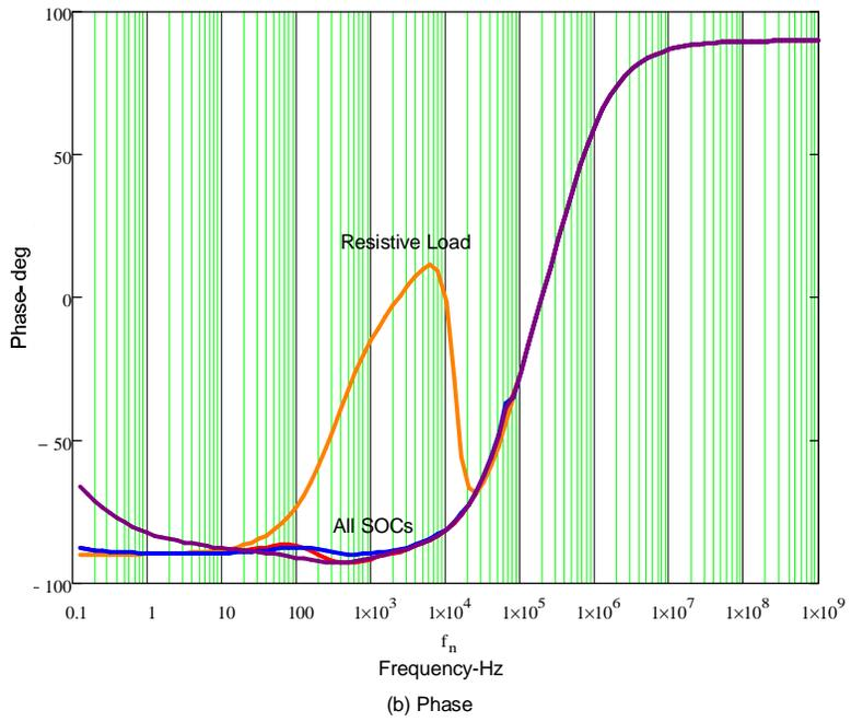
Figure 23 Input Current Loop (a) Gain and (b) phase for All SOCs and resistive load
