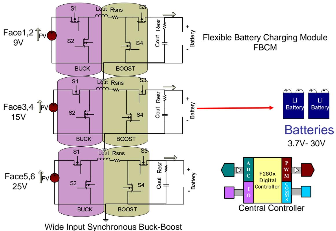
Figure 8 Flexible Battery Charger Module (FBCM) Structure
