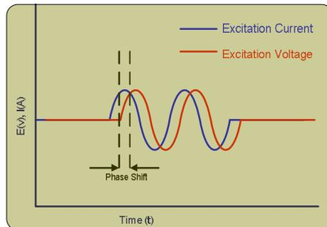
**Figure 35 Sinusoidal Current Response in a Linear System**
