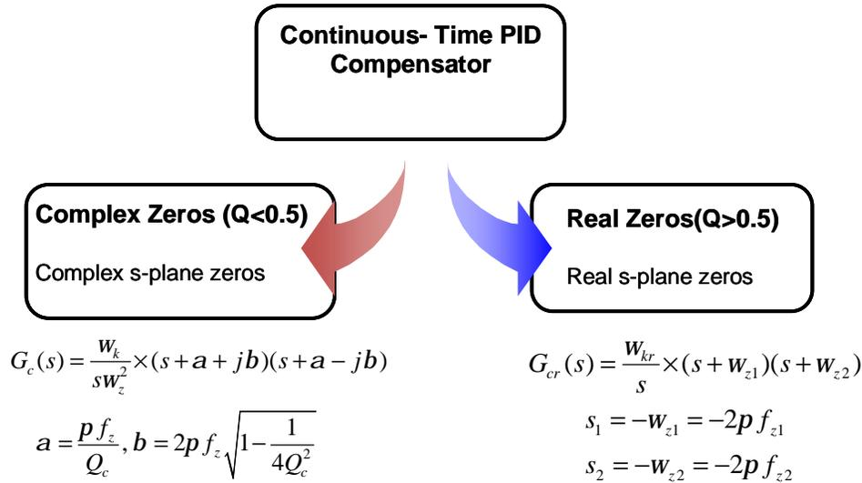
**Figure 61 shows the two types of continuous time compensators which are real and complex**
