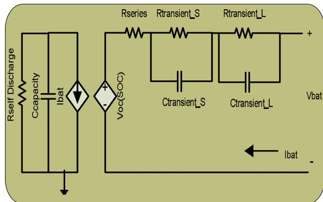
**Figure 37 Run time based Model**
