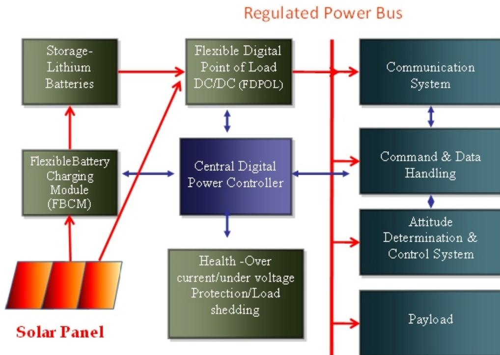
**Figure 7 Centralized Power System Architecture for small satellites**
