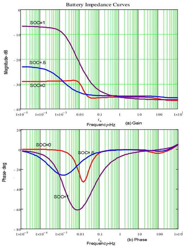
Figure 17 Battery Impedance (a) Gain and (b) phase plots at SOC=1, SOC=.5, SOC=0
