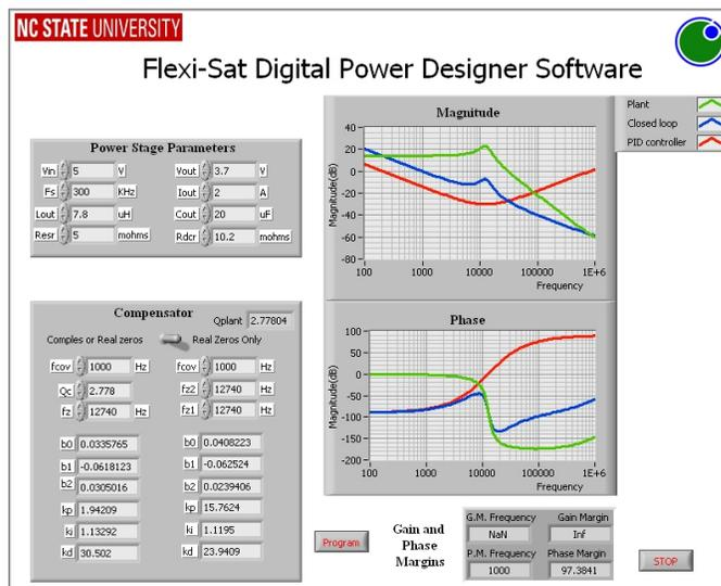
**Figure 10 Flexi-sat Digital Power Designer Software configuring the FDPOLs**
