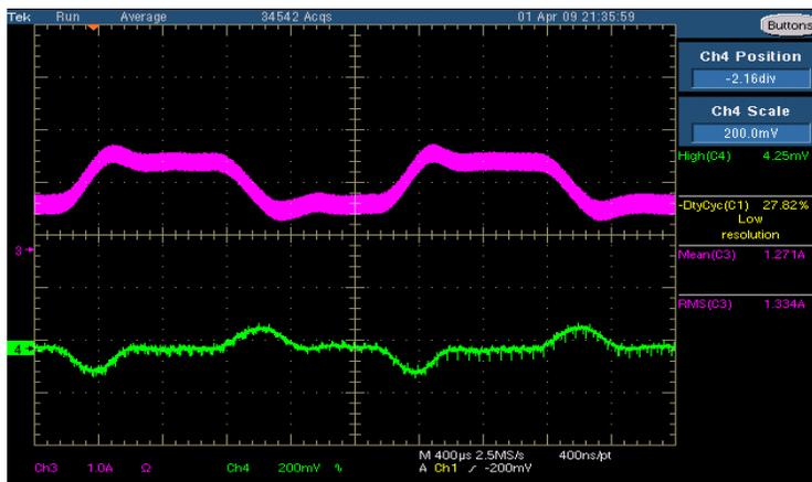
Figure 66 Transient performance of Buck regulator: 1A-2A step, 100mA/uSec slew rate
