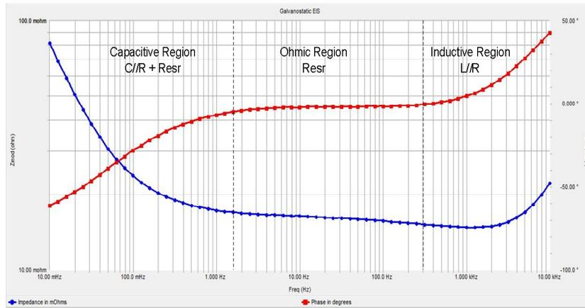
Figure 39 Galvanostatic EIS measurement Bode plot for Li-ion battery at SOC=1 at 0mA dc
