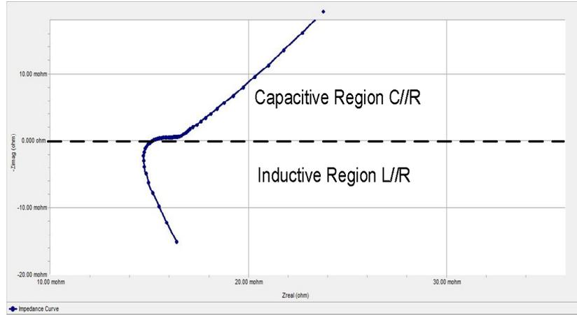
**Figure 40 Galvonostatic EIS measurement Nyquist plot for Li-ion battery at SOC=1 at 0mA dc**
