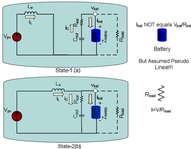
Figure 25 Linear equivalent circuit for each state of the boost converter in CCM
