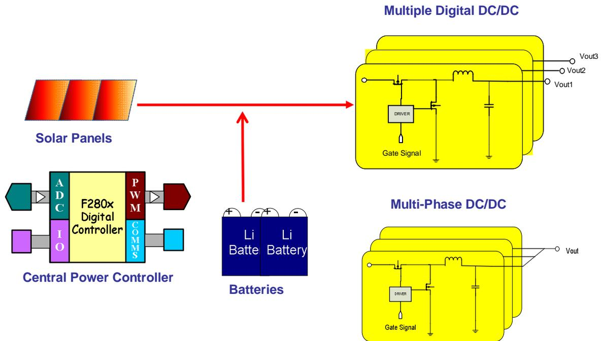
Figure 9 FDPOL modules providing regulated DC Bus for the satellite sub systems
