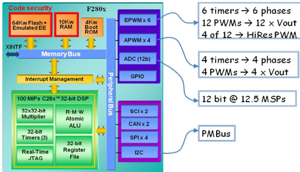
Figure 49 Central controller engine architecture
