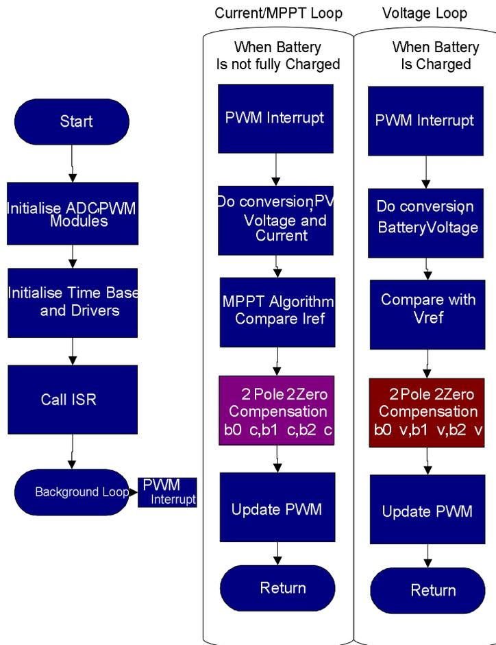
**Figure 54 Software Algorithm for Current/MPPT loop**
