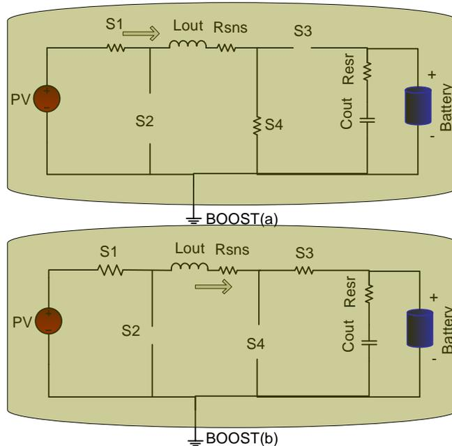
**Figure 13 (a) Boost Inductor charge and (b) Inductor discharge**
