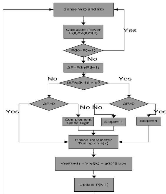
Figure 45 Adaptive P&O methodology flow chart
