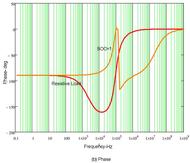
**Figure 30 Output Voltage Loop DCM (a) Gain and (b) phase for All SOCs and resistive load**
