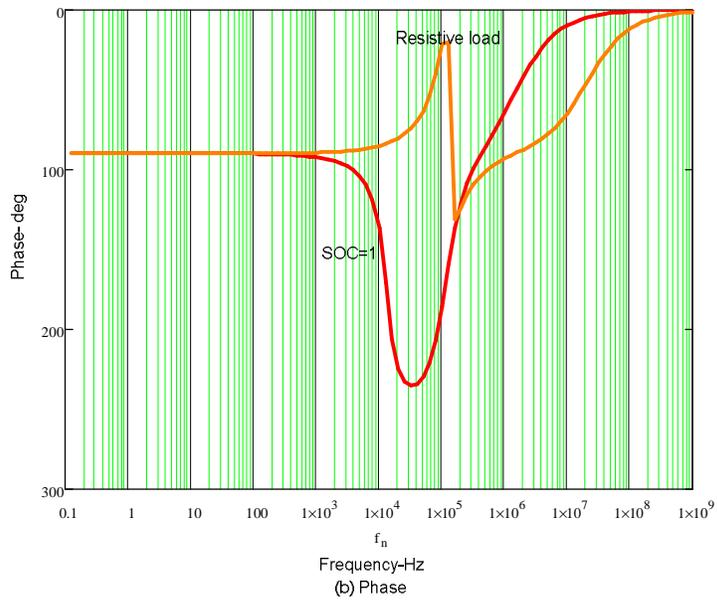
**Figure 24 Output Voltage Loop (a) Gain and (b) phase for SOC=1 and resistive load**
