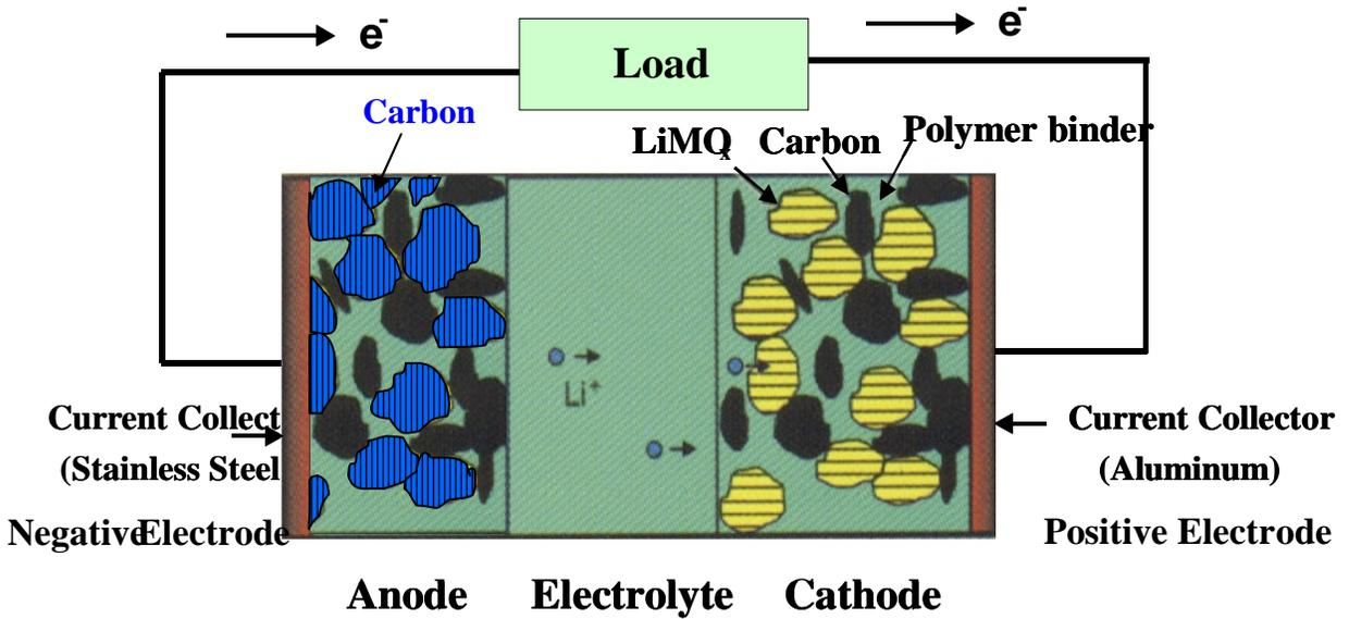
**Figure 31 Active positive and negative materials in a Lithium Ion Cell**
