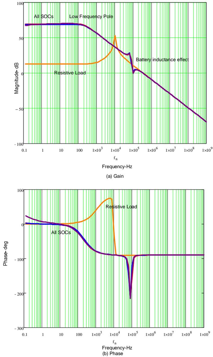
**Figure 27 Control-to- Charge Current Transfer Function (a) Gain and (b) phase plots at all SOC's and  $Z_L=150\Omega$**
