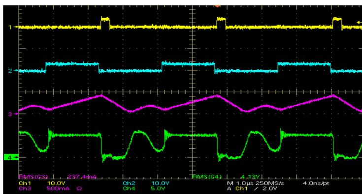
Figure 67 Non Synchronous Buck operation during light load operation
