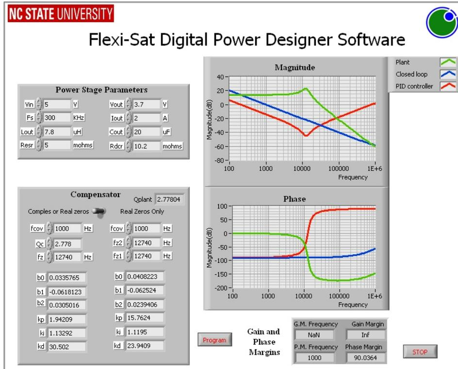
Figure 62 Flexi-Sat Digital Power Designer Software-showing design with complex compensator
