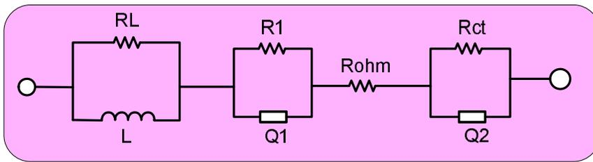
**Figure 16 Equivalent circuit diagram of the battery**
