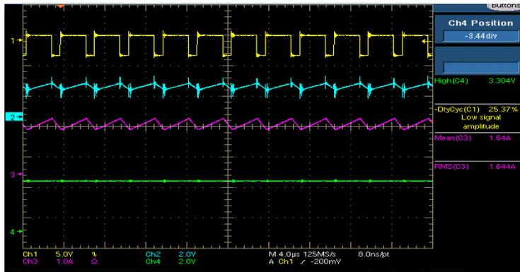
Figure 65 Voltage Regulation for Buck Converter  $V_{in}=5V$ ,  $V_{out}=3.3V$ ,  $I_{out}=2A$
