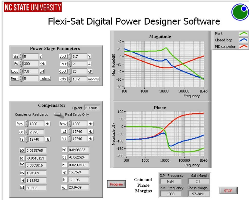
**Figure 60 Flexi-Sat Digital Power Designer Software-showing design with real compensator**
