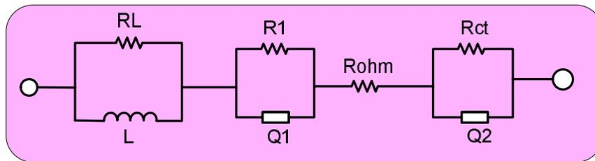
**Figure 26 Equivalent circuit diagram of the battery**
