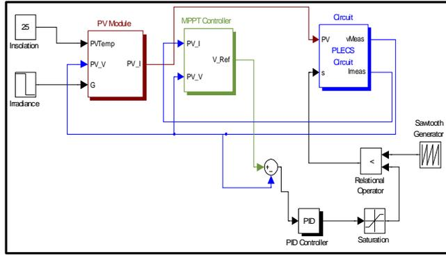
**Figure 47 Simulation of MPPT algorithm implementation in MATLAB, Simulink**
