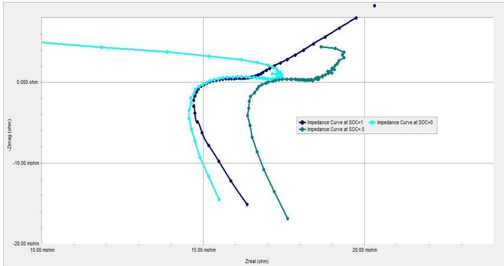
**Figure 43 Galvonostatic EIS measurement Nyquist plot for Li-ion battery for**
