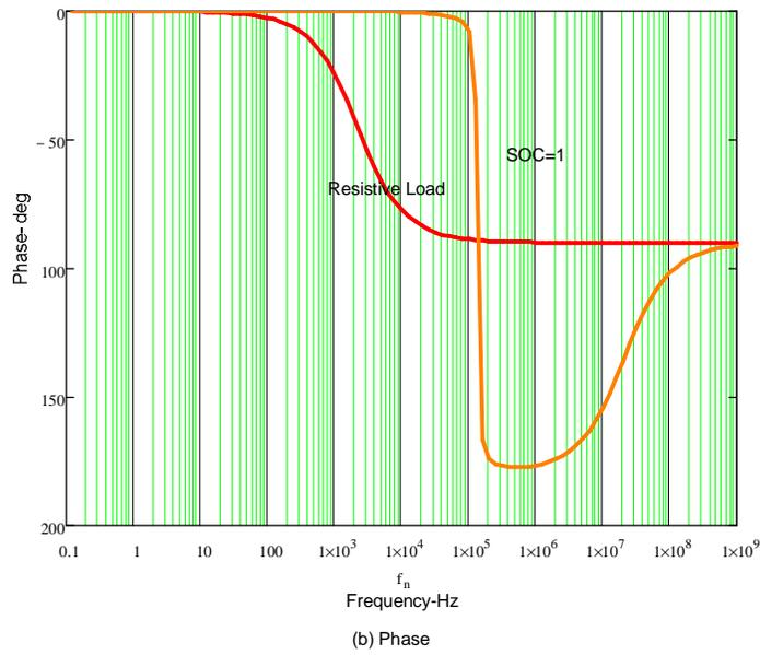
**Figure 28 Control-to-Output Voltage Transfer Function DCM (a) Gain and (b) phase plots**
