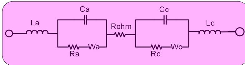
Figure 38 Electrochemical Equivalent Model
