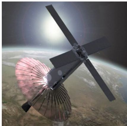
Figure 3. AENEAS – A 3U CubeSat [3]
