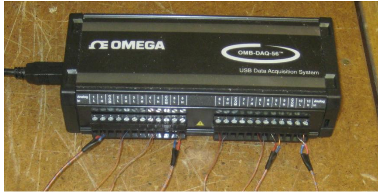
Figure 3.1: DAQ Device Containing 10 Thermocouple Attachments
