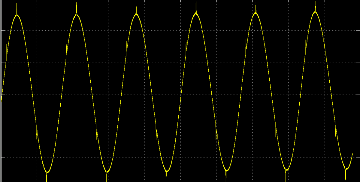
FIGURE 2.6 SOURCE CURRENT OF CLOSED LOOP CIRCUIT
