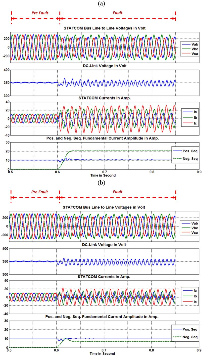
Figure 5-18. STATCOM performance with (b) and without (a) proposed controller when STATCOM is working in inductive mode
