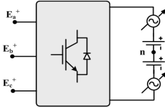
Figure 3-6. Equivalent circuit of the 3-Level NPC VSC used for calculation of the fundamental negative sequence voltage vector at VSC output terminals
