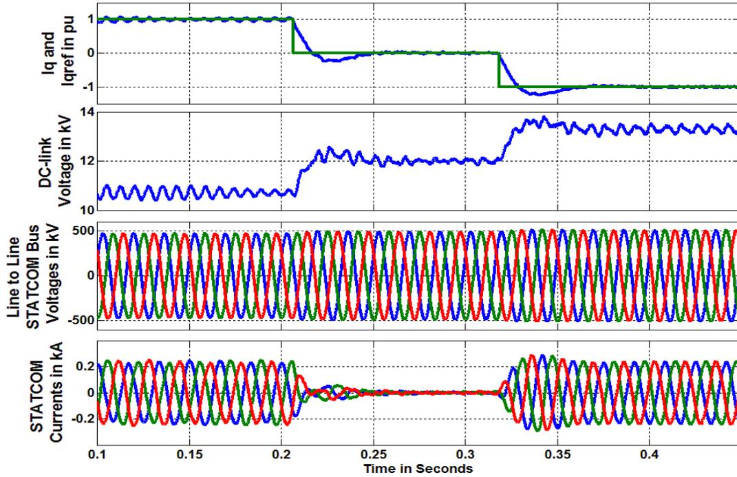
Figure 3-4. Angle-controlled STATCOM performance with two different instantaneous reactive current ( $I_q$ ) references
