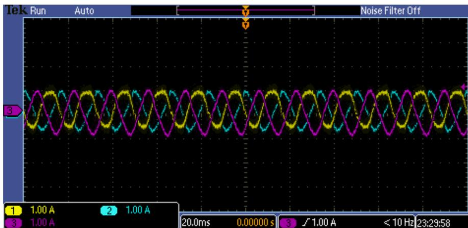
Figure 6-13. Converter currents under SLG fault at phase A when converter works with the proposed controller. Chanel 1, 2, and 3 indicate the  $I_a$ ,  $I_b$ , and  $I_c$  respectively. Current scale: 10A/div.
