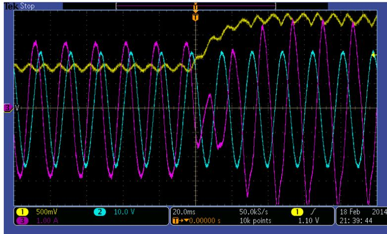
Figure 2-28. STATCOM transition from inductive mode  $I_q=0.6$  pu to capacitive mode  $I_q=-0.7$  pu
