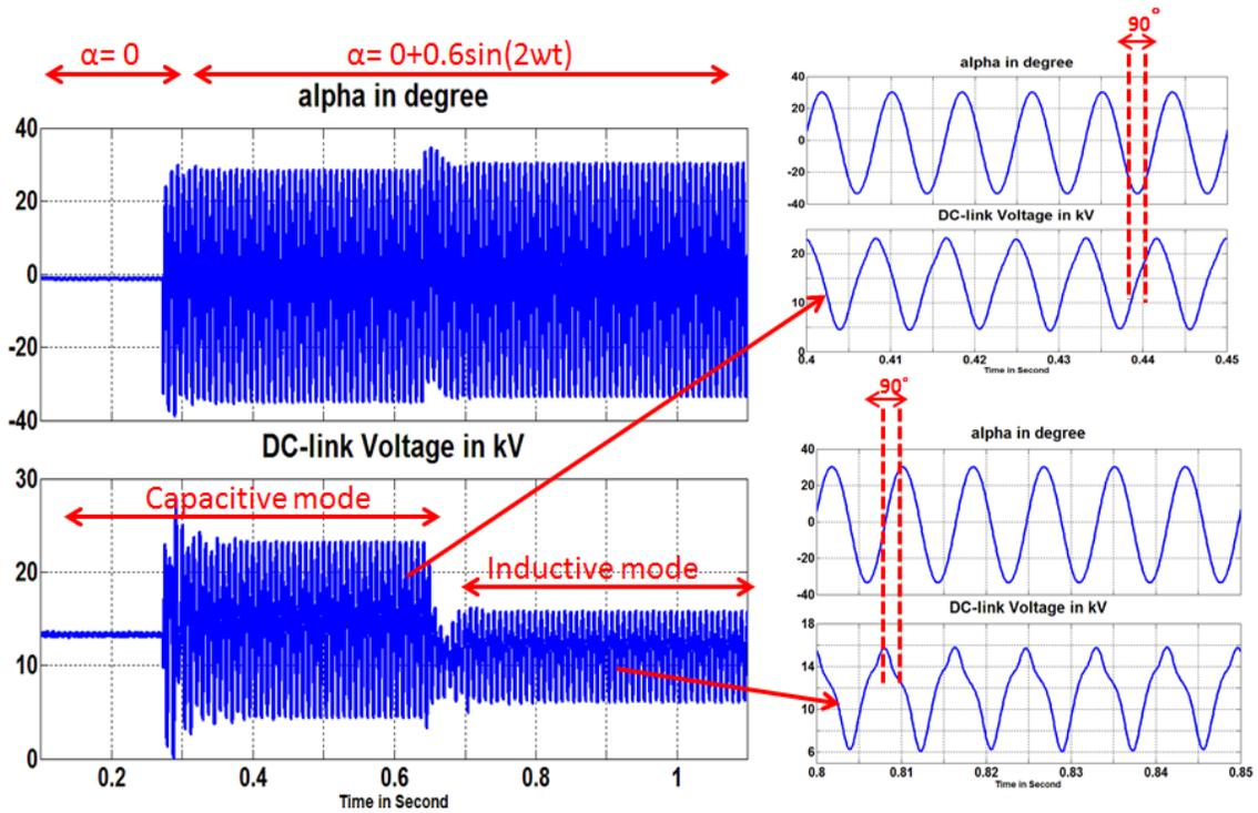
Figure 3-11. DC-link voltage 2nd harmonic oscillations generated by introducing 2nd harmonic oscillations to the  $\alpha$  in both capacitive and inductive operation modes
