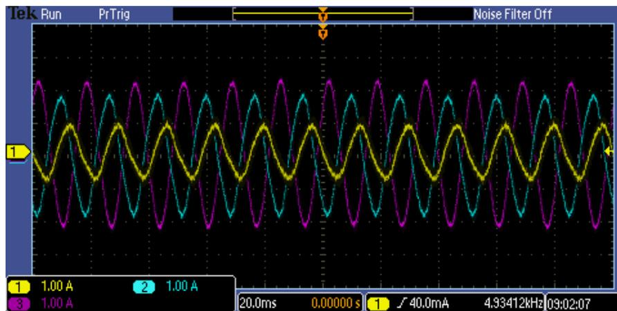
Figure 6-11. Converter currents under SLG fault at phase A when it works with conventional controller. Chanel 1, 2, and 3 indicate  $I_a$ ,  $I_b$ , and  $I_c$  respectively. Current scale: 10A/div
