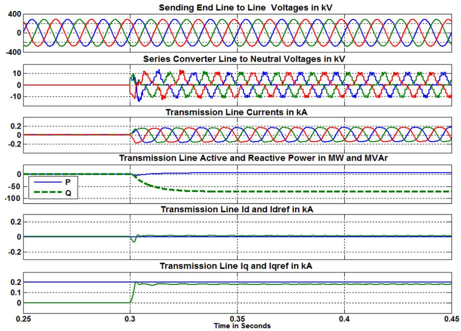
Figure 7-17. UPFC performance with a step change in the  $i_{q \text{ ref}}$  (reactive power reference).
