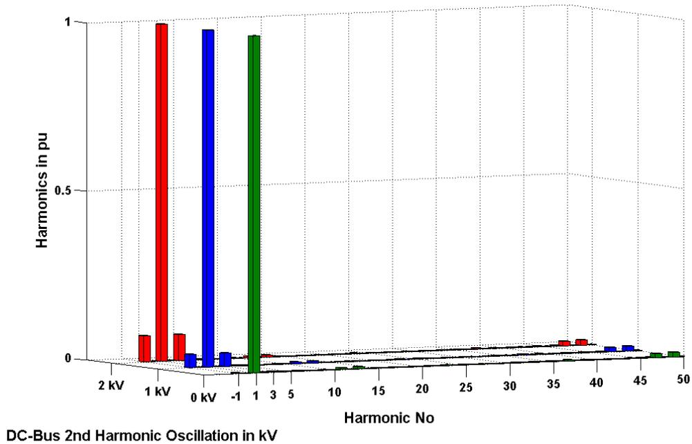
Figure 3-7. 48-pulse inverter output voltage harmonic content with different 2nd harmonic oscillations added to the DC-link voltage
