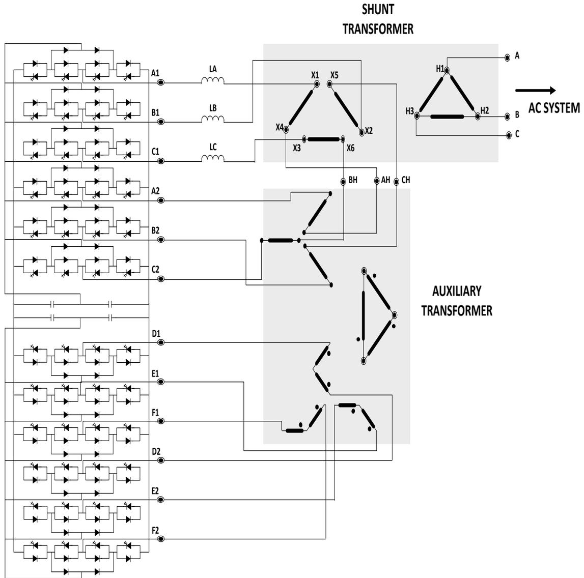
Figure 2-9. Power circuit of the NYPA three-level NPC 48-pulse inverter[30].
