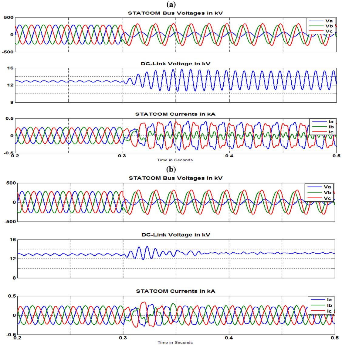
Figure 4-18. STATCOM performance with (b) and without (a) proposed solution under phase a SLG fault right at STATCOM bus (fault location1) when STATCOM is working in capacitive mode of operation.
