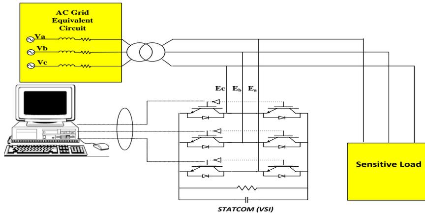
Figure 5-1. Voltage regulation of a load sensitive to voltage dip using a PWM VSC-based STATCOM
