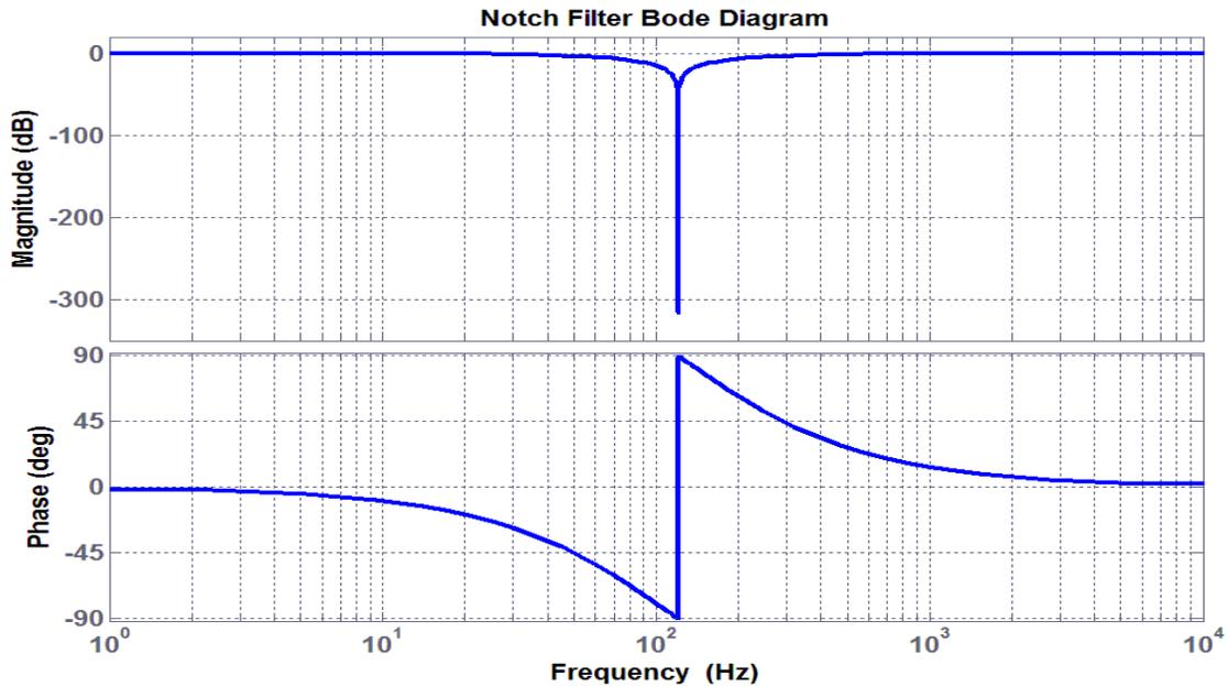
Figure 4-10. Notch filter bode plots
