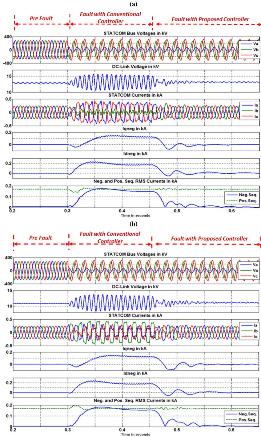
Figure 4-15. STATCOM performance with and without proposed solution under phase a SLG fault right at STATCOM bus (fault location1) when STATCOM is working in capacitive (a) and inductive (b) mode of operation. The current THD reaches from 1.2% before fault to around 2.9% after fault with proposed controller in both inductive and capacitive modes.
