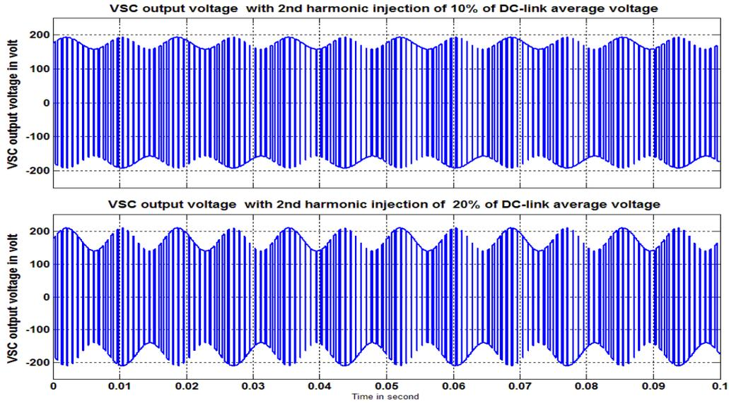
Figure 5-5. VSC output voltage with 2nd harmonic injection of 10% and 20% of the DC-link average voltage
