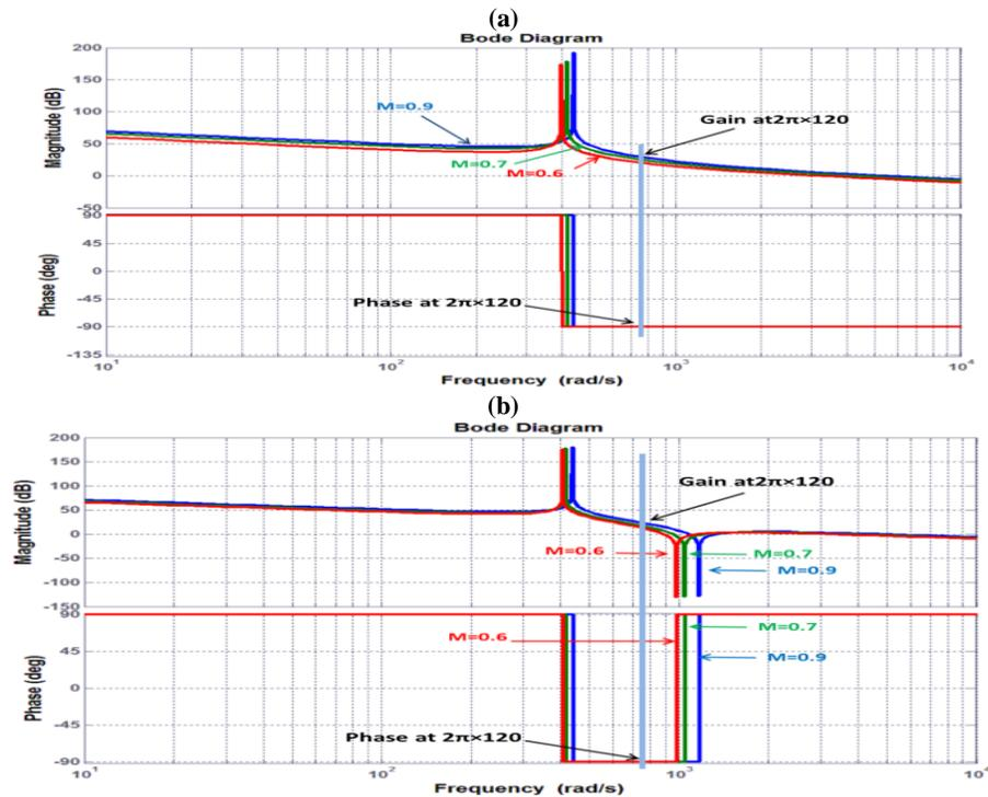
Figure 5-11. Bode plots of the DC-link voltage perturbation against  $\alpha$  perturbation around one capacitive (a)/inductive (b) equilibrium point with different modulation index.
