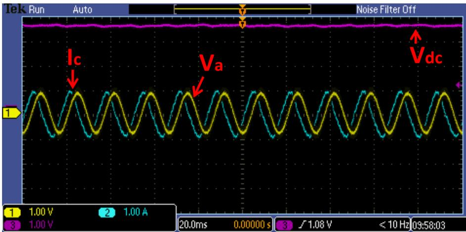
Figure 6-15. Converter performance with the proposed controller under SLG fault at phase A.
