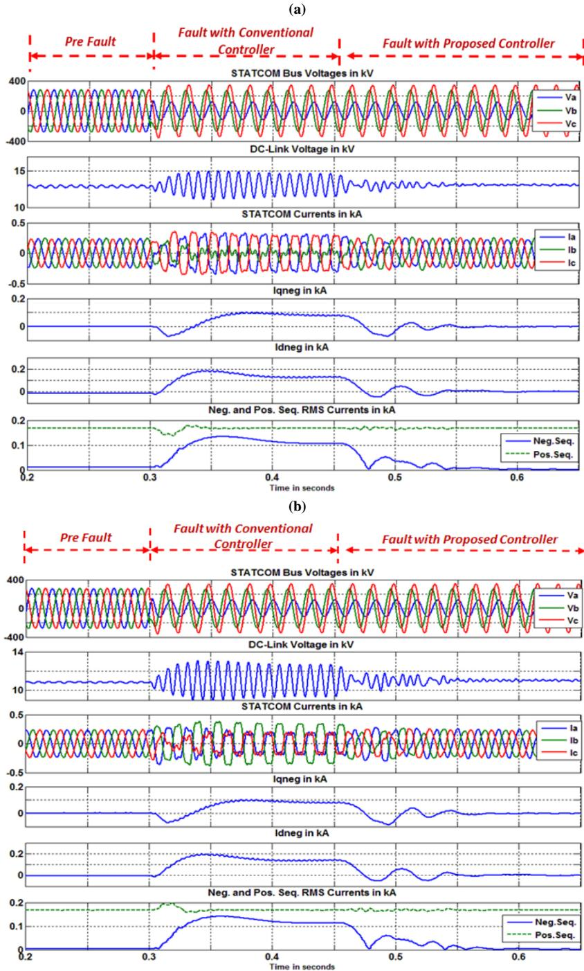
Figure 4-16. STATCOM performance with and without proposed solution under phase a SLG fault in the middle of the Marcy-Bus1 345 kV transmission line (fault location2) when STATCOM is working in capacitive (a) and inductive (b) mode of operation. The current THD reaches from 1.2% before fault to around 2.3% after fault with proposed controller in both inductive and capacitive modes.
