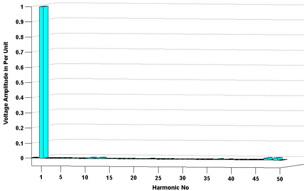
Figure 2-11. 48-pulse inverter output voltage harmonic content
