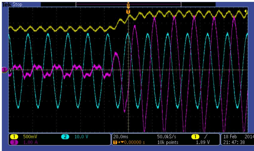
Figure 2-30. The STATCOM transition from zero current  $I_q=0$  pu to capacitive mode  $I_q=-0.7$
