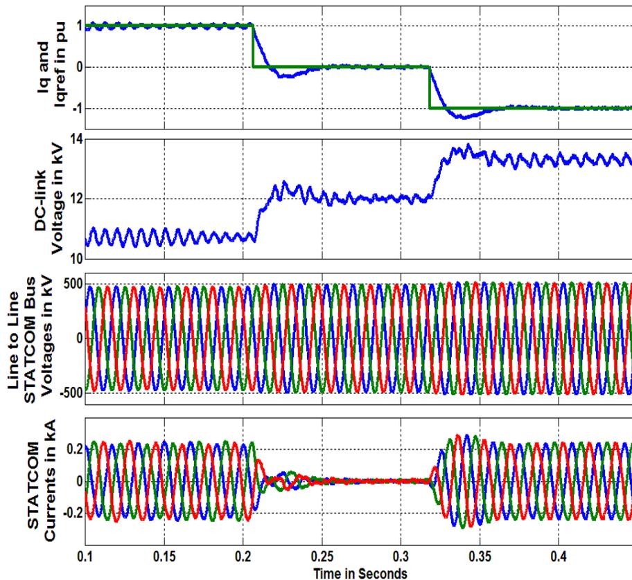
Figure 7-7. 48-pulse angle-controlled STATCOM performance with different current references. Per unit values are based on 345kV, and 100 MVA system
