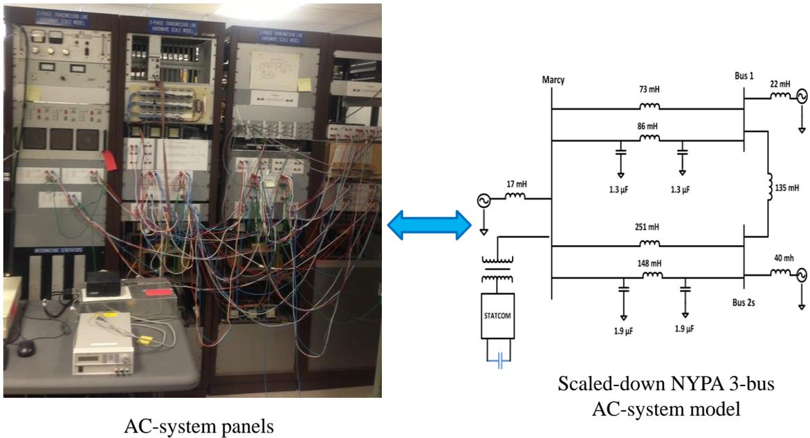
Figure 2-22. Scaled down model of the NYPA 3-bus AC system used for experimental verification
