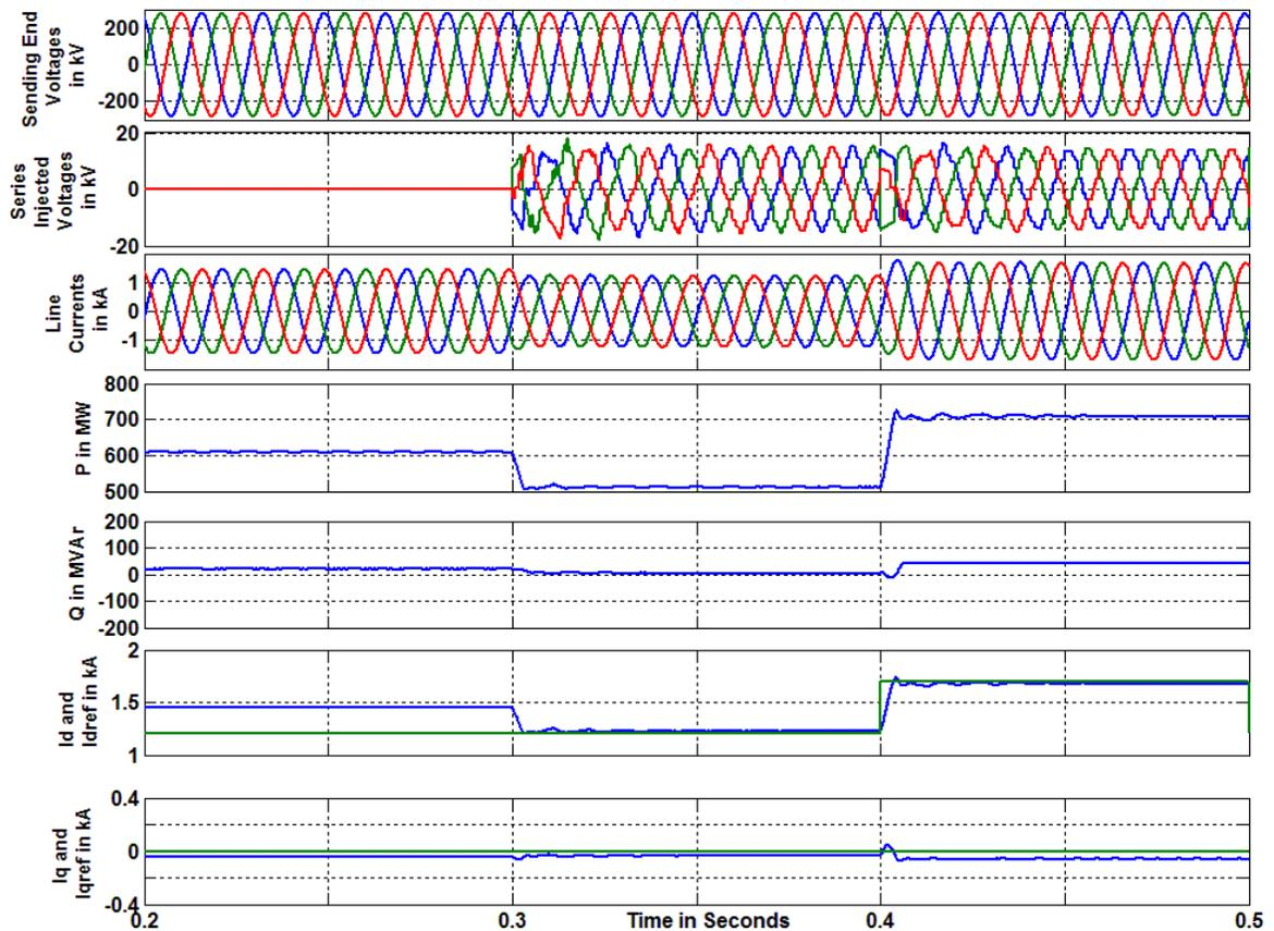
Figure 7-22. Simulated UPFC performance with different active and reactive power references
