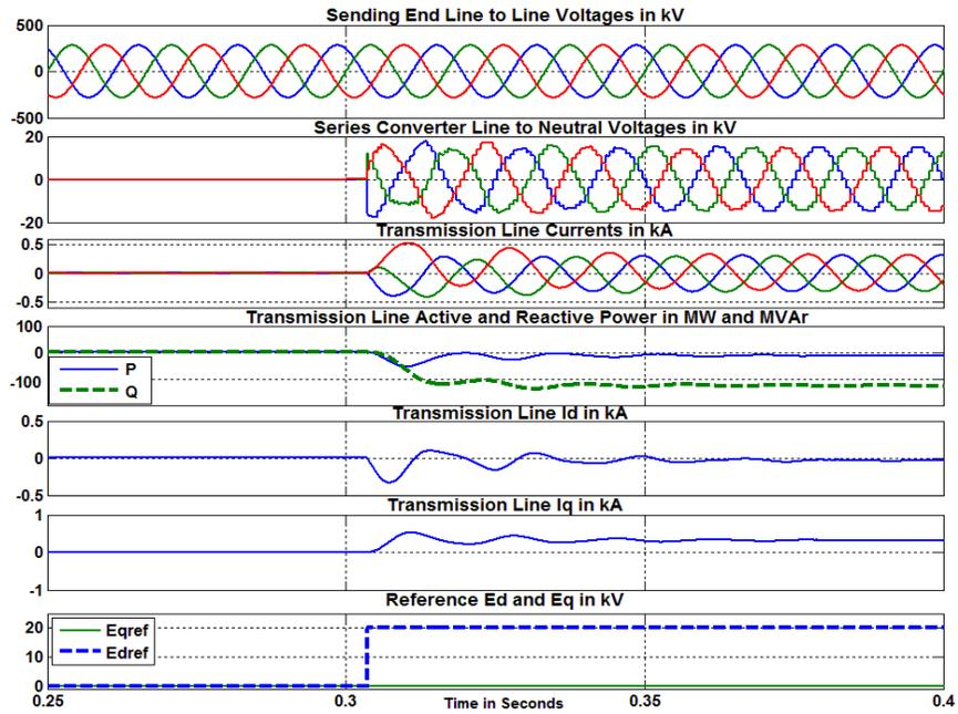
Figure 7-11. The UPFC performance with a step change in the d component of the series inverter voltage reference value. (The UPFC works in the voltage injection mode)
