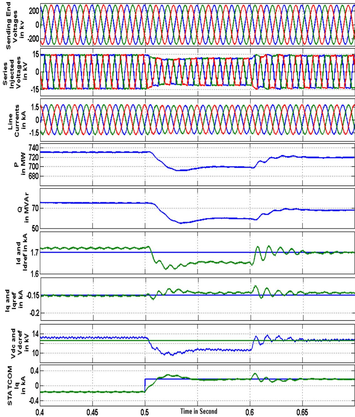
Figure 7-26. UPFC performance when the shunt inverter operating point changes form fully capacitive to fully inductive with and without proposed solution. The desired DC-link voltage is set to 12.5 kv ( $\sigma_{cal} = 31.7^\circ$ ).
