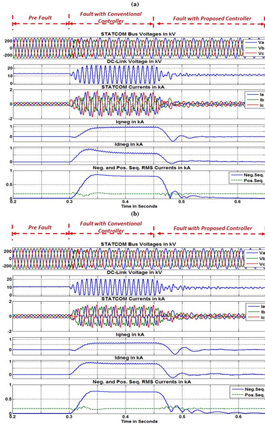
Figure 4-17. STATCOM performance with and without proposed solution under Line to Line fault between phase b , and c in the middle of the Marcy-Bus1 345 kV transmission line (fault location2) when STATCOM is working in capacitive (a) and inductive (b) mode of operation. The current THD reaches from 1.2% before fault to around 23% after fault with proposed controller in both inductive and capacitive modes.
