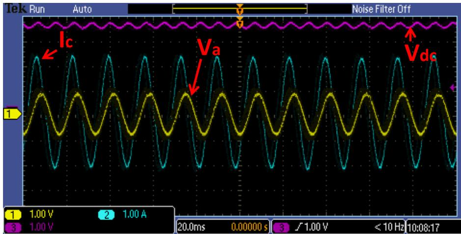
Figure 6-14. Converter performance with conventional controller under SLG fault at phase A.
