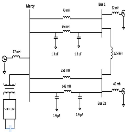
Figure 3-20. Scaled down model of the NYPA 3-bus AC system used for experimental verification
