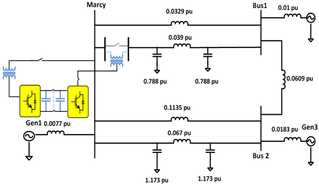
Figure 7-21. Simulation system, UPFC model based on the NYPA UPFC at Marcy substation is connected to the NYPA 3-bus AC-system. All the per unit values are based on 100 MVA and 345kV system.
