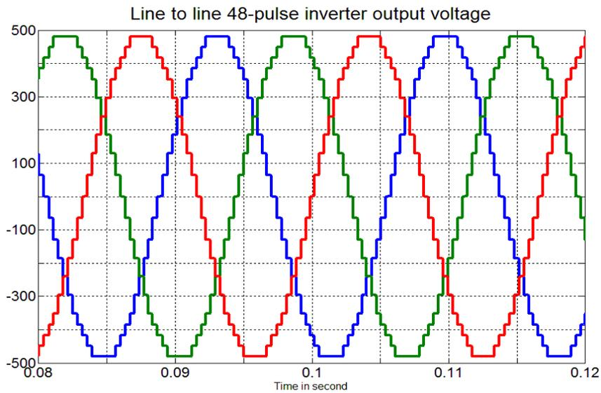
Figure 3-3. 48-pulse inverter line to line output voltages.
