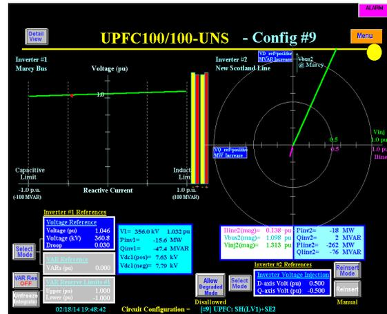
Figure 2-27. Operator Control Screen for UPFC
