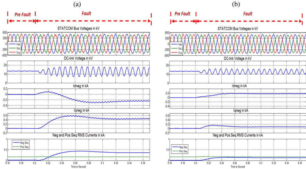
Figure 3-17. STATCOM performance with (b) and without (a) proposed DAC when STATCOM is working in capacitive mode and SLG fault at phase C is applied in the middle of the Marcy-Bus2 345 kV outgoing transmission line in the 3-bus AC system . (PSCAD/EMTDC simulation results)
