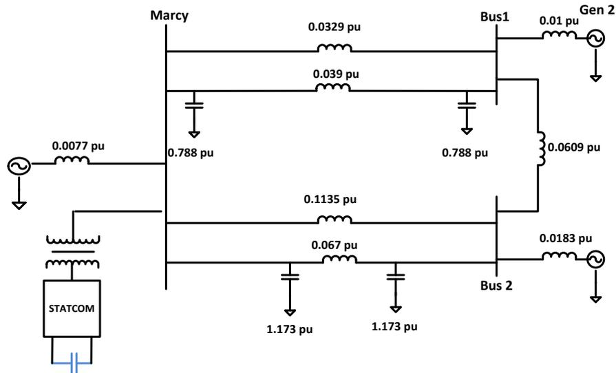
Figure 2-12. The angle-controlled STATCOM connected to the NYPA 3-bus AC system. Per unit values are based on 345kV, and 100 MVA.
