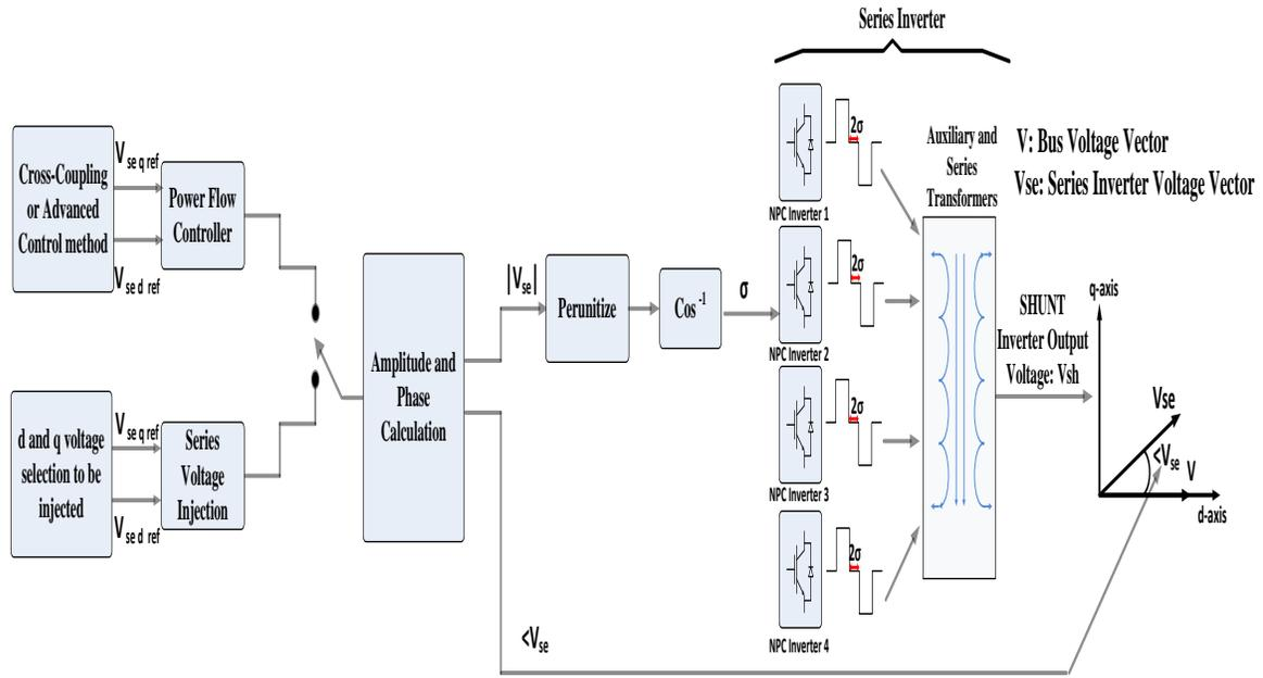
Figure 7-9. Series 48-pulse inverter control
