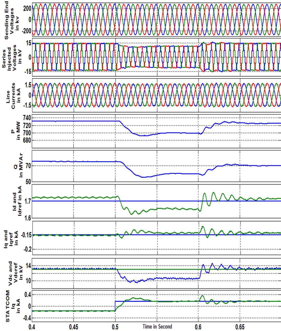
Figure 7-24. UPFC performance when the shunt inverter operating point changes form fully capacitive to fully inductive with and without proposed solution. The desired DC-link voltage is set to 13kv ( $\sigma_{cal} = 35.1^\circ$ ).
