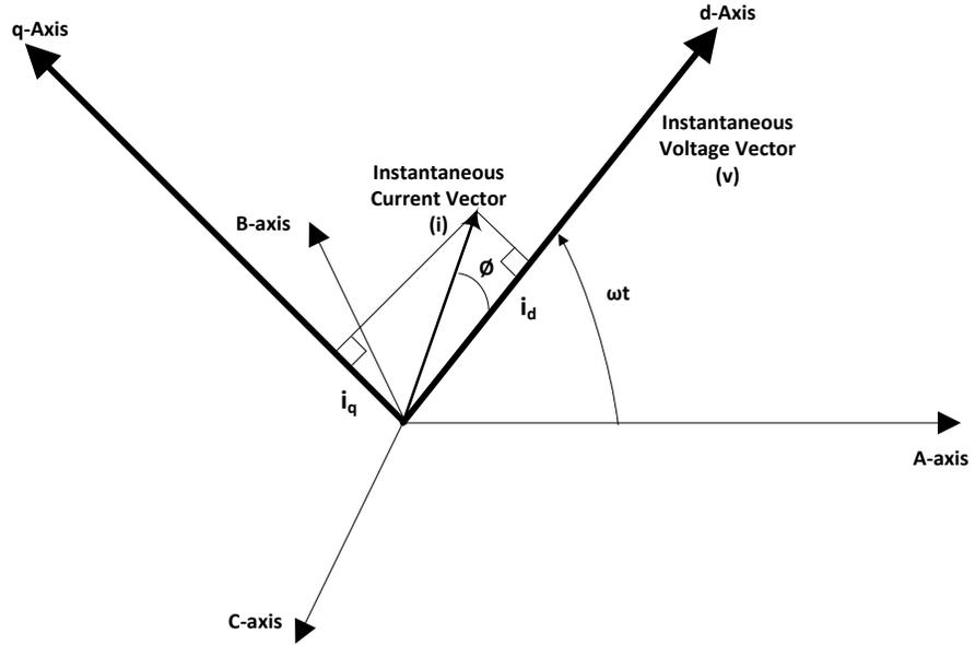
Figure 2-3. Instantaneous vectors in synchronous frame (dq)
