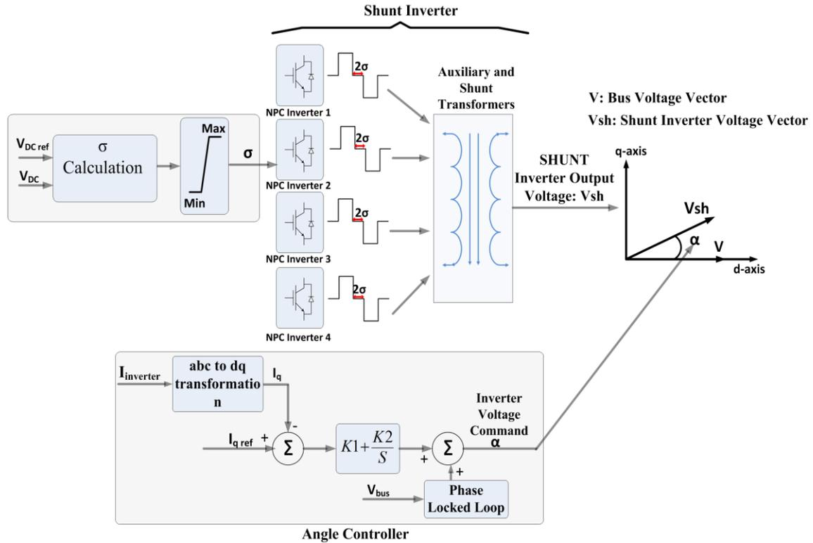
Figure 7-20. Proposed control structure
