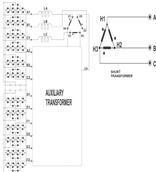
Figure 3-21. Power circuit topology of the inverters connected to auxiliary and shunt transformers to construct 48-pulse output voltage waveform
