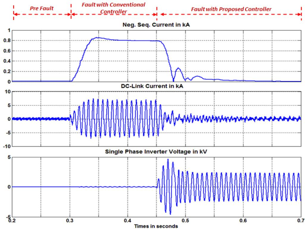
Figure 4-19. STATCOM negative-sequence current and single phase inverter current and voltage under a Line to Line fault in the middle of the Marcy-Bus1 345 kV transmission line
