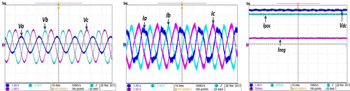
Figure 5-23. Inductive mode performance of the STATCOM under SLG fault with proposed controller. Voltage scale: 100V/div. and Current scale:5A/div.
