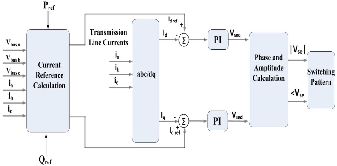
Figure 7-4. Cross-coupling controller
