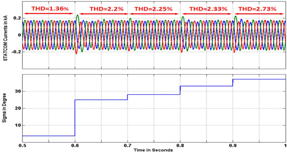
Figure 7-28. UPFC shunt inverter currents and their THD with different  $\delta$  values.
