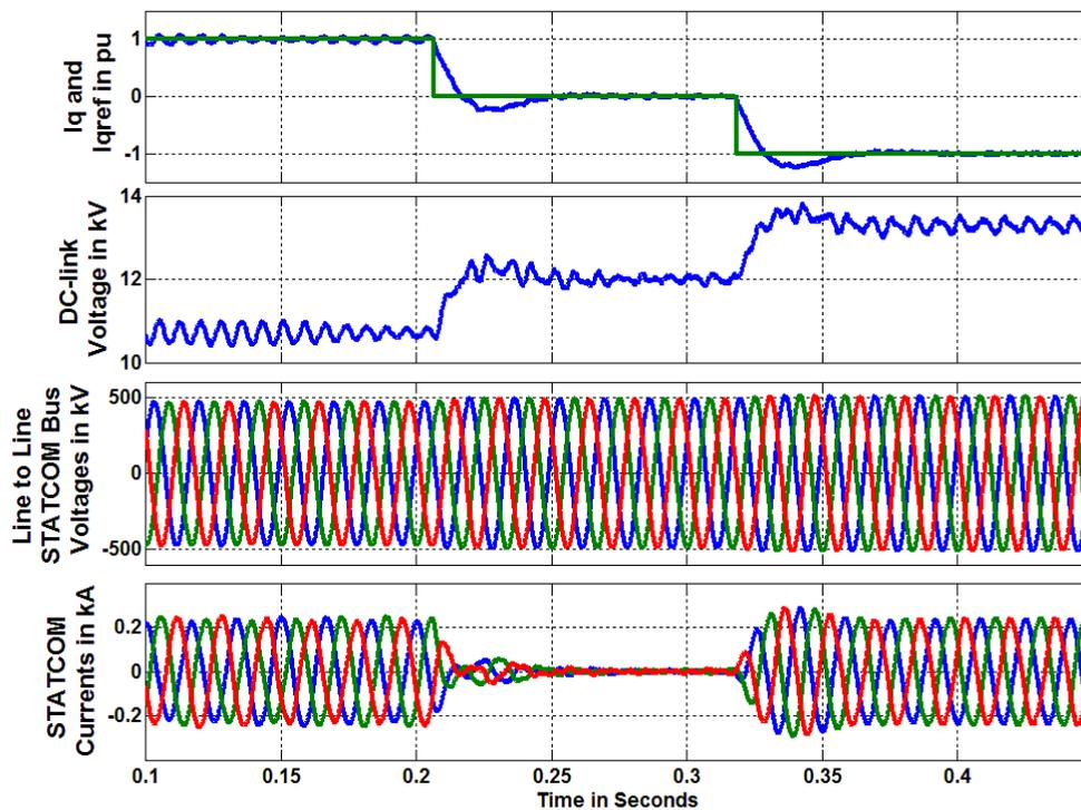
Figure 2-13. 48-pulse angle-controlled STATCOM performance with different current references. Per unit values are based on 345kV, and 100 MVA.
