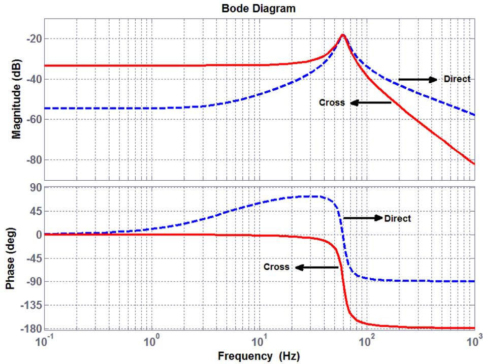
Figure 7-3. Bode plots of the direct and cross transfer functions.  $R=4\Omega$ ,  $L=0.123\text{ H}$  ( $X/R=11.6$ ). The  $R$ , and  $L$  values are based on the 345 kV simulation AC-system explained in the section 7.7
