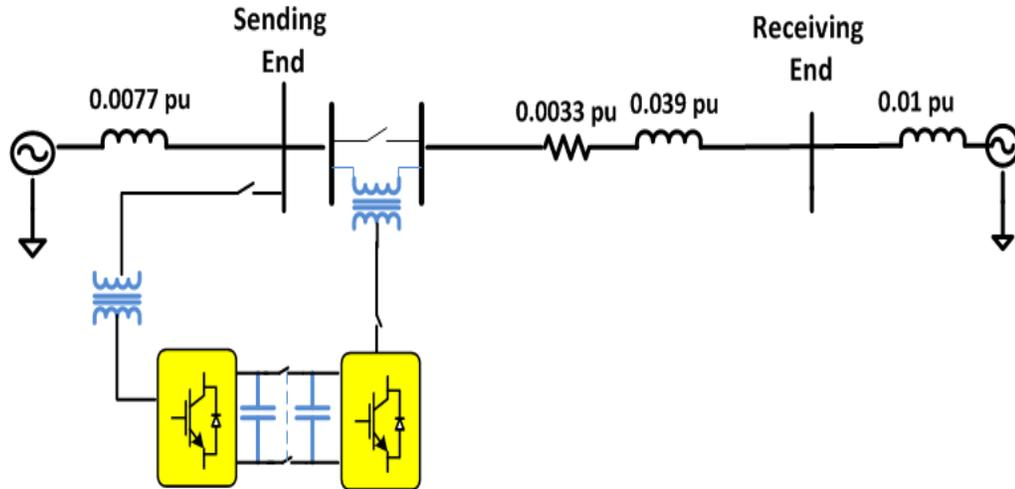
Figure 7-10. PSCAD UPFC model developed based on the NYPA UPFC at Marcy substation connected to the 2-Machine AC-system
