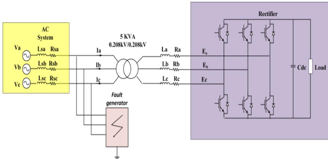
Figure 6-4. Single line diagram of the simulated test system
