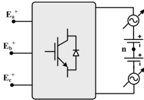
Figure 4-4. Equivalent circuit of the inverter used for calculation of the fundamental negative-sequence voltage vector at VSC output terminals.
