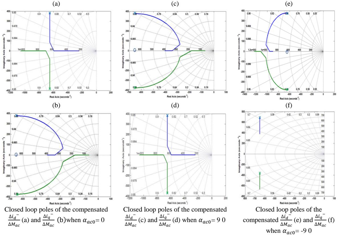
Figure 5-15. Closed loop root locus of the compensated  $\frac{\Delta i_d^-}{\Delta M_{ac}}$  and  $\frac{\Delta i_q^-}{\Delta M_{ac}}$  with three different values of  $\alpha_{ac0}$  i.e. 0, 90, and -90
