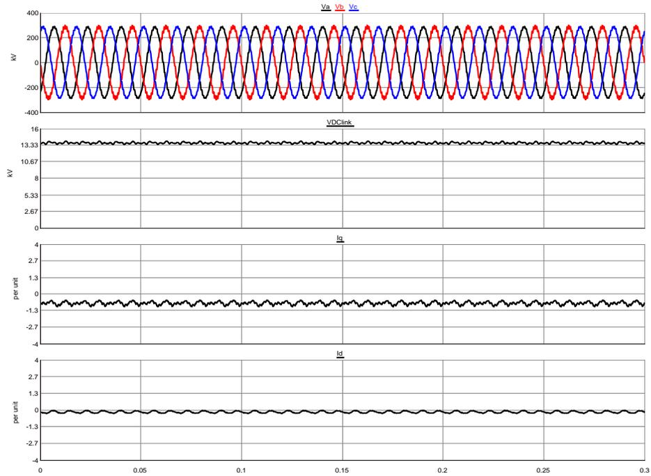
Figure 2-18. Angle-controlled STATCOM performance with  $i_q=-1$  pu capacitive
