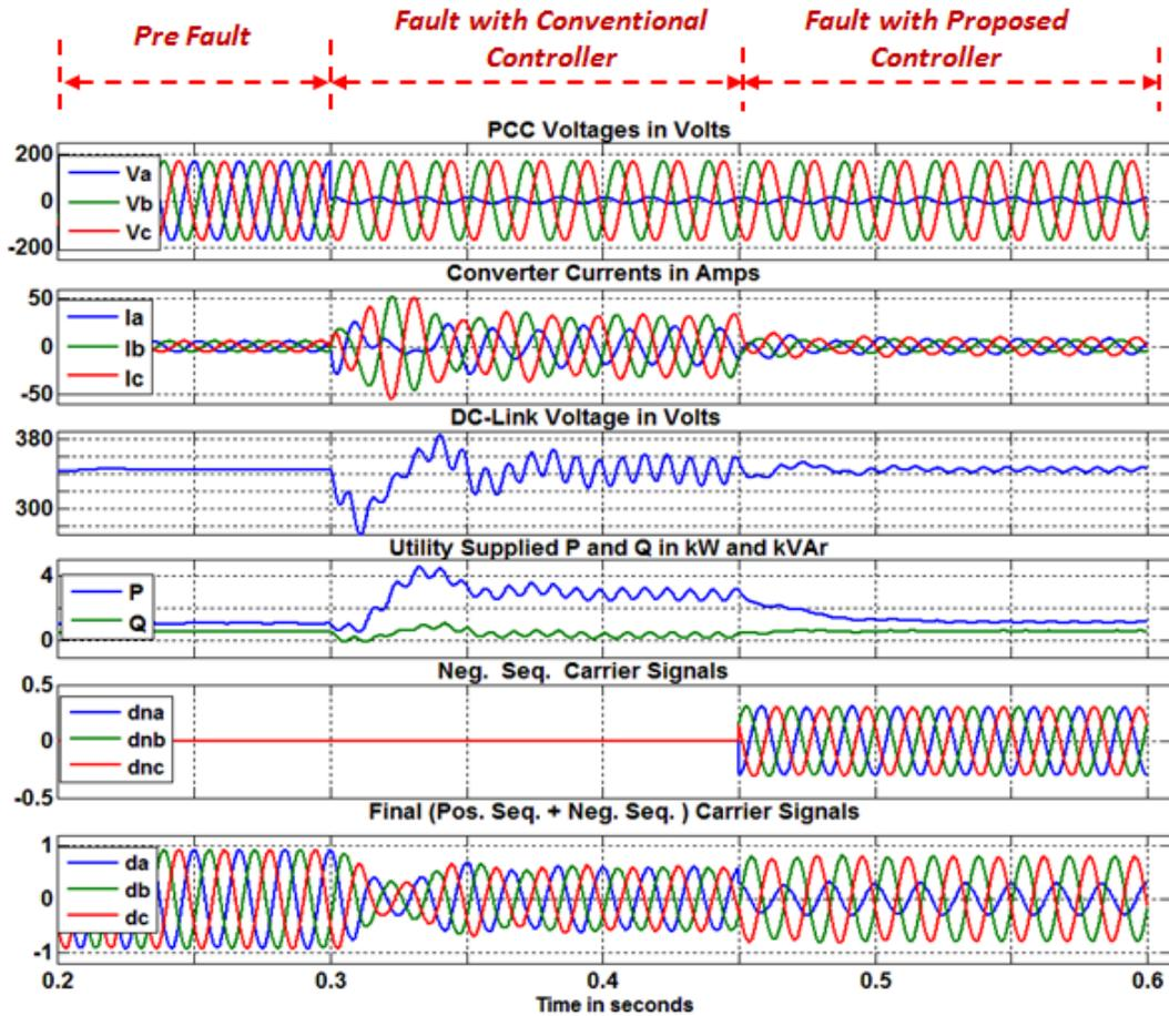
Figure 6-7. Converter performance with and without proposed controller under SLG fault at phase A right at PCC
