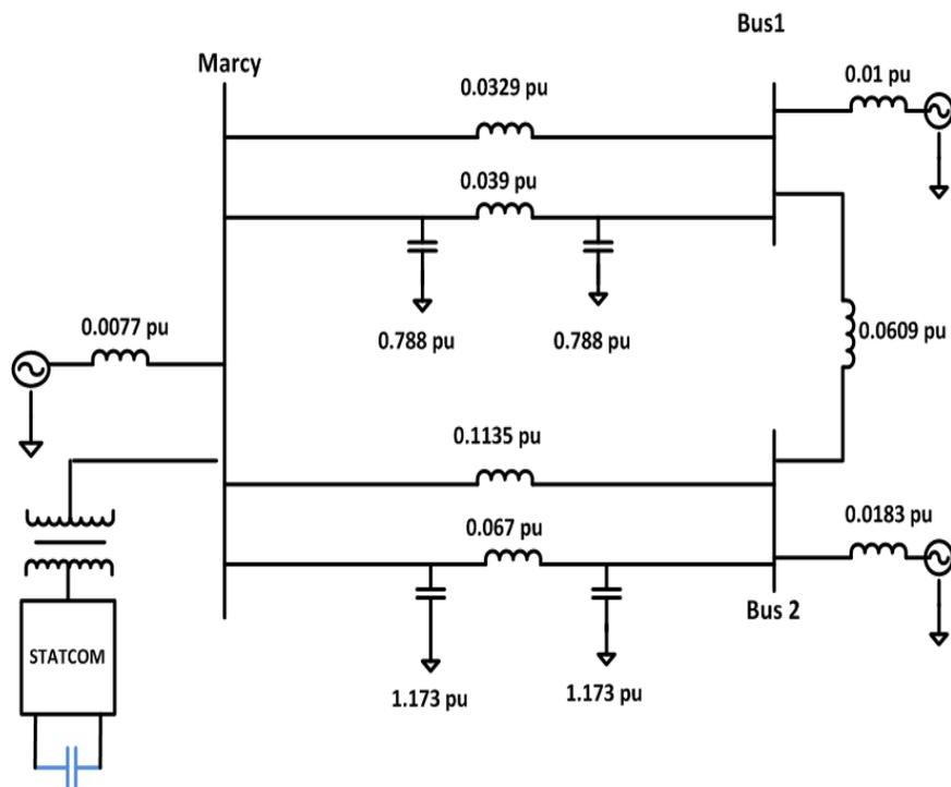
Figure 3-13. 3-bus AC system model. All the pu values are based on 345 kV and 100 MVA
