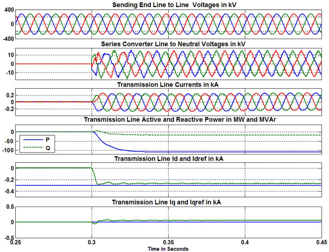
Figure 7-16. UPFC performance with a step change in the  $i_{d\ ref}$  (active power reference). UPFC series inverter is controlled with advanced control method.
