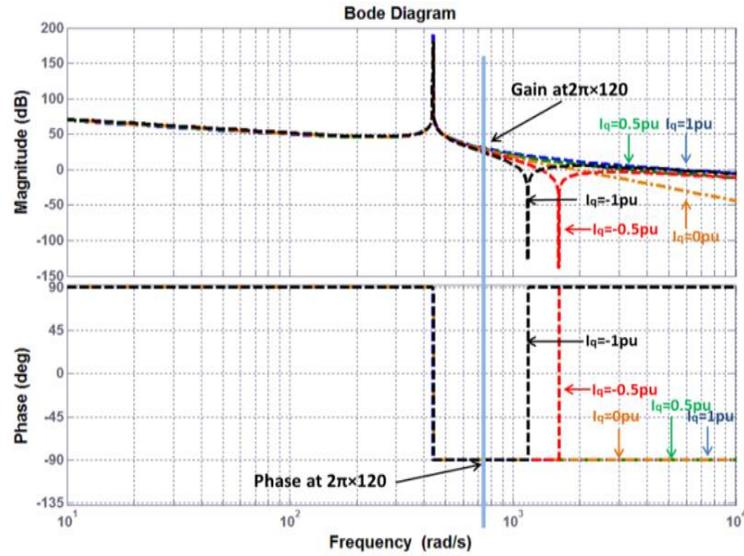
Figure 5-10. Bode plots of the DC-link voltage perturbation against  $\alpha$  perturbation around different inductive and capacitive equilibrium points. Positive and negative  $I_q$  corresponds to the capacitive and inductive mode of operations respectively.
