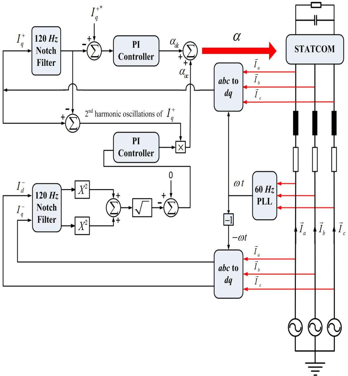
Figure 3-12. Proposed Control structure
