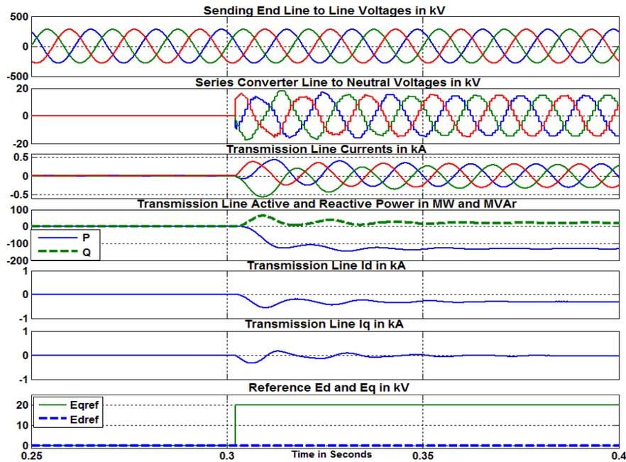
Figure 7-12. The UPFC performance with a step change in the q component of the series inverter voltage reference value. (The UPFC works in the voltage injection mode)
