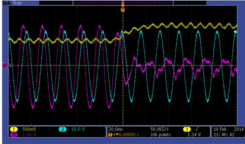
Figure 2-29. The STATCOM transition from inductive mode  $I_q=0.6$  pu to zero current  $I_q=0$
