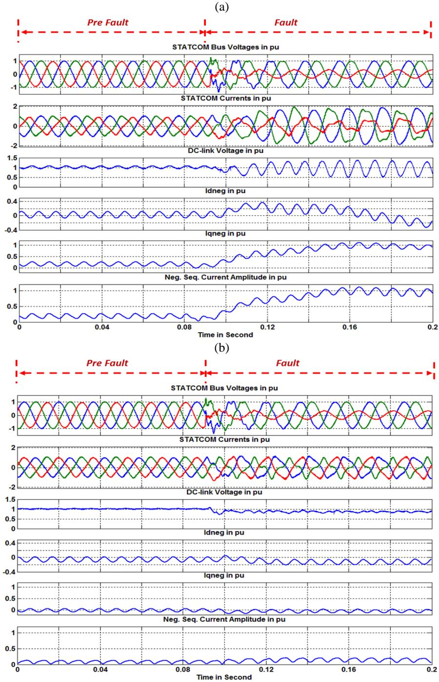
Figure 3-23. Capacitive mode performance of STATCOM under single line to ground fault with (b) and without (a) DAC. All pu values are based on 12 VA and 100 V RMS (L-L) ac system. (Experimental results)
