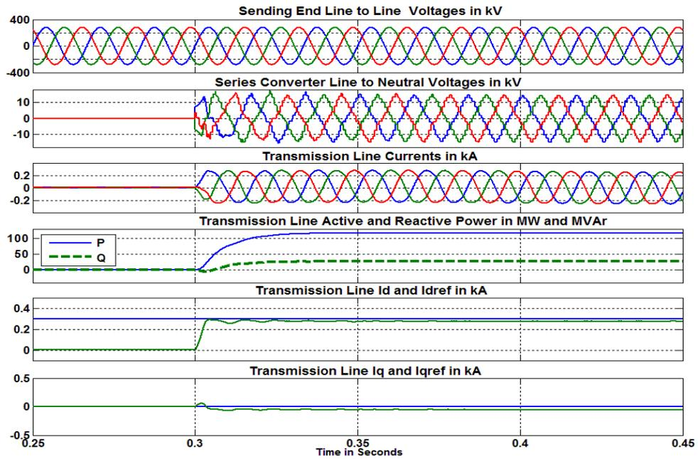
Figure 7-14. UPFC performance with a step change in the  $i_{d\text{ref}}$  (active power reference). UPFC works in power flow controller mode and series inverter is controlled with advanced control method
