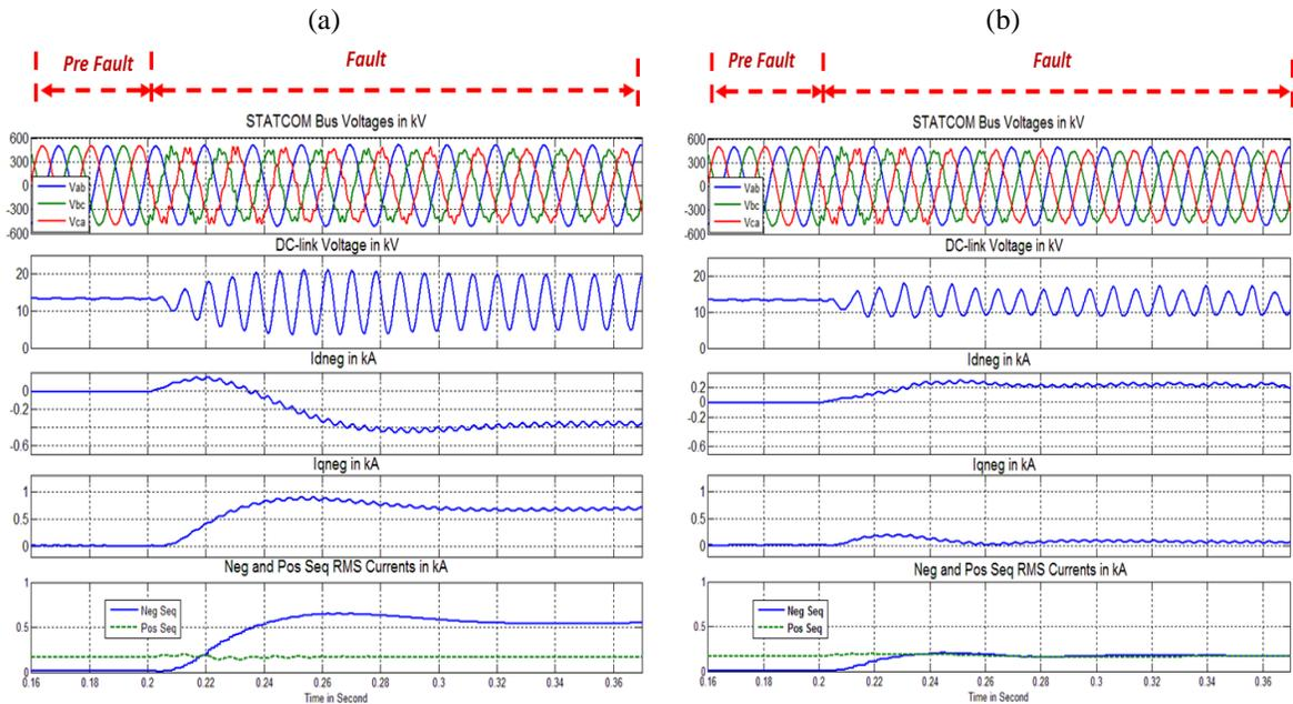
Figure 3-16. STATCOM performance with (b) and without (a) proposed DAC when STATCOM is working in capacitive mode and SLG fault at phase C is applied in the middle of the Marcy-Bus1 345 kV outgoing transmission line in the 3-bus AC system. (PSCAD/EMTDC simulation results)
