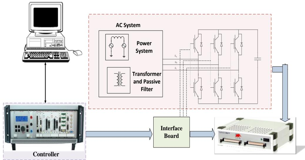
Figure 6-8. Hardware-in-the-Loop test system
