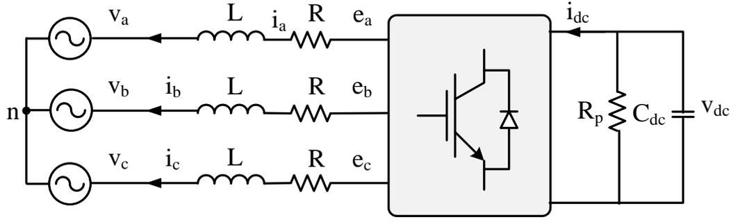
Figure 2-4. STATCOM connected to the AC-system
