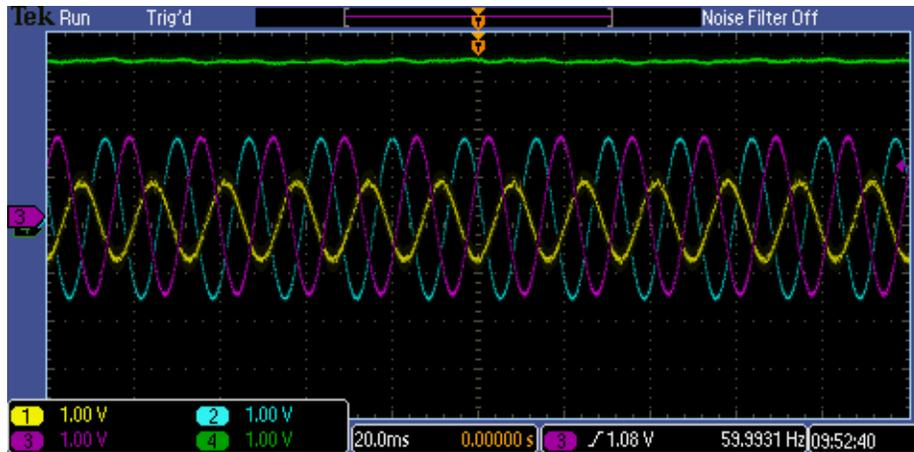
Figure 6-12. PCC and DC-link voltages under SLG fault at phase A when converter works with the proposed controller. Chanel 1, 2, 3, and 4 indicate the  $V_a$ ,  $V_b$ ,  $V_c$ , and DC-link voltage respectively. Voltage scale: 100V/div.
