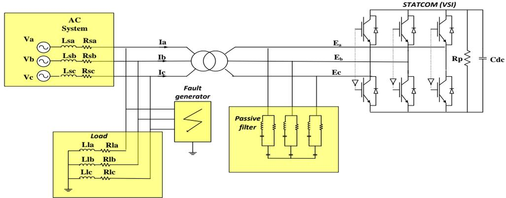
Figure 5-16. Single line diagram of the simulated test system
