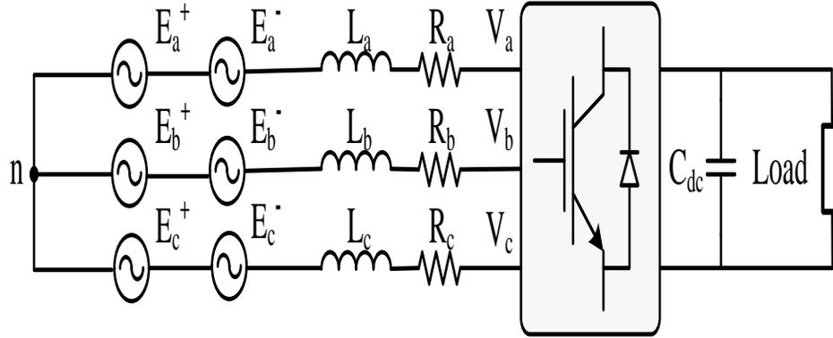
Figure 6-2. Converter equivalent circuit with series negative sequence voltage sources
