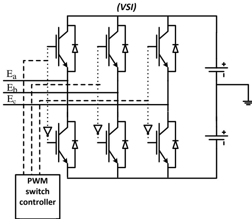
Figure 2-7. 2-level VSC-based PWM controlled inverter
