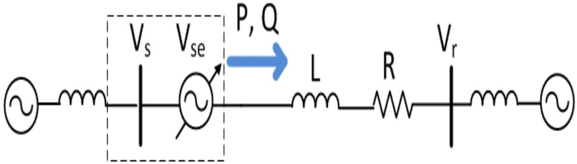
Figure 7-2. Simplified model of the UPFC connected to the sending end of the transmission line
