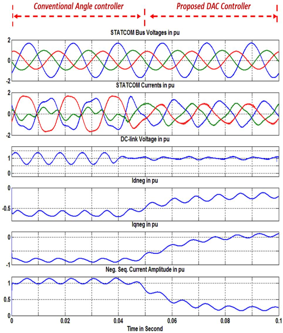
Figure 3-22. STATCOM performance with and without DAC in capacitive operation mode when there is 25% of negative sequence voltage injection at STATCOM bus. All pu values are based on 12 VA and 100 V RMS (L-L) ac system. (Experimental results)
