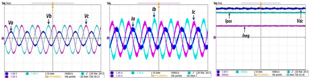
Figure 5-22. Inductive mode performance of STATCOM under SLG fault without proposed controller. Voltage scale: 100V/div. and Current scale:5A/div.
