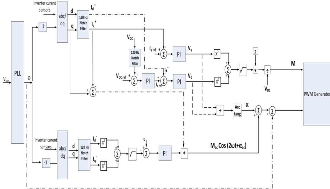
Figure 5-13. Proposed control structure
