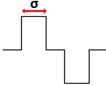
Figure 2-31. NPC converter output voltage
