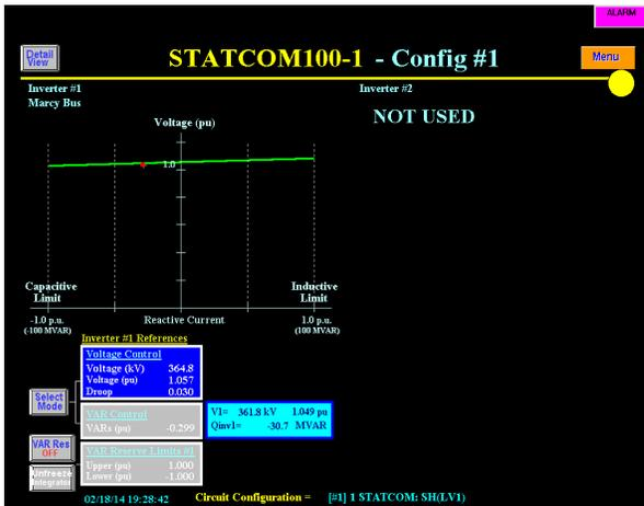
Figure 2-26. Operator Control Screen for STATCOM
