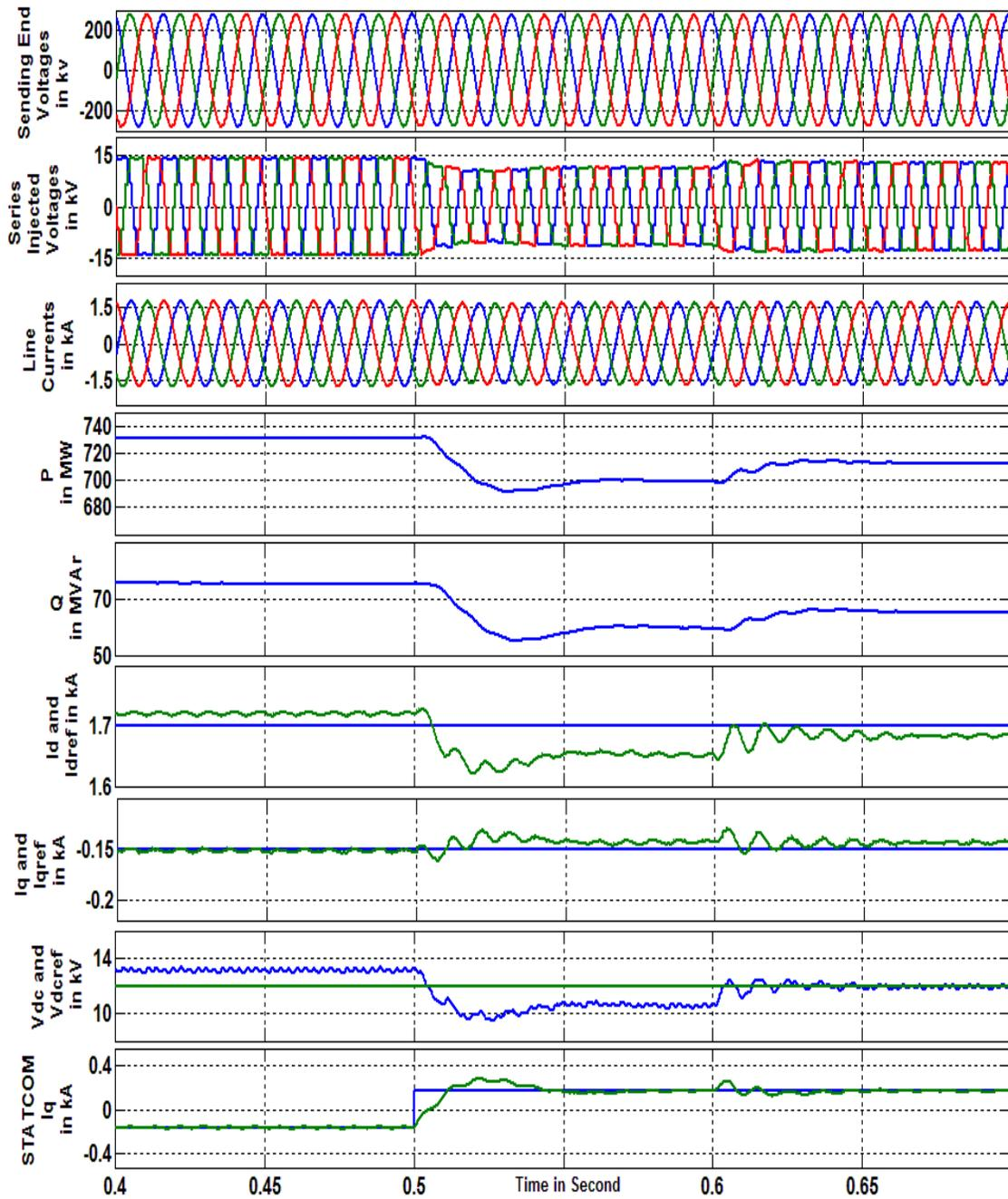
Figure 7-23. UPFC performance when the shunt inverter operating point changes from fully capacitive to fully inductive with and without proposed solution. The desired DC-link voltage is set to 12kV ( $\sigma_{cal} = 27.6^\circ$ ).
