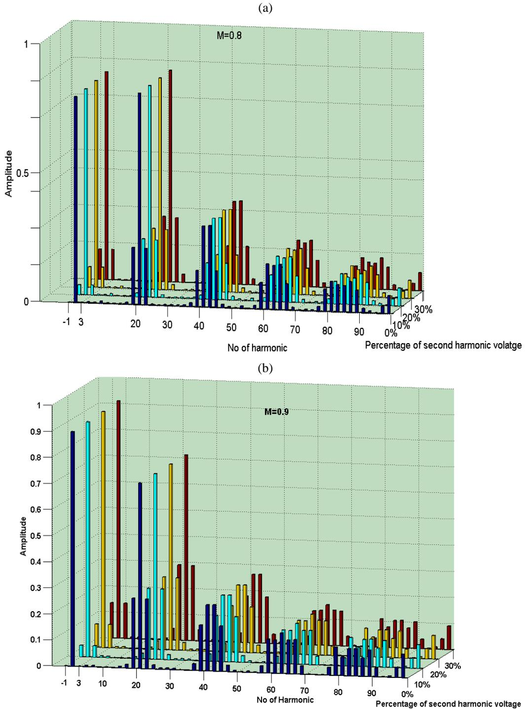
Figure 5-6. Inverter output voltage with modulation index of 0.8(a), and 0.9 (b) and switching frequency of 1260 Hz when different percentages of 2nd harmonic oscillations (with respect to the DC-link average voltage ) are added to the DC-link voltage.
