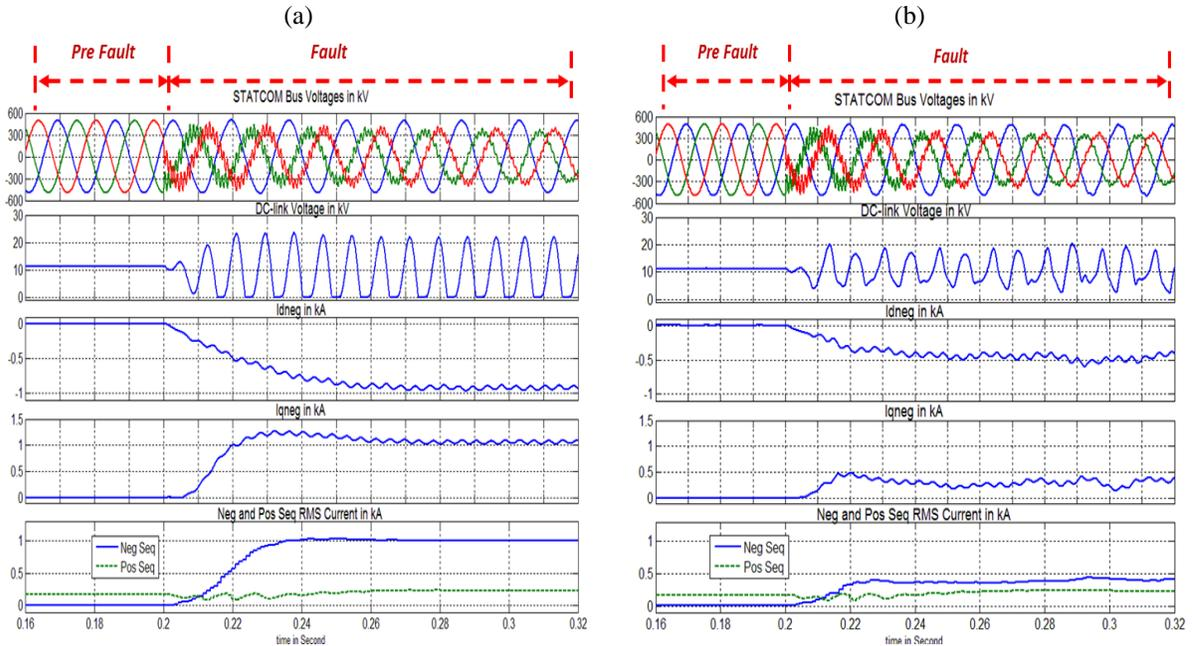
Figure 3-15. STATCOM performance with (b) and without (a) proposed DAC when STATCOM is working in inductive mode and SLG fault at phase C is applied right at STATCOM bus. (PSCAD/EMTDC simulation results)
