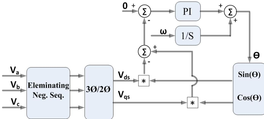
Figure 4-11. Block diagram of the Phase Locked Loop
