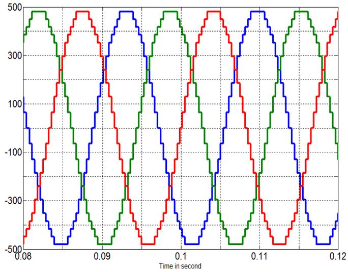
Figure 4-13. The 48-pulse output voltage when the DC-link is not connected to the single phase inverter.
