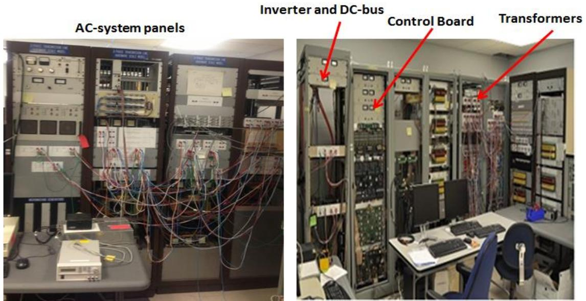
Figure 3-19. Control and magnetic panels
