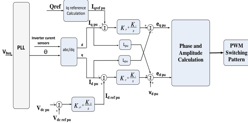
Figure 2-5. Vector controlled STATCOM control structure
