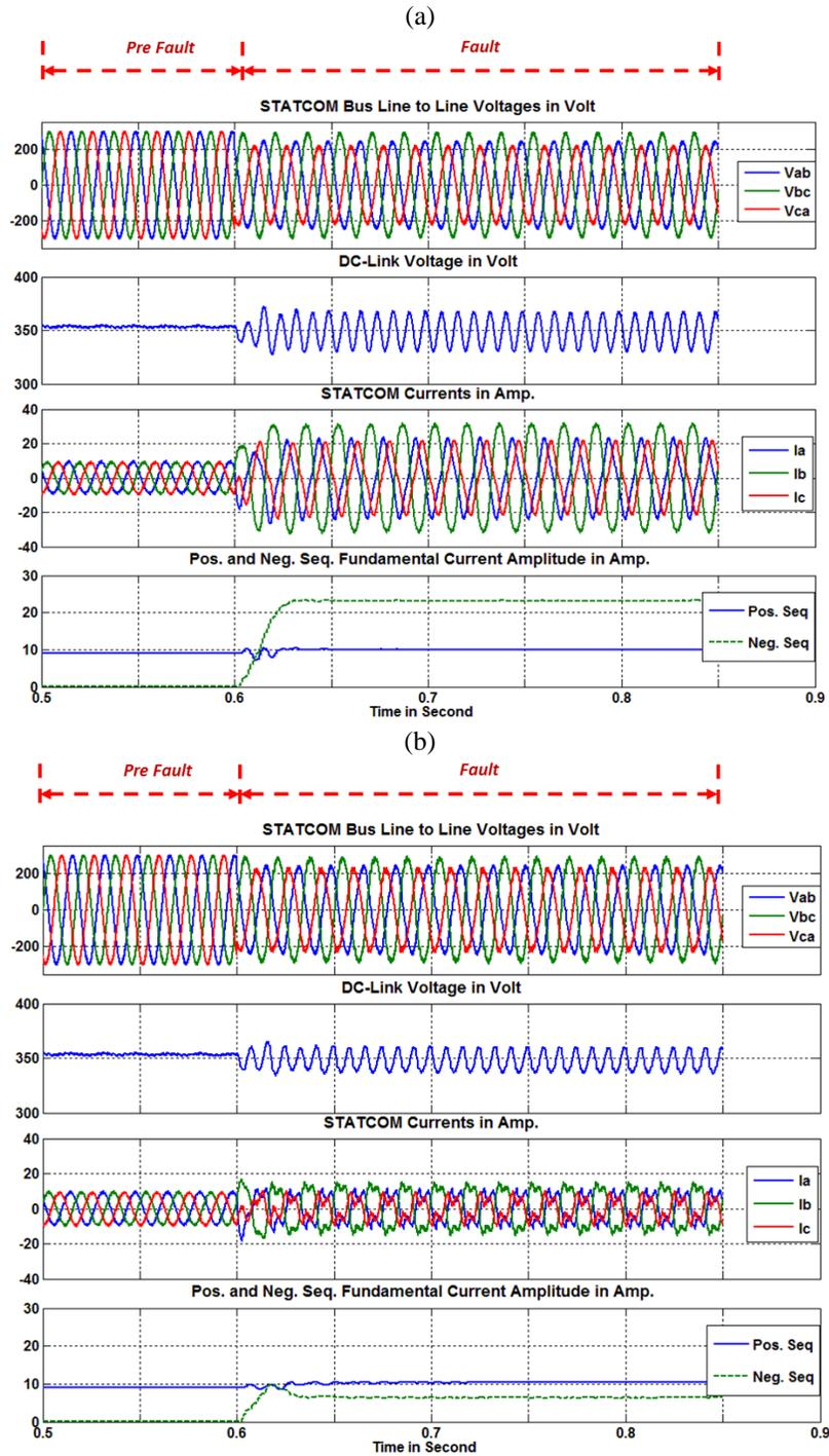
Figure 5-17. STATCOM performance with (b) and without (a) proposed controller when STATCOM is working in capacitive mode
