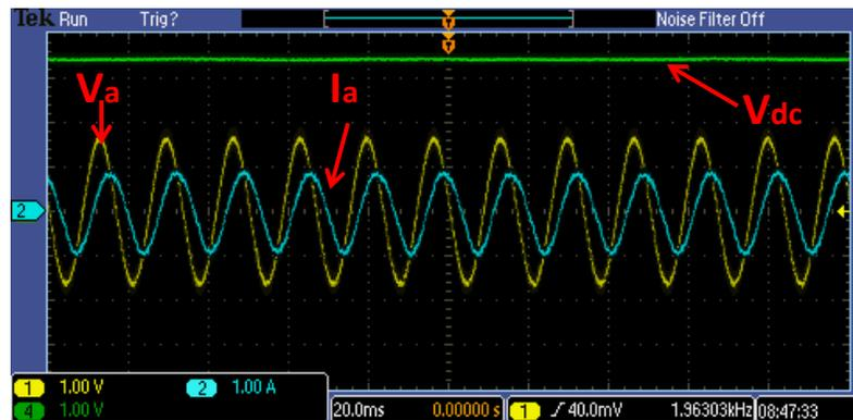
Figure 6-9. Rectifier voltages and current under normal condition. Voltage scale: 100V/div. and Current scale: 10A/div.
