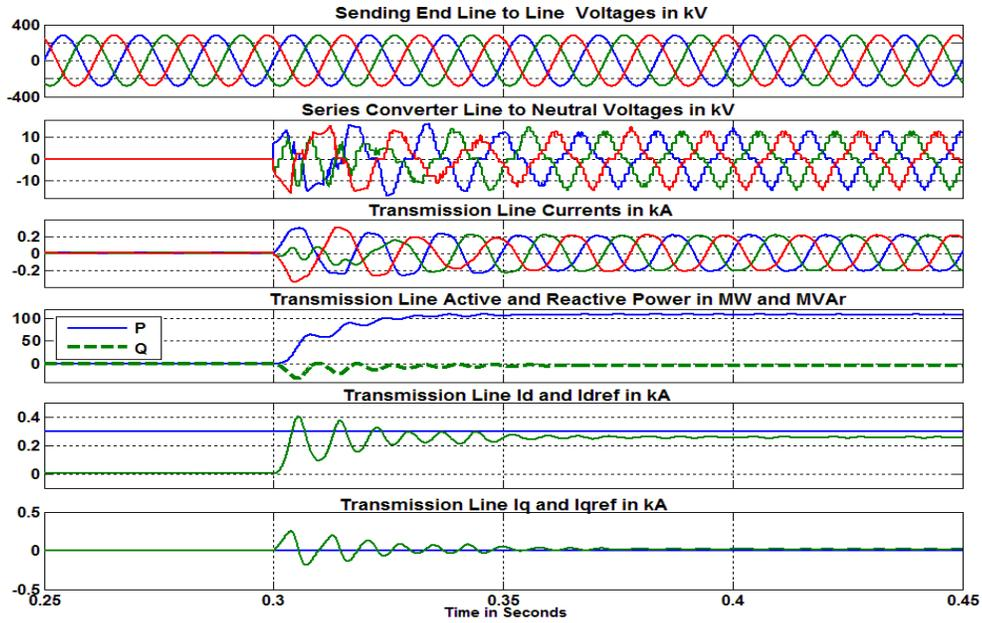
Figure 7-13. UPFC performance with a step change in the  $i_{d\text{ref}}$  (active power reference). UPFC works in power flow controller mode with series inverter in cross-coupling method
