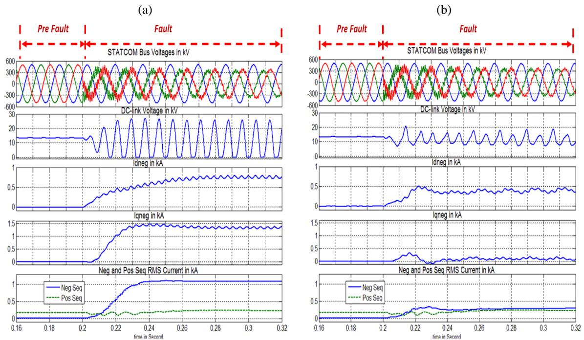
Figure 3-14. STATCOM performance with (b) and without (a) proposed DAC when STATCOM is working in capacitive mode and SLG fault at phase C is applied right at STATCOM bus. (PSCAD/EMTDC simulation results)
