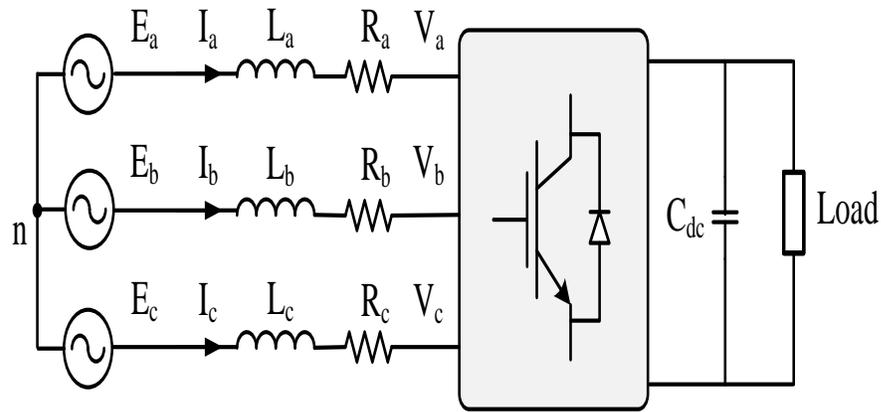
Figure 6-1. VSC connected to the grid
