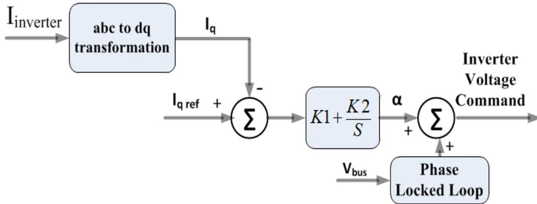
Figure 7-6. Angle-controlled STATCOM control structure
