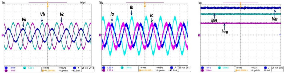
Figure 5-20. Capacitive mode performance of the STATCOM under SLG fault without proposed controller. Voltage scale: 100V/div. and Current scale:5A/div.
