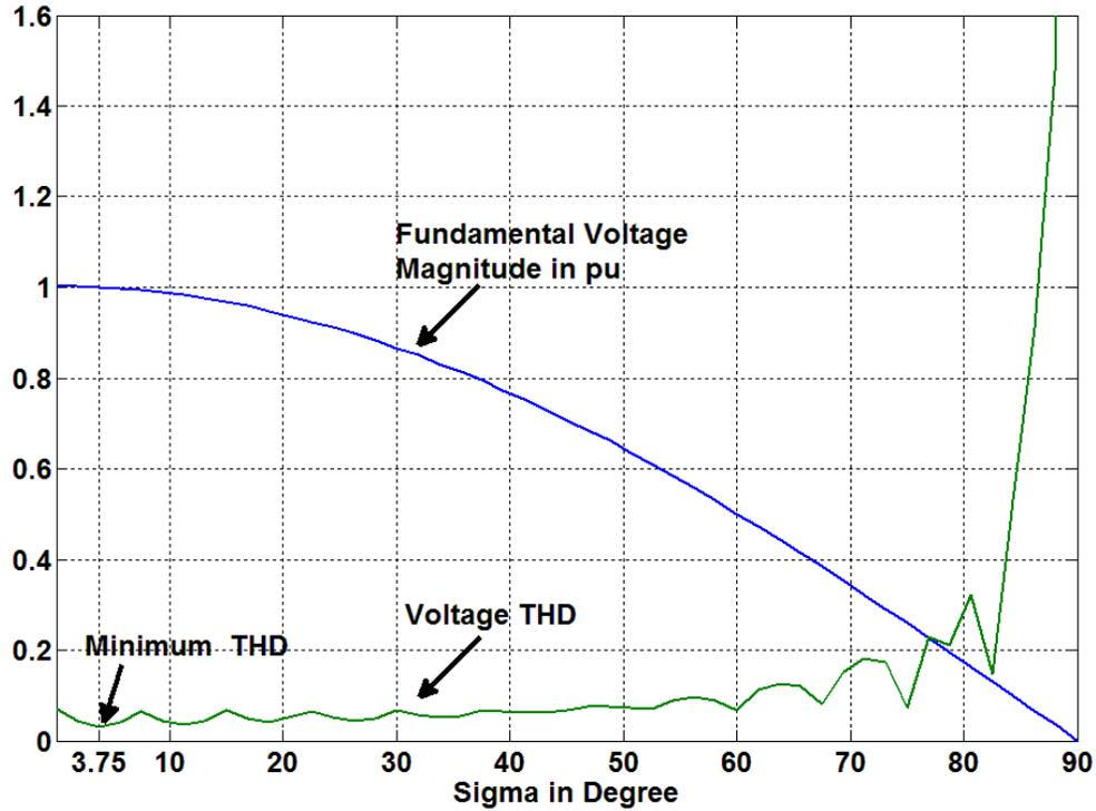
Figure 7-19. Fundamental voltage amplitude and the output voltage THD of the simulation system 48-pulse inverter when  $\sigma$  increases from zero to  $90^\circ$ . Per unit values are based on 345kV, and 100 MVA
