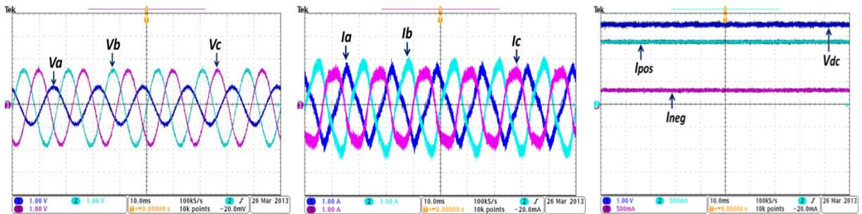
Figure 5-21. Capacitive mode performance of STATCOM under SLG fault with proposed controller. Voltage scale: 100V/div. and Current scale:5A/div.
