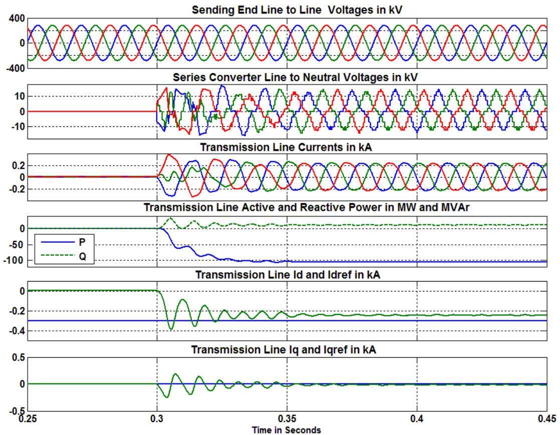
Figure 7-15. UPFC performance with a step change in the  $i_{d\ ref}$  (active power reference). UPFC series inverter is controlled with cross-coupling method.
