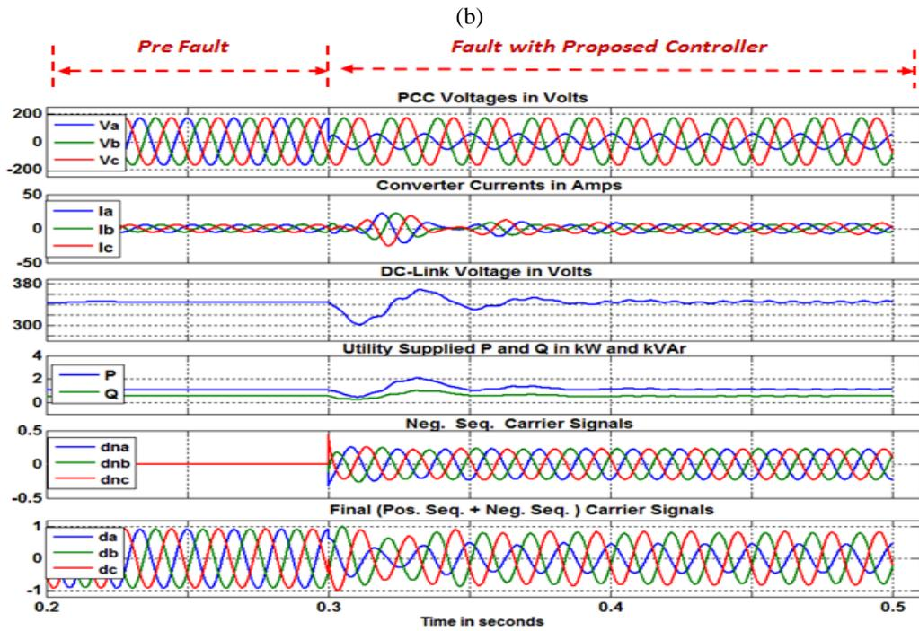
Figure 6-6. Converter performance with (b) and without (a) proposed controller under SLG fault at phase A right at PCC
