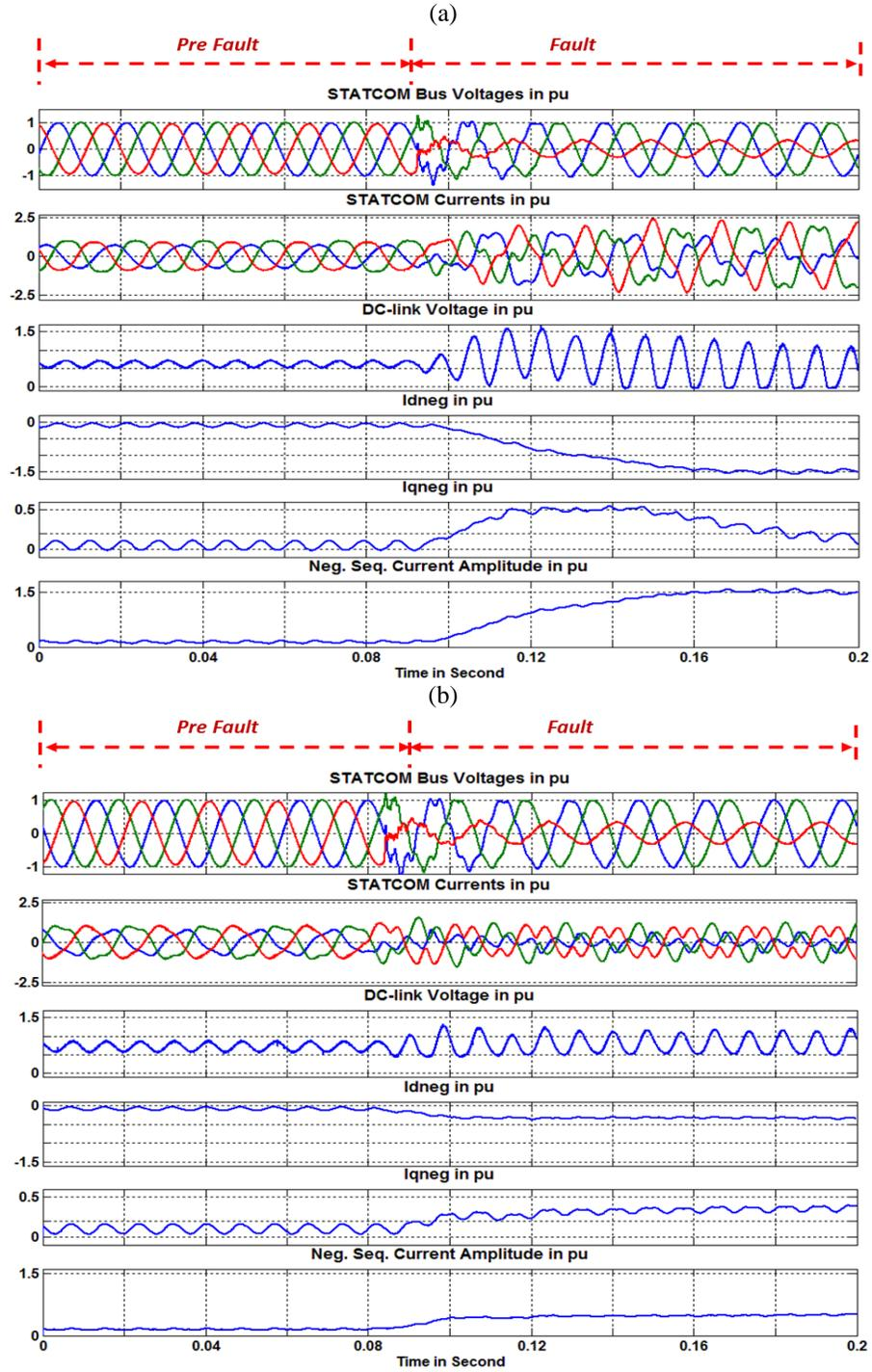
Figure 3-24. Inductive mode performance of STATCOM under single line to ground fault with (b) and without (a) DAC. All pu values are based on 12 VA and 100 V RMS (L-L) ac system. (Experimental results)
