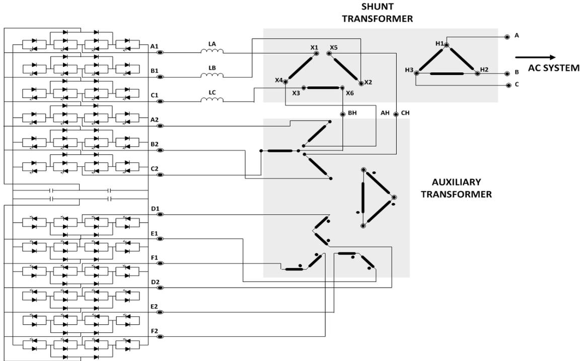
Figure 4-12. Power circuit of the NYPA three-level NPC 48-pulse inverter
