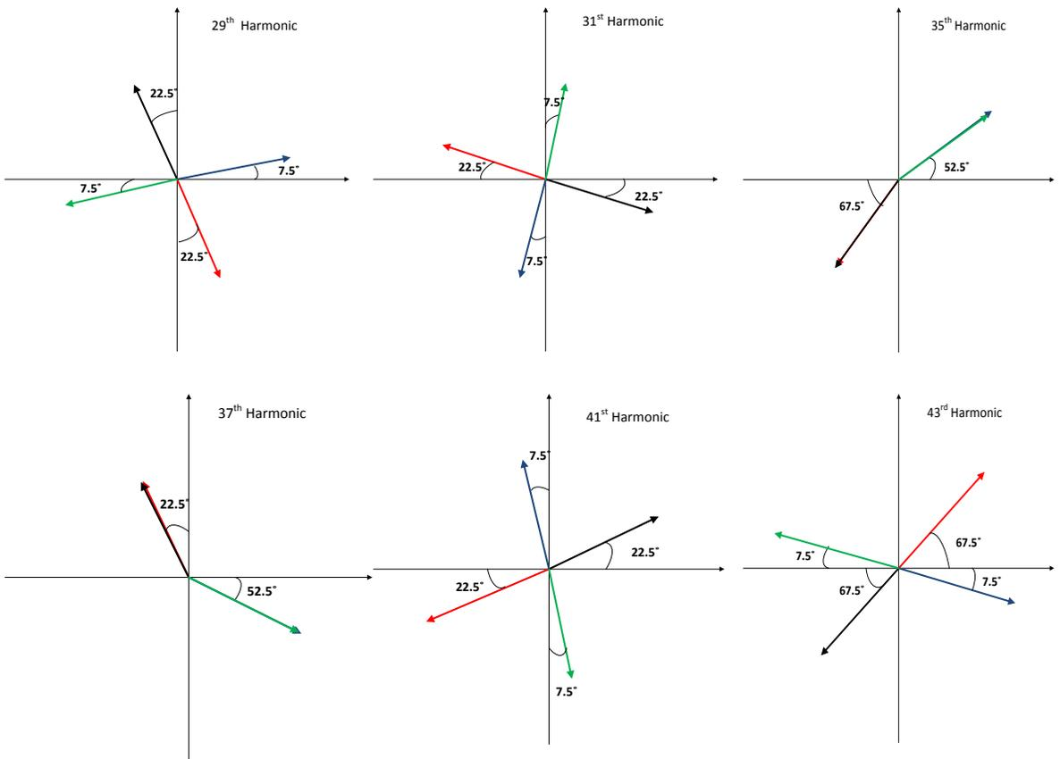
Figure 2-32. illustrative harmonic elimination of the 48-pulse inverter using the gate drive phase shift and also auxiliary and shunt transformers phase shifting. All the harmonics up to the 49<sup>th</sup> are illustrated. Blue, red, green, and black represent the NPC converter 1, 2, 3, and 4 respectively.
