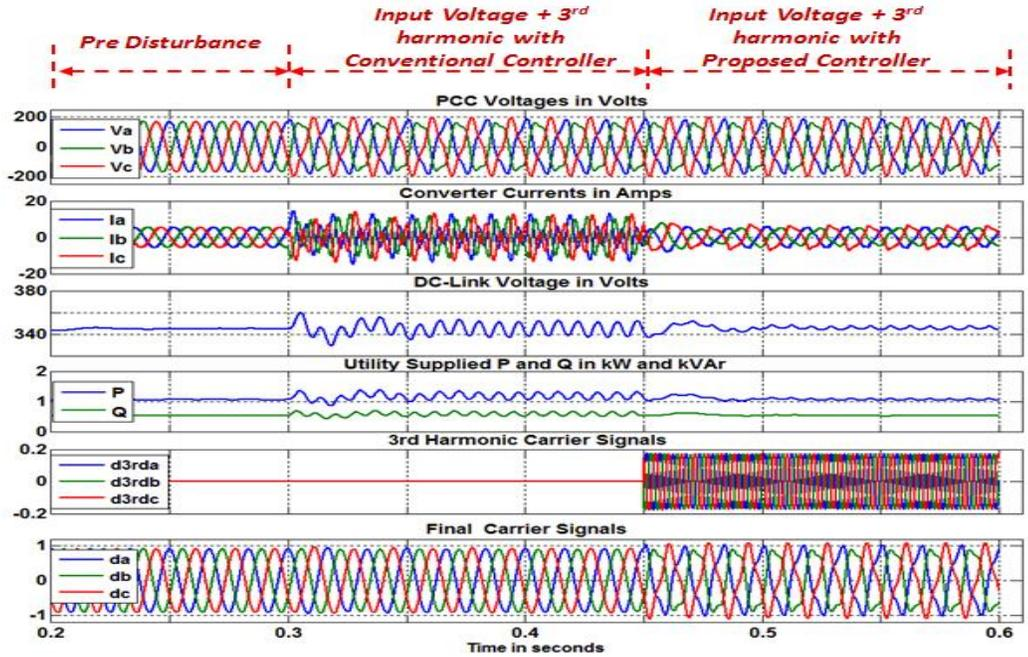
Figure 6-5. Converter performance with and without proposed controller when there is negative (a)/3rd harmonic (b) voltage injection as big as 20% of the nominal system voltage in series with grid AC sources
