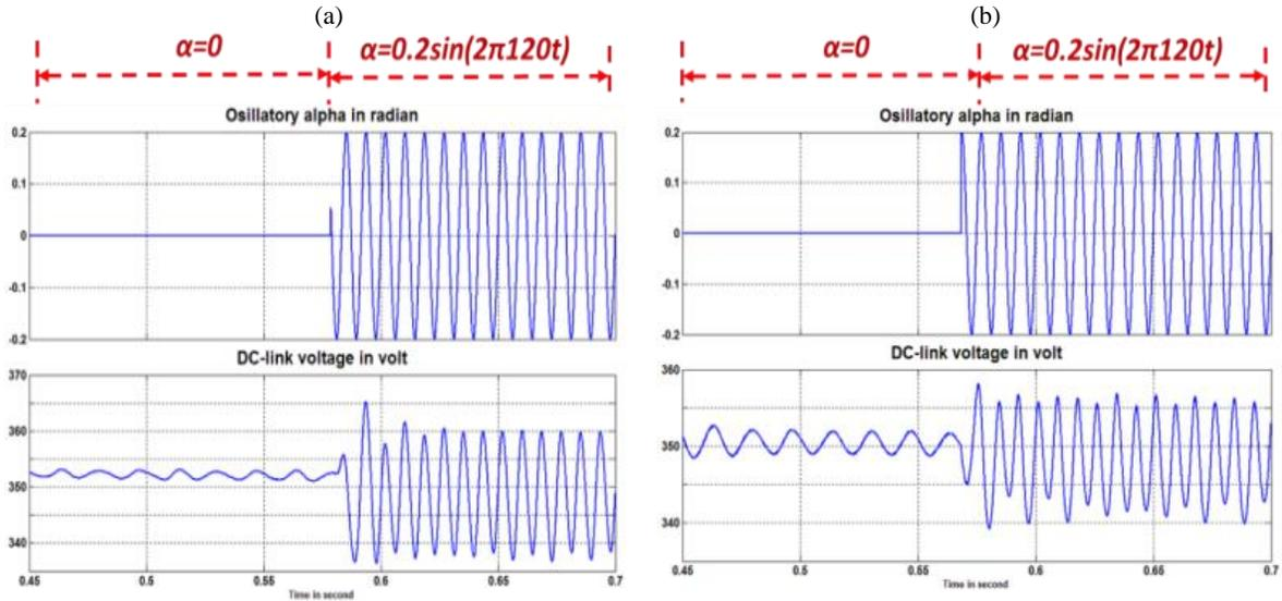
Figure 5-12. DC-link voltage 2nd harmonic oscillations generated by introducing 2nd harmonic oscillations to  $\alpha$  in both capacitive (a) and inductive (b) operation modes.
