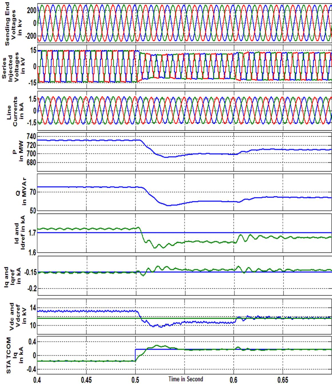
Figure 7-25. UPFC performance when the shunt inverter operating point changes from fully capacitive to fully inductive with and without proposed solution. The desired DC-link voltage is set to 11.5kV ( $\sigma_{cal} = 22.4^\circ$ ).
