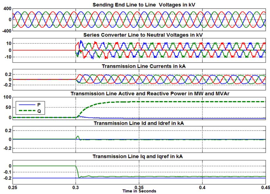
Figure 7-18. UPFC performance with a step change in the  $i_{q \text{ ref}}$  (reactive power reference) when the series inverter is controlled with advanced control method.
