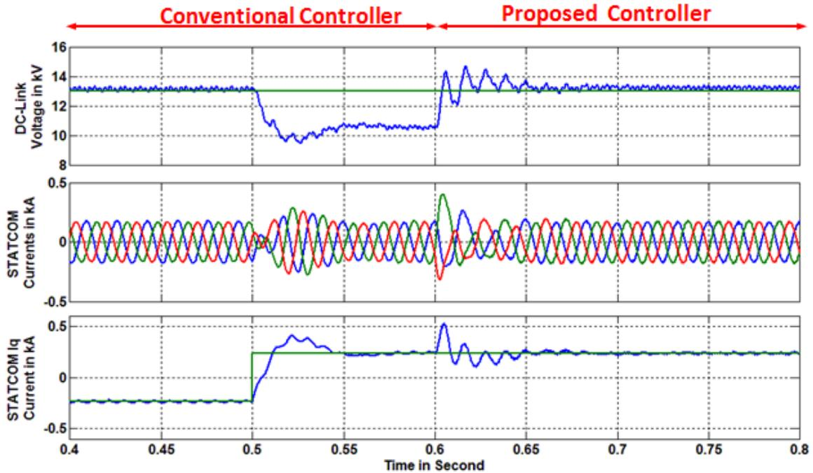
Figure 7-27. UPFC shunt inverter performance when the shunt inverter operating point changes form fully capacitive to fully inductive with and without proposed solution.
