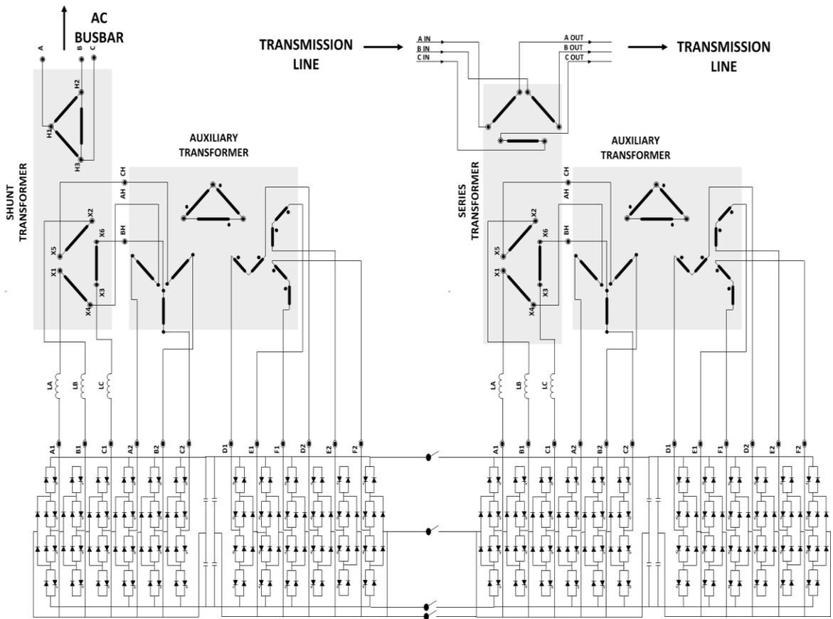
Figure 7-8. Power circuit of the UPFC used in the simulation verification. This UPFC model is developed based on the NYPA UPFC at Marcy substation[30]
