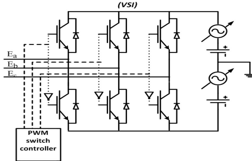
Figure 5-4. 2- level inverter with variable AC-sources used to calculate the generated negative sequence voltage at VSC terminals
