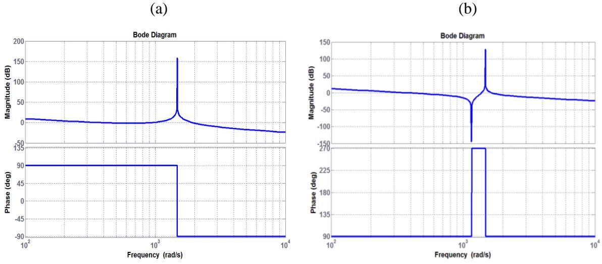
Figure 3-10. Bode plots of the DC-link voltage perturbation against  $\alpha$  perturbation around a capacitive (a)/inductive (b) equilibrium point
