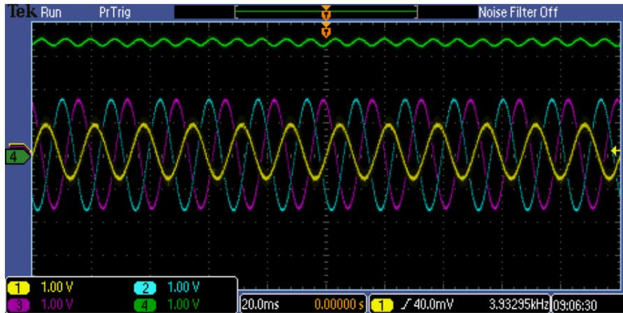
Figure 6-10. PCC and DC-link voltages under SLG fault at phase A when converter works with conventional controller. Chanel 1, 2, 3, and 4 indicate the  $V_a$ ,  $V_b$ ,  $V_c$ , and DC-link voltage respectively. Voltage scale: 100V/div.
