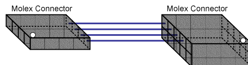
Figure 8.16 RS232 serial cable layout
