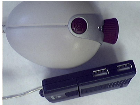
Figure 4.1 Compact USB hub shown beside the EvBot's USB camera for size comparison.
