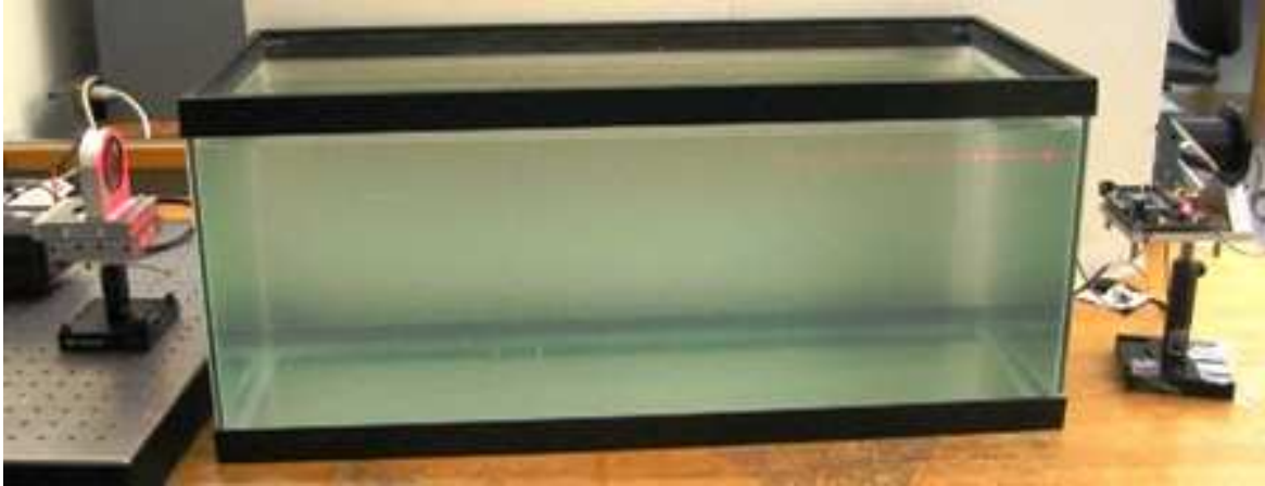
Figure 5.9 Underwater experiment tank filled with 5mL of Maalox® liquid (side view)
