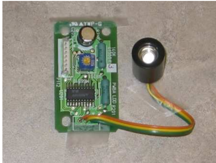
Figure 4.3 Laser driver board with laser diode attached to it
