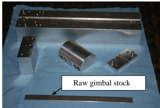
Fig. 15. Initial gimbal fabrication fixture components
