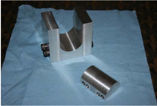
Fig. 2. Final gimbal forming fixture
