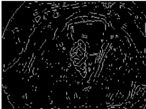
Fig. 6. LaPlacian of Gaussian Edge Detection results - simple case
