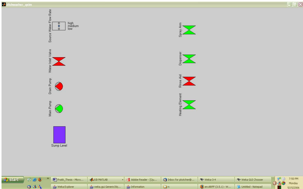
Figure 9 Display showing qualitative status of different components of the dishwasher
