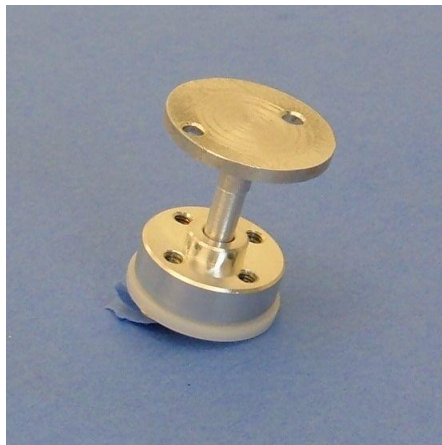
Figure 22 - EndoWrist Attachment and Aluminum Hub Mount
