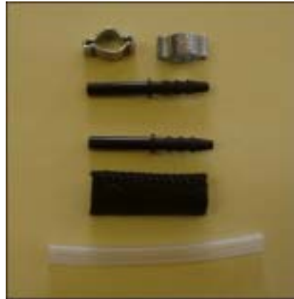
Figure 3.12 Materials required for new air muscle design
