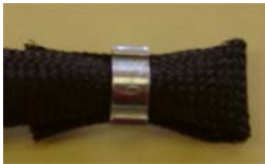
Figure 3.13 Loop formed on plugged end of air muscle
