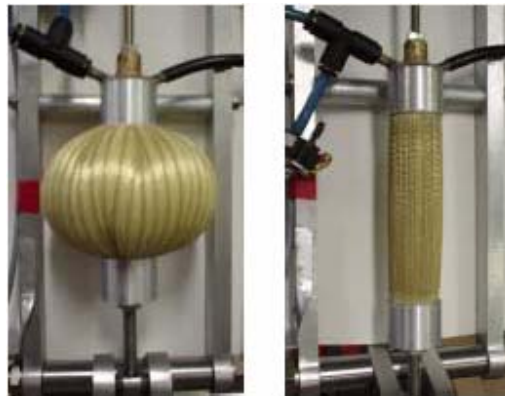
Figure 2.11 Pleated Air Muscle and its ‘pumpkin’ shape
