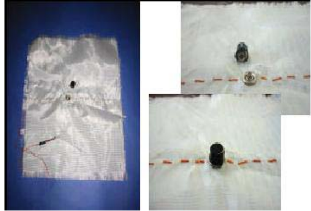
Figure 3.6 Coaxial snap connector for microphone attachment.
