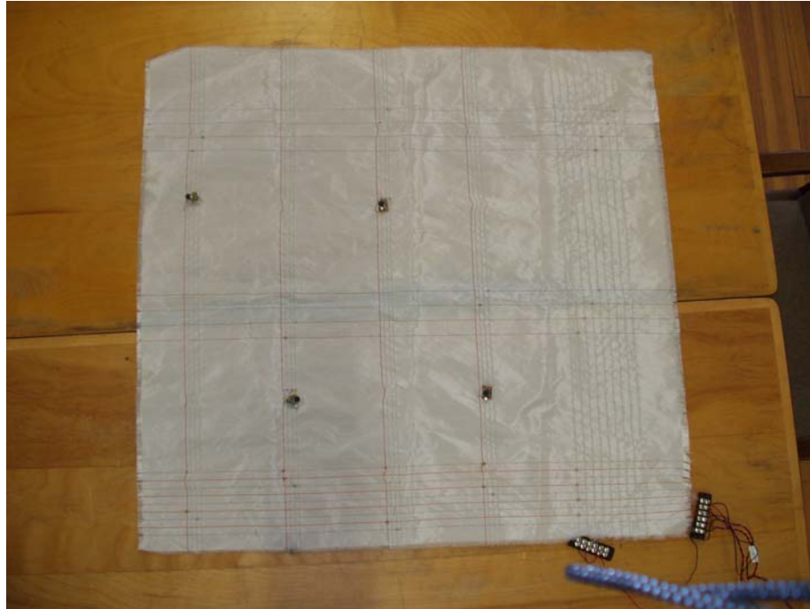
Figure 3.4 Textile array containing both microphones and amplifiers on fabric.
