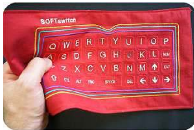
Figure 2.1 A Flexible PDA keyboard utilizing SOFTSwitch technology [10].
