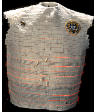
Figure 2.3 Georgia Tech's Smart Shirt is used to monitor the wearer's vital signs.
