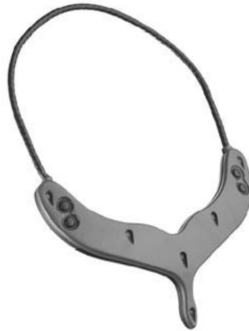
Figure 2.5 Acoustic array necklace for the hearing impaired.
