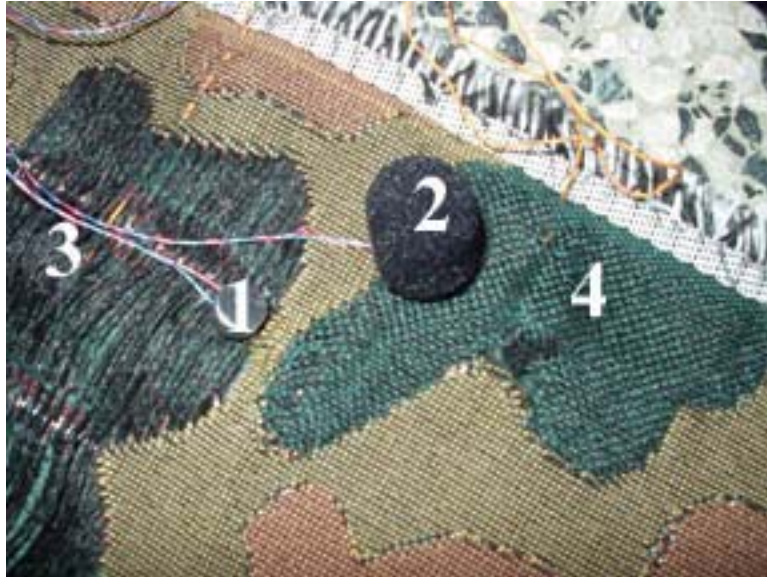
Figure 3.2 Camouflage array with woven windscreens. 1 is an unprotected mic, 2 has a lavalier windscreen, 3 is a loosely woven windscreen, and 4 is a tight woven windscreen.
