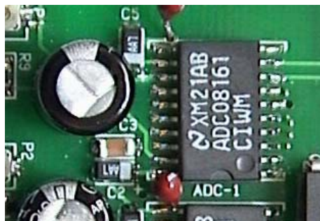
Figure 5.6: Analog-to-digital converter on a section of the USB-DAQ8 board.
