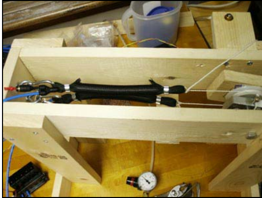
Figure 4.5 Antagonistic muscle pair controlling the wooden arm
