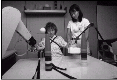
Figure 2.4 MIME uses a PUMA 560 for the patient's impaired limb.
