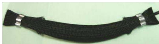
Figure 3.5 New Air Muscle Design
