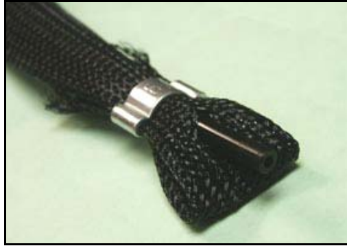
Figure 3.7 Open tube end of air muscle pushing through braiding
