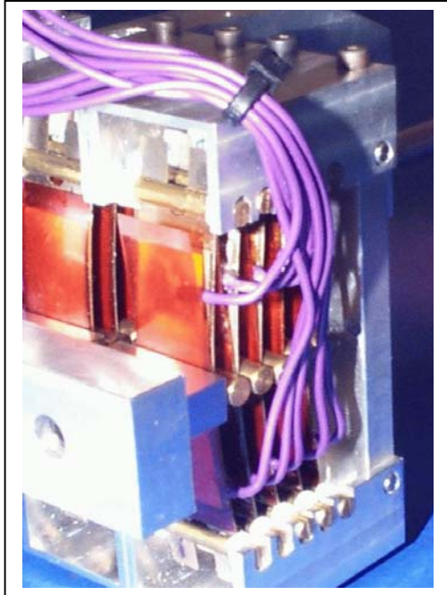
Figure 7.1.1—3. (color) Close-up of parallel arrangement in each actuator box, showing end axles and center pivots (Photograph by graduate student, N.C. State University Center for Robotics and Intelligent Machines)
