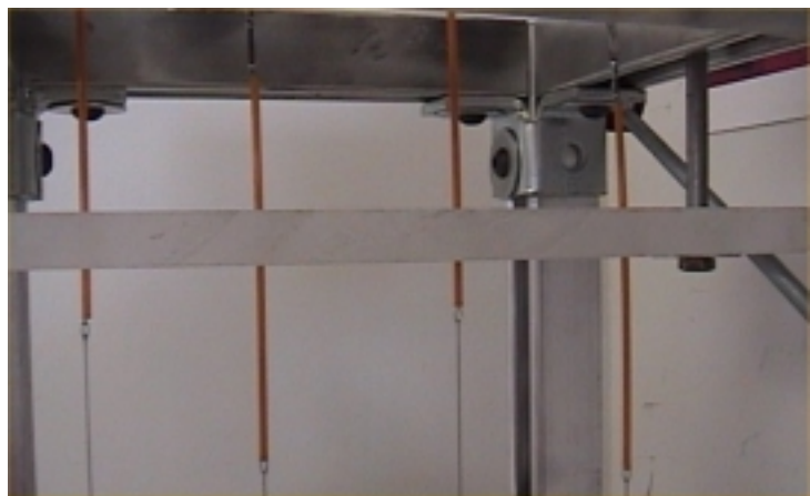
Figure 3.15 Plexiglas guide for harness path.
