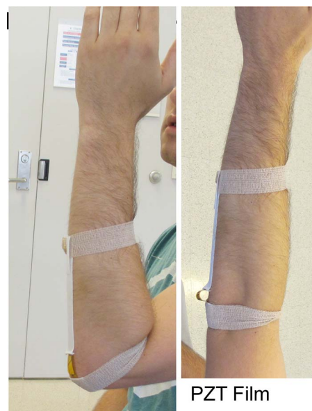
Fig. 7. Piezoelectric-coated film on a Ni foil, bent around an elbow.
