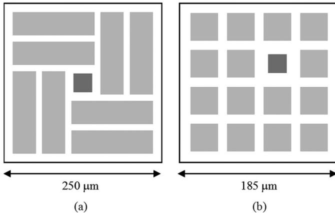
Fig. 3. CMUT cell layouts for (a) design 1 and (b) design 2. The light shade denotes membranes; the dark shade denotes contact vias.
