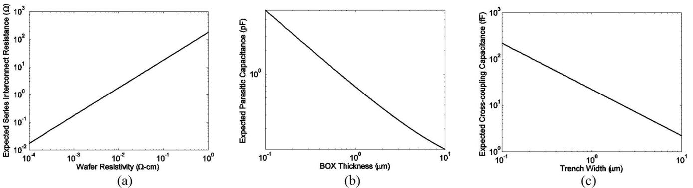
Fig. 2. (a) Expected series resistance, (b) expected parasitic capacitance, and (c) expected cross-coupling capacitance.
