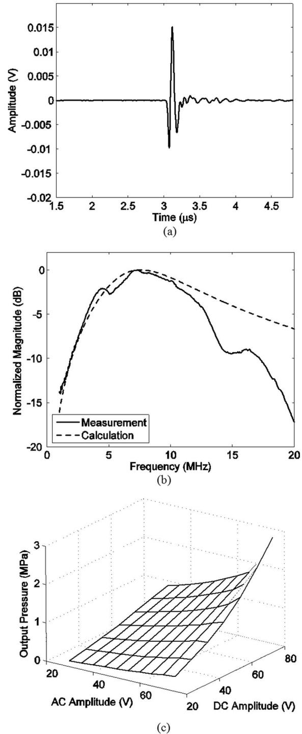
Fig. 8. (a) Waveform received by the hydrophone, (b) spectrum of the hydrophone reading, and (c) output pressure at the surface of the transducer for various DC bias and AC excitation voltages.
