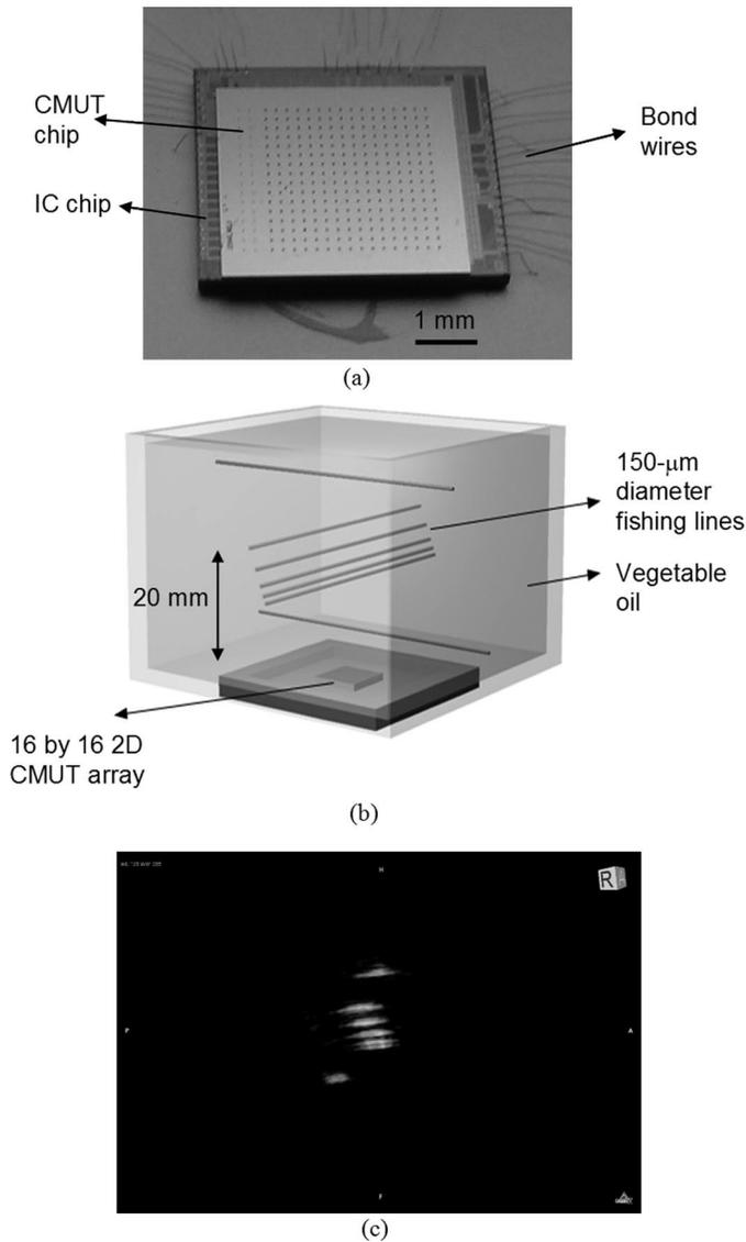
Fig. 9. (a) Photograph of 2-D array chip-to-chip bonded to an IC, (b) diagram of the wire phantom setup for the 3-D imaging experiment, and (c) 3-D ultrasound image of the wire phantom.
