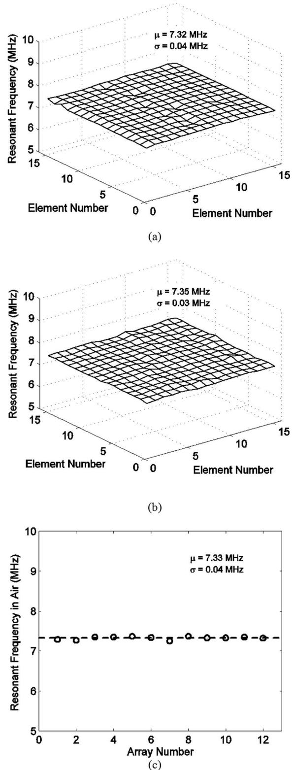
Fig. 6. Resonant frequency distribution across a  $16 \times 16$ -element 2-D array: (a) before chip-to-chip bonding, (b) after chip-to-chip bonding, and (c) across 12 arrays.
