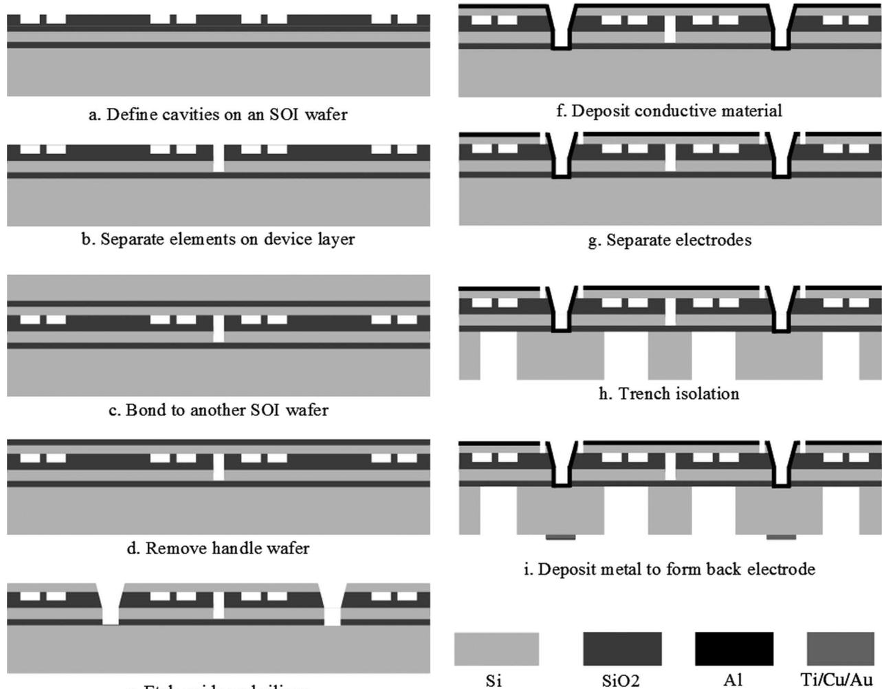
Fig. 4. Illustration of the fabrication process.
