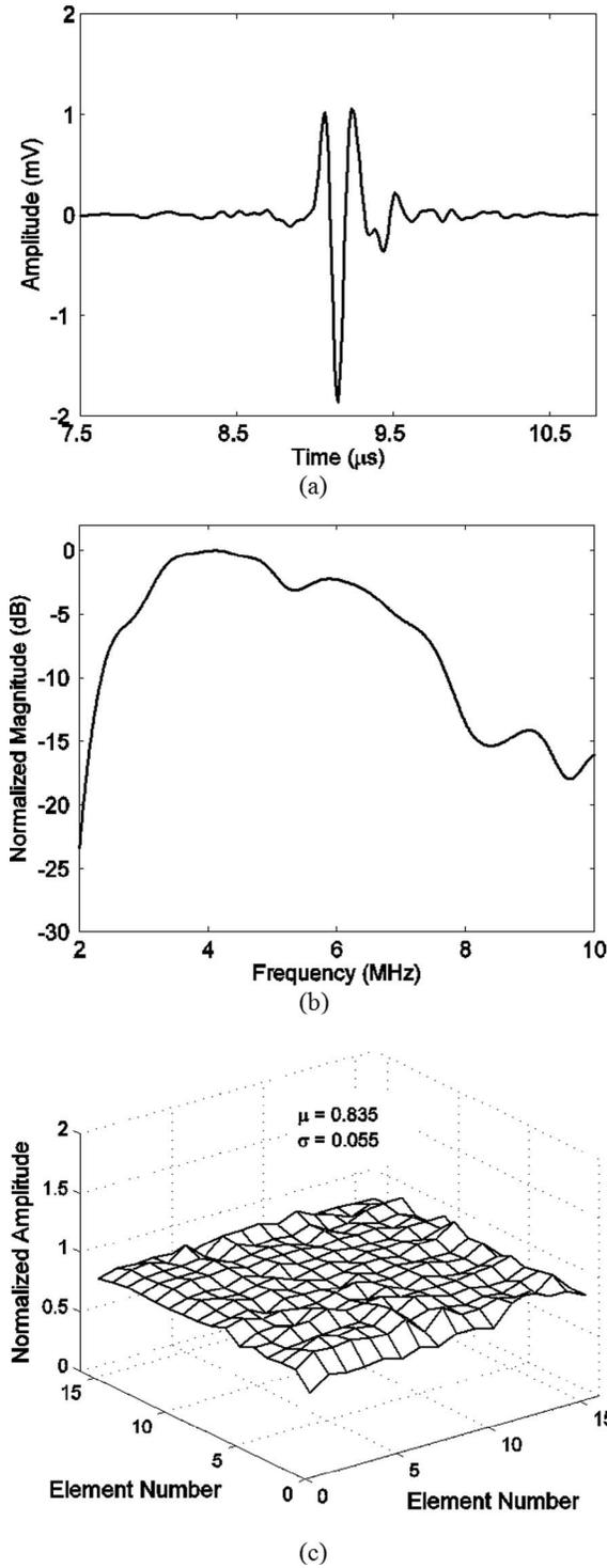
Fig. 7. (a) Received pulse-echo waveform, (b) pulse-echo spectrum, and (c) pulse-echo amplitude distribution across the array.
