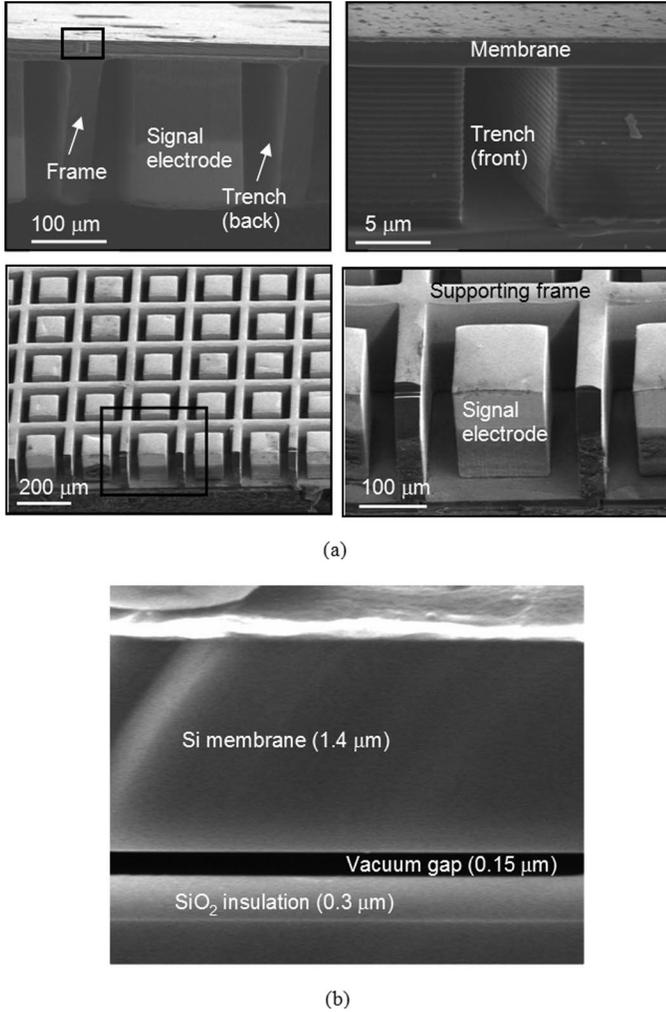
Fig. 5. (a) SEM pictures show the trench and frame structures. (b) Good control over the membrane thickness as well as vacuum gap height is achieved.
