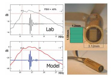
**Figure 2.** The second-generation 14.4-MHz ML piezoceramic 9F subassembly is shown (right) with measured (top left) and estimated (bottom left) pulse echo performance. Fifty percent FBW was achieved. The array aperture of only  $1.2 \times 1.58$  mm is shown (top right) with the element layout as indicated.
