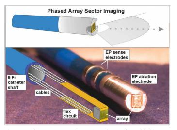
**Figure 1.** The 14-MHz, 24-element phased array forward-looking ML catheter tip region is shown. A completely equipped mechanical prototype is shown with its internal structures, including the PZT array, flex circuit, and cabling (bottom left).
