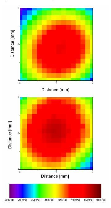
Figure 2. Mechanically scanned calibrated image (Top). Electrically scanned CMUT hydrophone image (Bottom)
