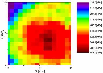
Figure 5. Spot Shower measured at 5 W of input power.
