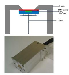
Figure 1. Diagram and picture of hydrophone package.
