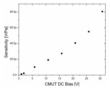
Figure 4. CMUT sensitivity as a function of DC bias.
