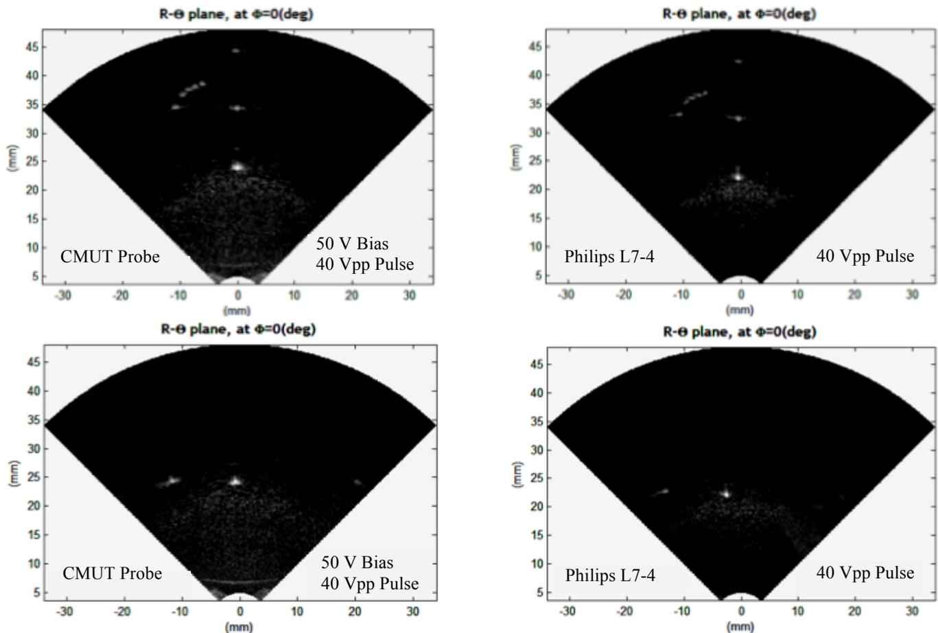
Figure 6. Images of nylon wires (Gammex 406LE) acquired by the CMUT probe (left) & a commercially available probe (right). Dynamic range: 40 dB.
