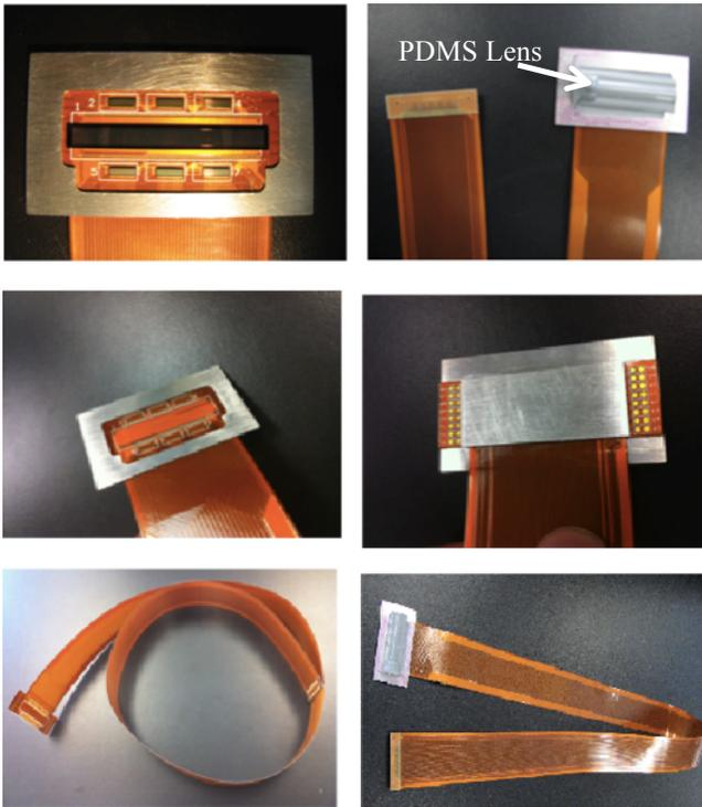
Figure 4. Assembly photos of CMUT probe
