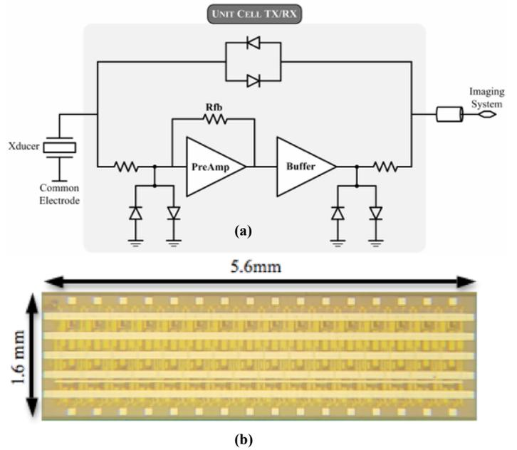
Figure 3. (a) Block diagram of a single channel, (b) Die photo of a single IC (16 channels)
