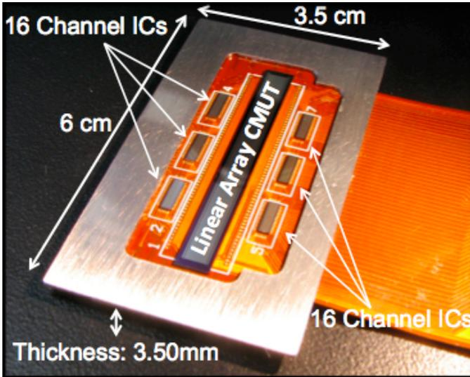
Figure 2. Integration of CMUT and ICs on flexible PCB
