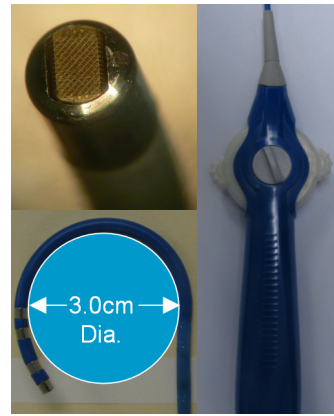
Figure 2. The microlinear (ML) general design format as a 9F (3 mm) catheter with a 24 element 14 MHz phased array at the tip. The steerability and multiple electrodes permit good endocardial positioning and operation with the electroanatomical mapping system used.
