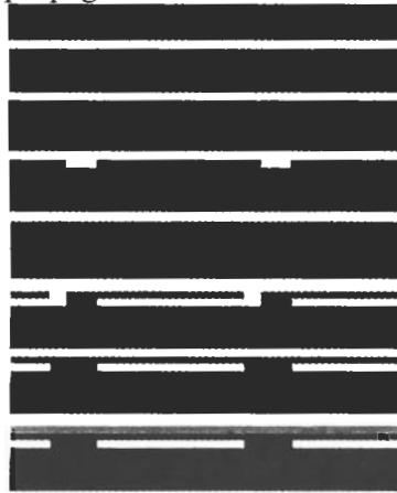
Fig. 3. Schematic of the processing schedule for fabricating cMUTs.
