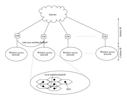
Fig. 2. Cellular IP architecture.
