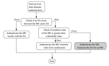
Fig. 7. Overview of local authentication control scheme.
