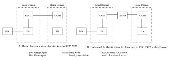
Fig. 6. Basic and enhanced authentication architecture in Mobile IP.
