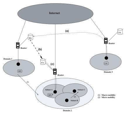
Fig. 1. Mobile IP architecture.
