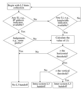
Fig. 5. Layer 3 movement estimation process.
