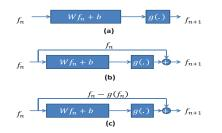
**Fig. 1**. Schematic scheme of a single layer in a)ANN b)ResNet and c)modified ResNet Architectures.
